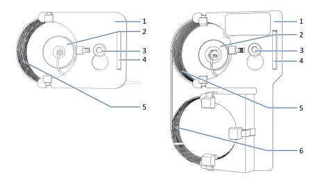
Figure 65: Components of the sample loop unit (left: 10/25/100  $\mu$ L, right: 250/1000  $\mu$ L)
