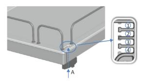
Figure 31: Guide hole and tubing guides in the solvent rack
