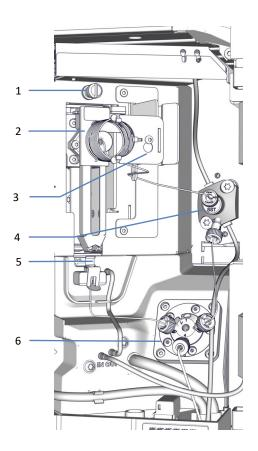
Figure 5: Injection unit in the VC-Single split sampler (without insulation loop cover)
