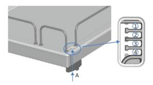
Figure 27: Guide hole and tubing guides in the solvent rack
