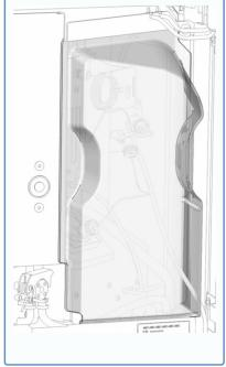
Figure 37: Left: Installing the protective cover behind the leak tray Right: Protective cover installed
