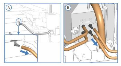
Figure 96: Disconnecting the wash line to the needle wash reservoir (A: VF-/VH-single split sampler, B: dual split sampler)
