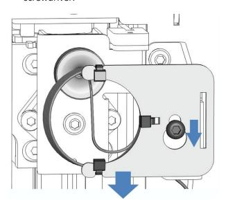
Figure 67: Aligning the sample loop unit to the screw
