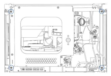
Figure 97: Captive screws on the slide-in module
