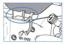
Figure 41: Loop cover notches
