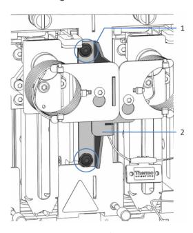
Figure 90: Carrier plate for the sample loops in the dual split sampler
