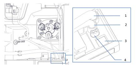
Figure 23: Drain ports in the leak tray of the VC single split sampler
