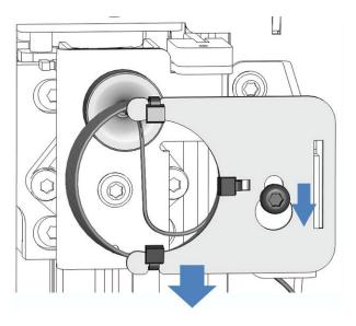
Figure 73: Aligning the left sample loop unit to the screw
