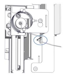
Figure 68: VC-autosampler capillary from the sample loop to the metering device head
