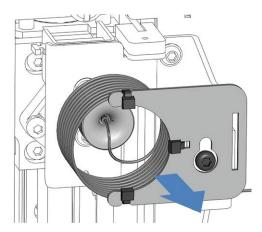
Figure 71: Removing the sample loop unit (here: left sample loop)
