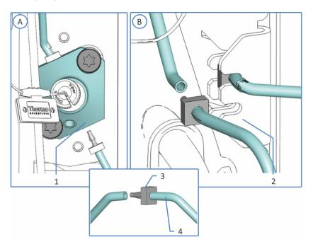
Figure 64: Seal wash outlet line connection
