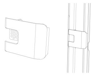
Figure 20: Tubing bracket (left), tubing bracket installed (right)
