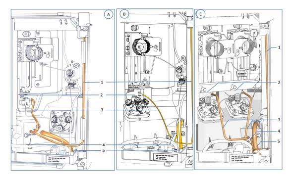
Figure 29: Needle wash components
