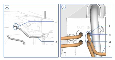
Figure 30: Needle wash inlet connections (shown here: VF- and VH-autosampler)
