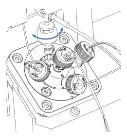
Figure 75: Needle seat VF/VH-autosampler
