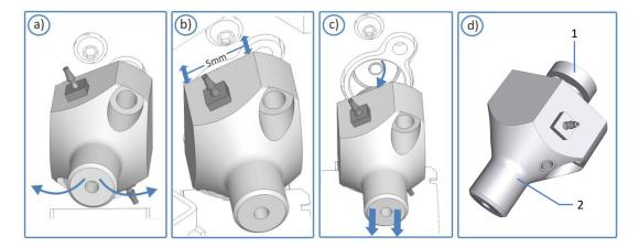
Figure 80: Detaching the metering device head
