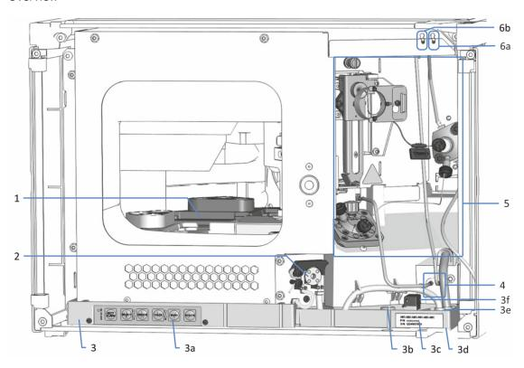
Figure 6: VH-A10 / VF-A10 Single split sampler interior view
