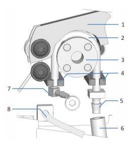
Figure 88: Tubes disconnected from the drain pump, example view from VF-/VH-autosampler.
