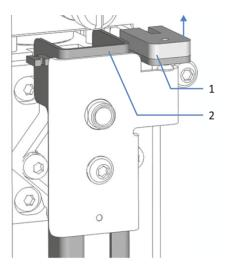
Figure 78: Moving lock for vial pusher upward
