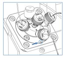
Figure 82: Drain hole on the injection valve (shown here VF-/VH-autosampler injection valve)
