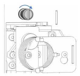
Figure 46: Tightening the shipping lock screw
