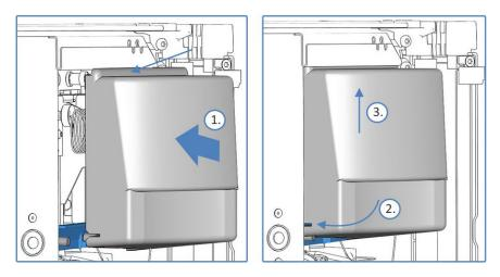
Figure 40: Insulation loop cover installation at the dual split sampler
