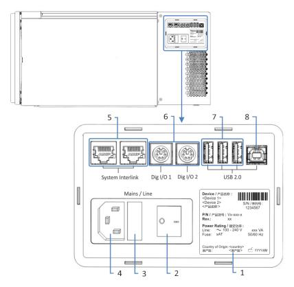
Figure 18: Electrical connectors on the right side of the autosampler
