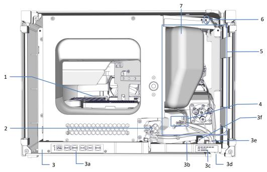
Figure 3: VC-A12 Single split sampler interior view
