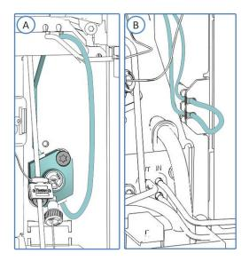
Figure 95: Closing the seal wash path in the autosampler (A: single split sampler, B: dual split sampler)
