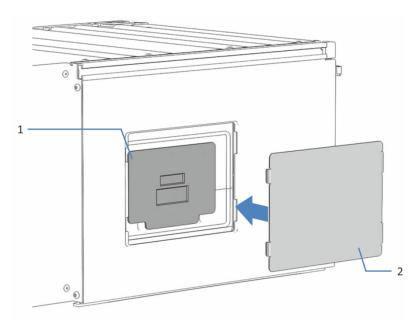
Figure 45: Closing the Charger opening (here with metal cover plate clamped in the opening)
