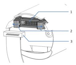
Figure 85: Connector and cable on the rear side of the injection valve drive
