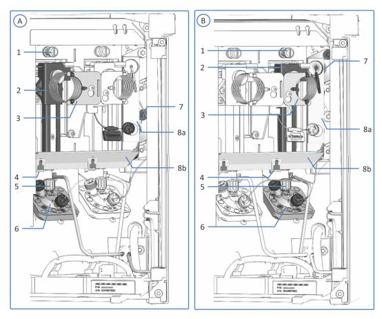
Figure 9: Injection units in the dual split sampler without insulation loop cover
