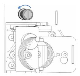
Figure 15: Loosening the shipping lock screw
