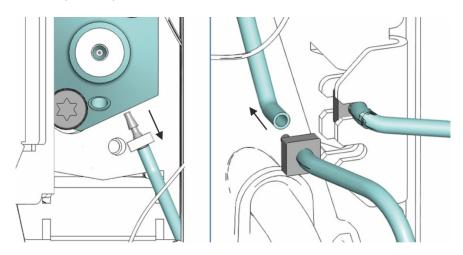
Figure 63: Interconnecting seal wash outlet line
