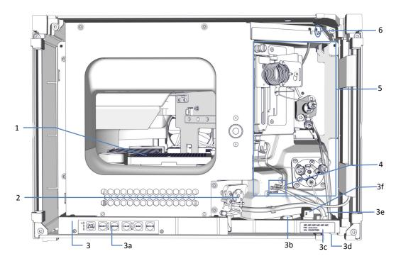
Figure 4: VC-A12 with removed loop cover / VC-A13 Single split sampler interior view
