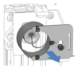
Figure 66: Removing the sample loop unit
