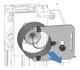
Figure 101: Removing the sample loop unit
