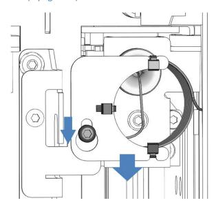
Figure 72: Aligning the right sample loop unit to the screw
