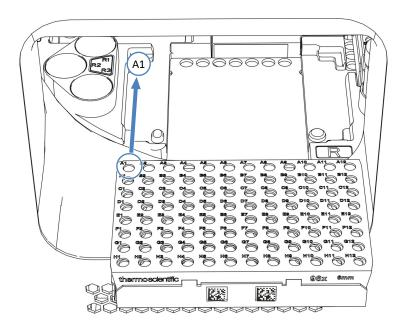
Figure 44: Correct orientation in carousel (here with a sample rack)
