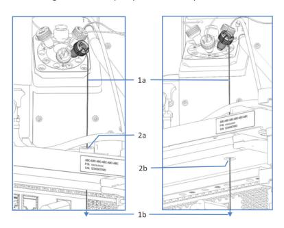
Figure 35: Guide holes in the autosampler and pump (left: view from VF-/VH-autosampler (example); right: view from pump)
