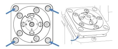
Figure 83: 4 Screws fixing the injection valve at the VF- and VH-autosampler (left); levering up the injection valve (right)
