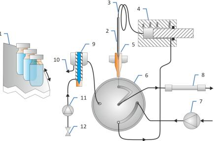
Figure 1: Operating principle VH- and VF-Autosampler
