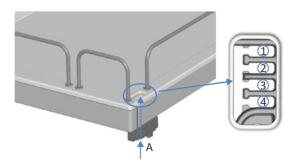
Figure 60: Guide hole and tubing guides in the solvent rack
