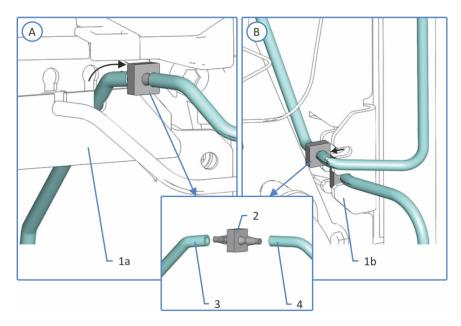
Figure 58: Seal wash reservoir line connection
