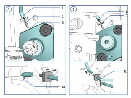
Figure 61: Seal wash inlet line connection
