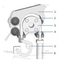
Figure 89: Drain pump
