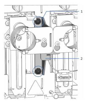
Figure 47: Carrier plate for the sample loops in the dual split sampler
