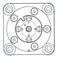
Figure 84: 4 Screws fixing the injection valve at the VC-autosampler
