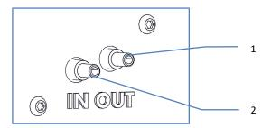
Figure 56: Needle wash outlet port connections in the VC-autosampler
