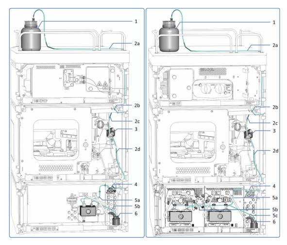
Figure 24: Seal wash system in the Vanquish system (examples with a VF/VH single split sampler, left: with quaternary pump, right: with binary pump)
