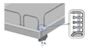
Figure 53: Guide hole and tubing guides in the solvent rack
