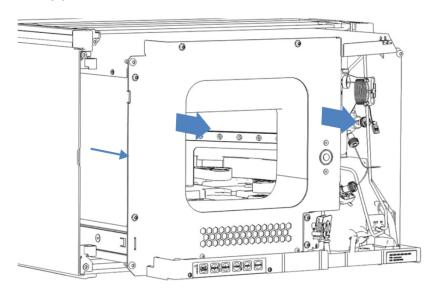
Figure 98: Pulling out the slide-in module
