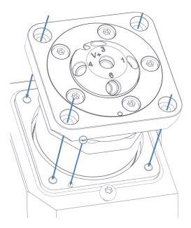
Figure 87: Aligning the injection valve (shown here: VF- and VH-autosampler)
