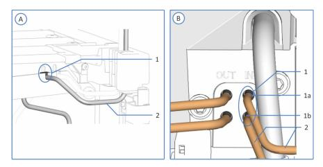
Figure 52: Needle wash inlet port connections
