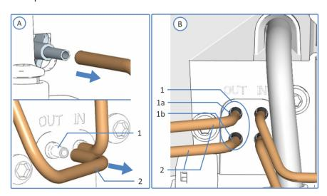
Figure 55: Needle wash outlet port connections in the VH/VF-autosampler
