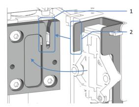
Figure 77: Installing the needle unit to the needle carriage
