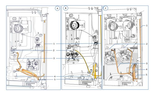
Figure 51: Needle wash components
