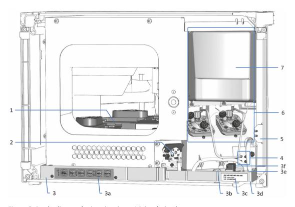
Figure 8: Dual split sampler interior view with insulation loop cover
