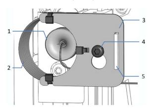
Figure 100: Sample loop unit installed to the needle unit
