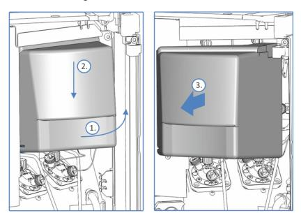
Figure 39: Insulation loop cover removal at dual split sampler
