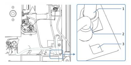
Figure 22: Drain ports in the leak tray of a VH/VF single split sampler
