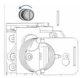
Figure 91: Loosening the shipping lock screw
