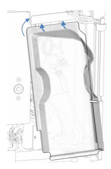
Figure 36: Sliding the protective cover under the top enclosure frame
