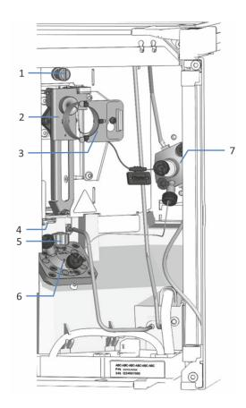
Figure 7: Injection unit in the single split sampler
