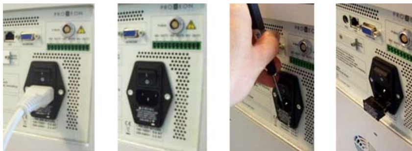
Figure 96. Replacing the main power fuse
