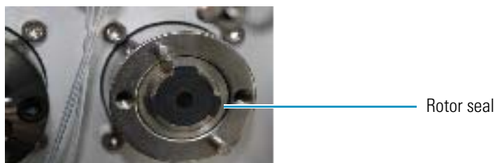
Figure 68. Rotor seal mounted on the valve driver
