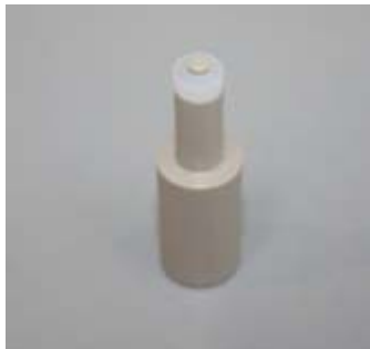
Figure 54. Piston seal mounted onto the piston seal tool (PLF model pump)
