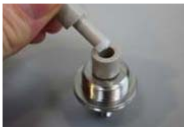
Figure 8. Inserting the piston seal tool into the guide
