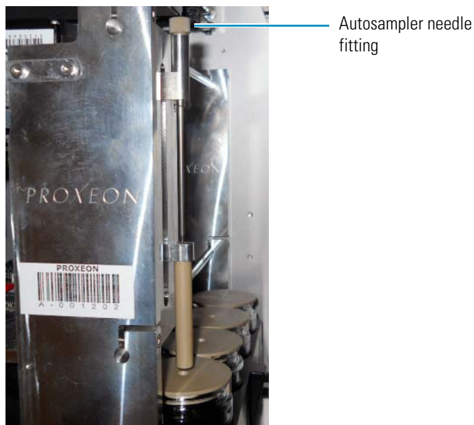
Figure 114. Needle connected to the needle holder
