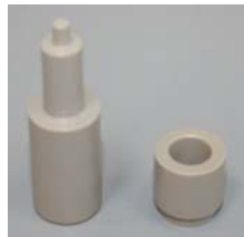
Figure 4. Two-component piston seal tool for the PLF model pump
