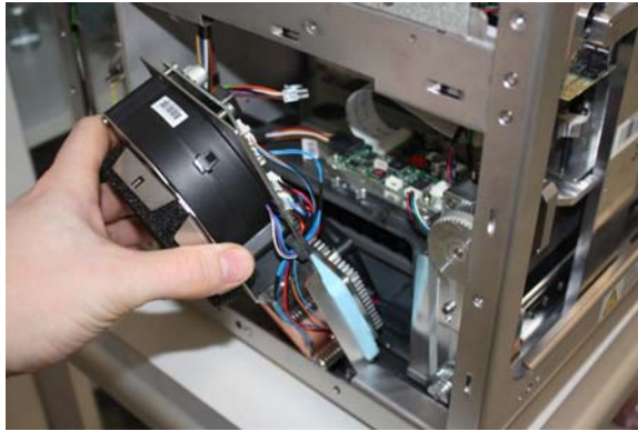
Figure 142. Pulling out the cooler
