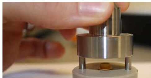
Figure 5. Inserting the piston seal into the pump head
