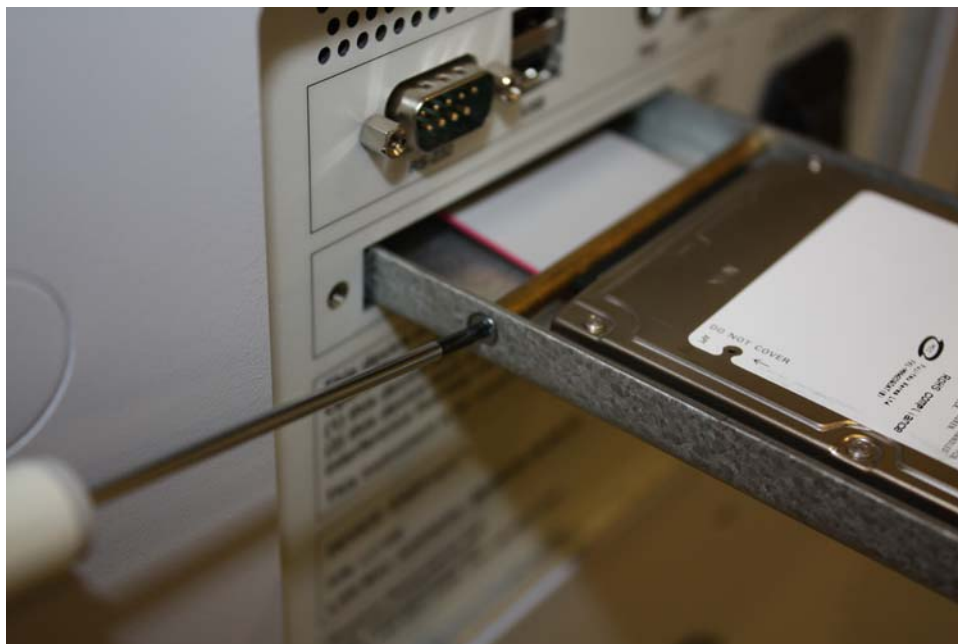
Figure 96. Removing the brass rod that holds the cable down
