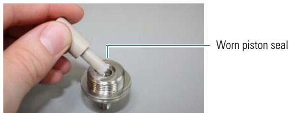
Figure 5. Using the piston seal tool to remove the worn piston seal
