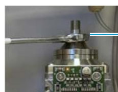
Figure 3. Removing the pump head
