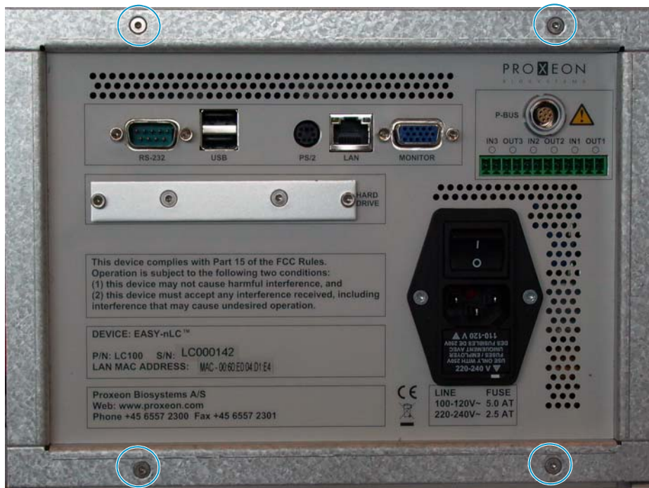
Figure 101. Screws to remove from the computer box
