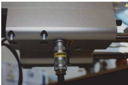
Figure 74. High-voltage cable connected to the ion source
