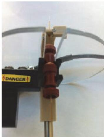
8. Connect the high voltage cable from the UHPLC liquid junction cross to the socket underneath the ion source (Figure 79).
