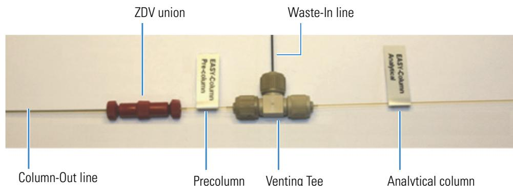
4. Connect the analytical column outlet to the transfer line going to the detector.
