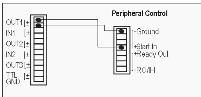
To make contact closure between the EASY-nLC instrument and the Orbitrap Fusion mass spectrometer, you must modify the Thermo Fisher contact closure cable by replacing one of the two-pin terminal blocks with the 8-pin terminal block provided in the MS Setup Kit.
