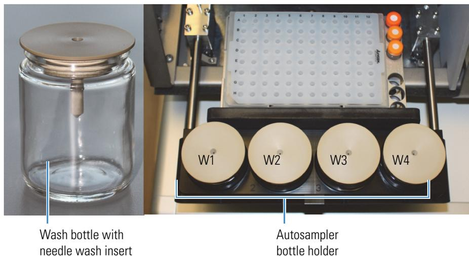
6. Put a wash bottle that contains solvent A into position W3.
