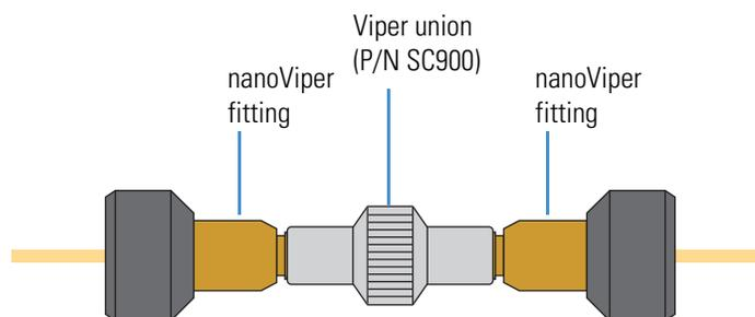
Figure 92 shows an internal view of the Viper union with nanoViper fittings connected to both ports. The two nanoViper fittings seal against each other in the center of the union, and a portion of the last thread on each nanoViper fitting is visible.
