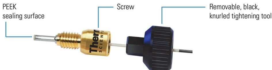
Even though nanoViper fittings can withstand UHPLC backpressures of up to ~1034 bar (~15 000 psi), they are fingertight fittings, which require only very small torques to seal. To avoid damage by overtightening, you must follow this procedure.
