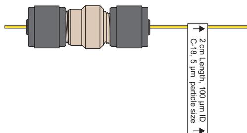
4. Using the tightening tool provided in the UHPLC Liquid Junction Kit, tighten the internally-threaded knurled nuts an additional one-quarter turn (Figure 71).
