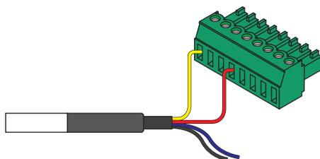
❖ **To connect the contact closure cable**
