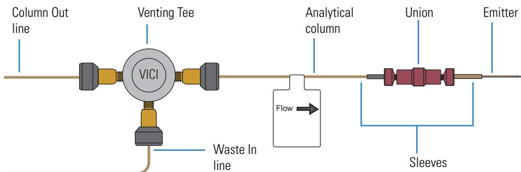
**Figure 9.** One-column setup for the EASY-nLC II instrument and Nanospray Flex source
