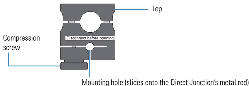
2. Slide the protective cover's body onto the DirectJunction's metal rod. If necessary, loosen the compression screw in the body until the hole in the body fits over the rod, and then tighten the screw.
