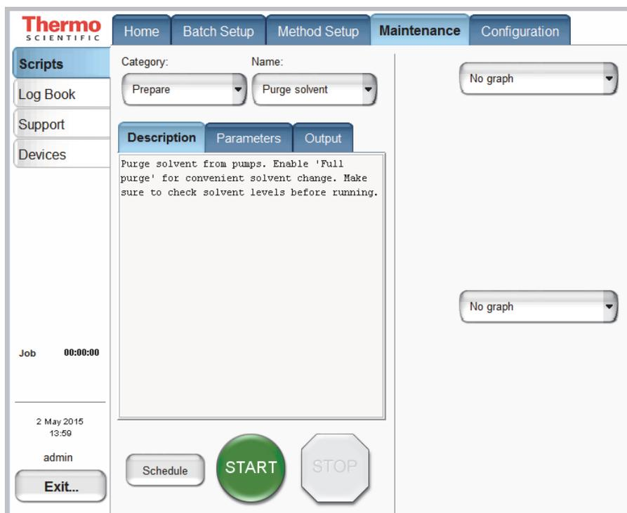
The green START button is active when a job or script is ready to execute. After you press START, the STOP button replaces the START button and remains active until the job or script ends. During execution you can terminate a job or script by pressing the red STOP button.
