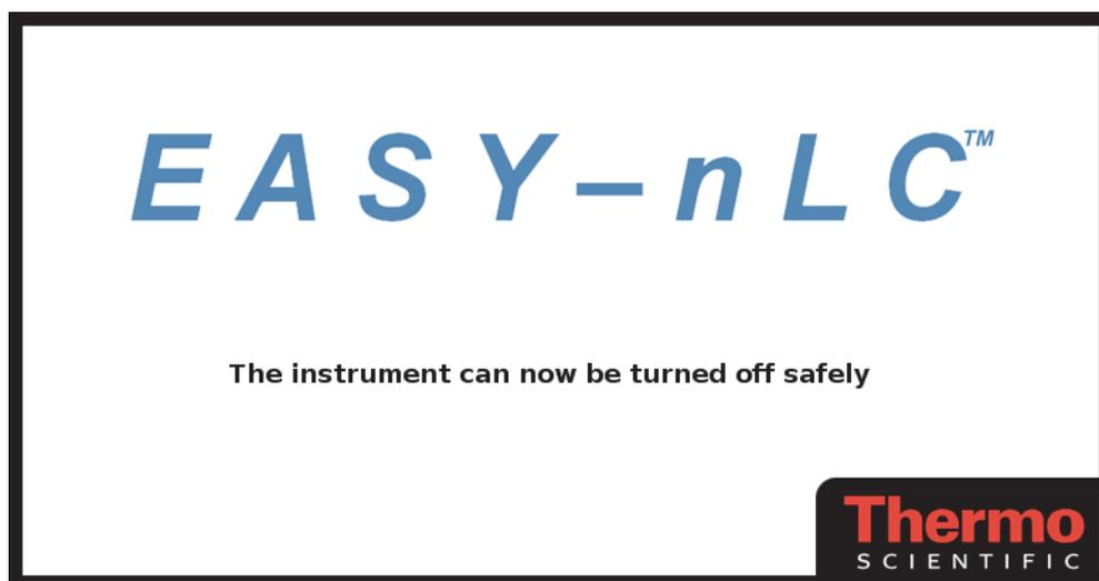
3. After receiving the message that you can safely turn off the instrument, turn off the power switch on the back panel of the instrument.
