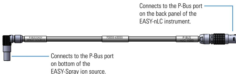
The EASY-nLC instrument provides power to the EASY-Spray ion source through the P-Bus cable.
