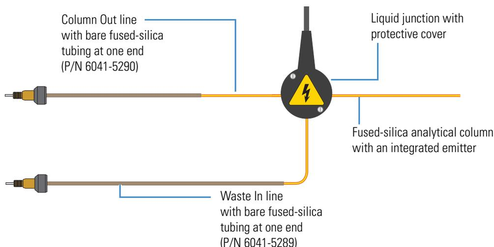
Figure 65 shows a two-column setup with the modified Column Out and Waste In lines and an analytical column with an integrated emitter. Both the precolumn and analytical column have bare fused-silica ends. The UHPLC fused-silica union connects the Column Out line to the precolumn's inlet.
