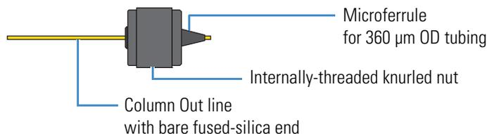
2. Insert the stainless steel cartridge into the deeper end of the externally-threaded PEEK holder (see Figure 66 on page 99). Then insert the Column Out line into the deeper end of the PEEK holder and hand-tighten the nut (Figure 69).
