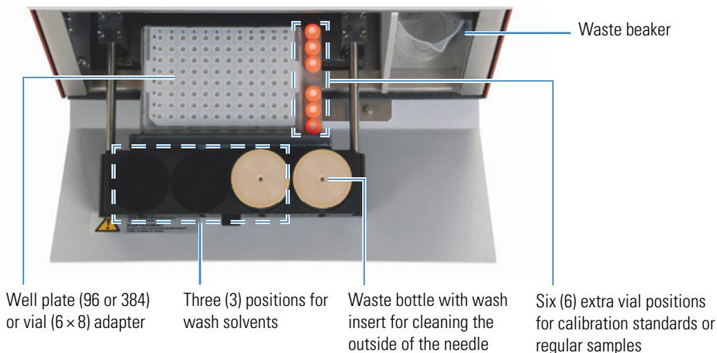
The tray compartment holds the sample tray and the wash bottles. The tray compartment for the ASC model holds an additional six vials. The compartment to the right of the tray compartment holds the waste beaker.
