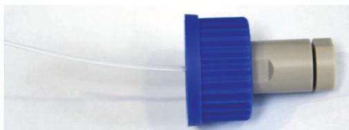
**IMPORTANT** To establish proper surface wetting, prime the filters with methanol or acetonitrile.
