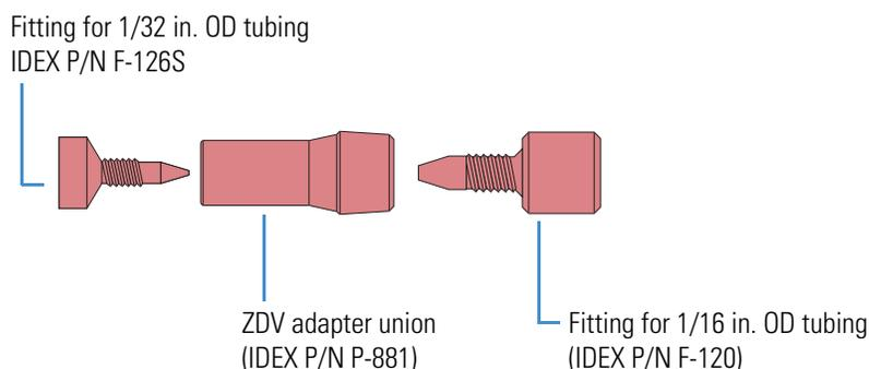
2. Using the ZDV adapter union and the one-piece fitting for 1/32 in. OD tubing, connect the Column Out line to a precolumn as follows:
