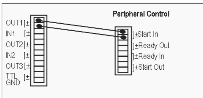
**Figure 31.** Two-way contact closure connection for an Orbitrap Fusion mass spectrometer
