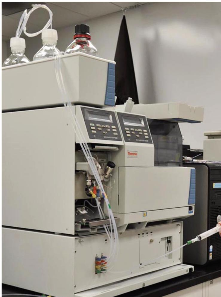
3. Slowly withdraw the syringe plunger so that air is drawn out of the degasser and solvent is drawn into the inlet tube.
