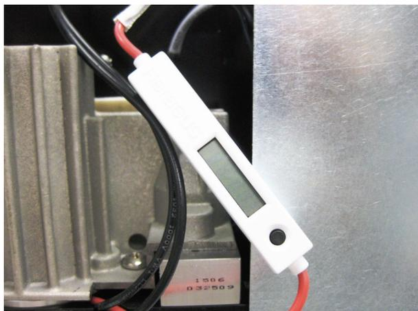
3. Press the black button on the meter once to view the hours on the meter's LCD panel.
