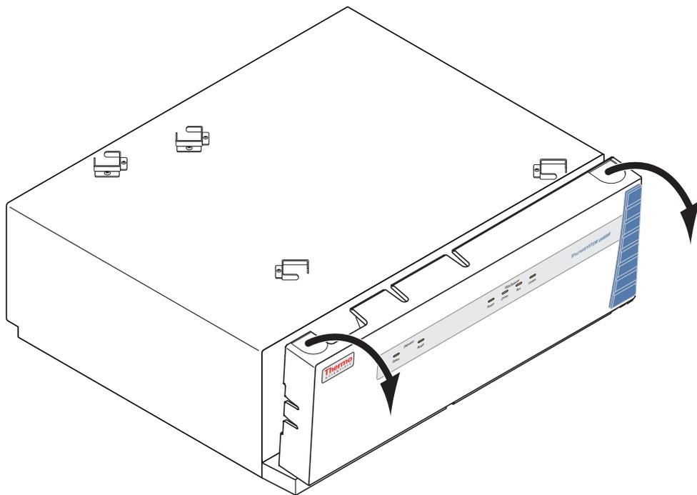
3. Unscrew the captive screw that secures the LightPipe flowcell access cover to the front panel of the detector and pull the cover off (Figure 70).
