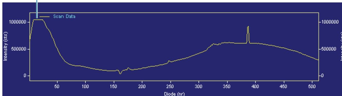
Figure 59 shows a diode array that is saturated in both the UV and visible regions. The configuration is set to a 20 Hz diode array scan rate and the attenuators are completely open.
