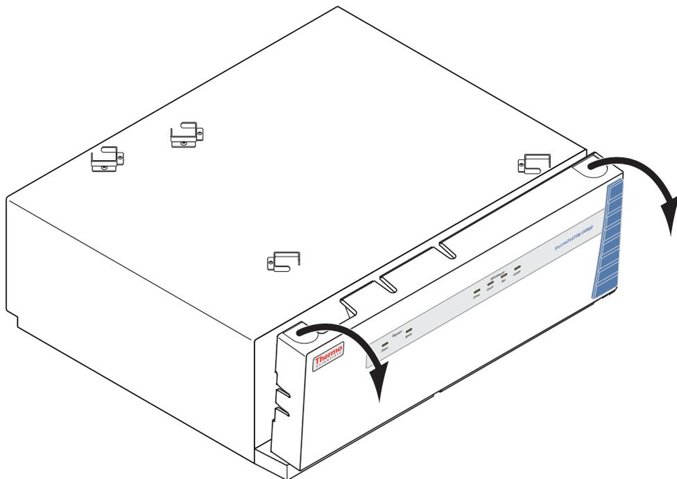
2. Unscrew the captive screw that secures the LightPipe flowcell access cover to the front panel of the detector and pull the cover off (Figure 12).
