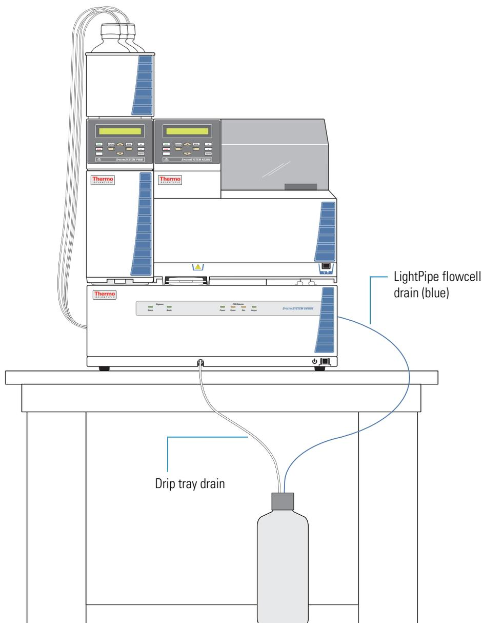
2. Connect the LightPipe flowcell outlet tubing to a sealed waste bottle (Figure 36).
