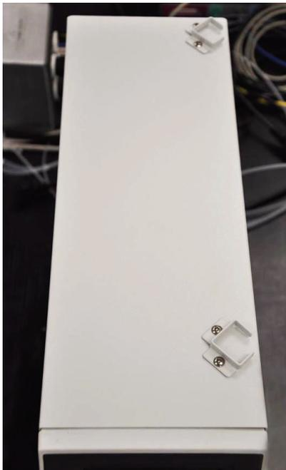
2. Position the pump on the top left area of the UV8000 module, placing two of the feet on the pump in the two brackets on the left.
