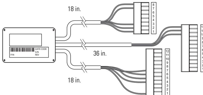
Connecting the UV8000 module requires an adapter cable (Figure 19).
