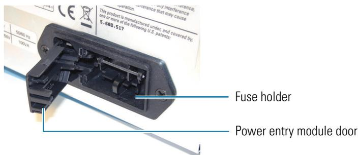
4. Take the loose fuse holder out of the power entry module ([Figure 82](#)).
