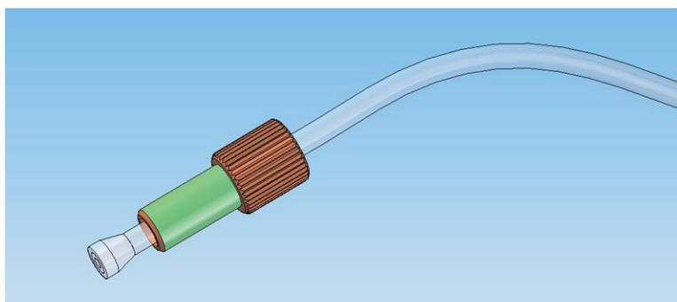
Note the orientation of the ferrule on the tubing.
