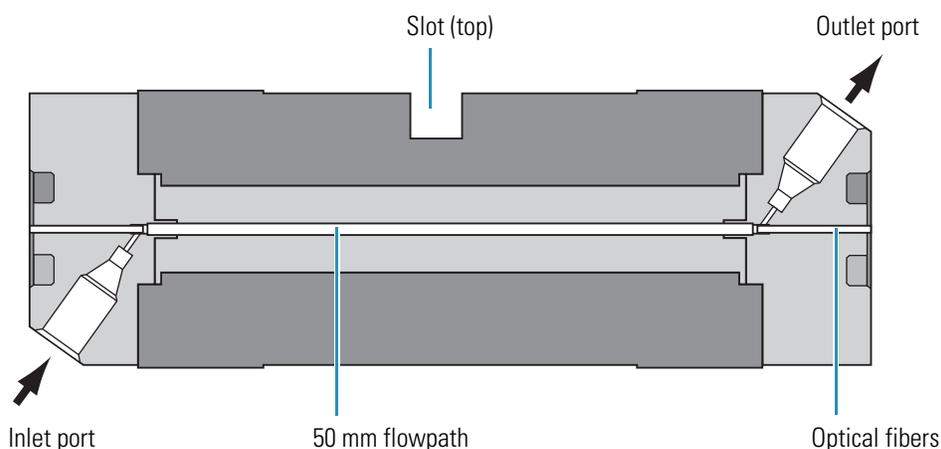
Sensitive optical fibers are exposed at both ends of the LightPipe flowcell (Figure 4). Thermo Fisher Scientific ships the LightPipe flowcell with end caps to protect these optical fibers (Figure 5). Do not remove the protective end caps until you install the LightPipe flowcell. Replace the protective end caps for storage if you remove the LightPipe flowcell from the detector.
