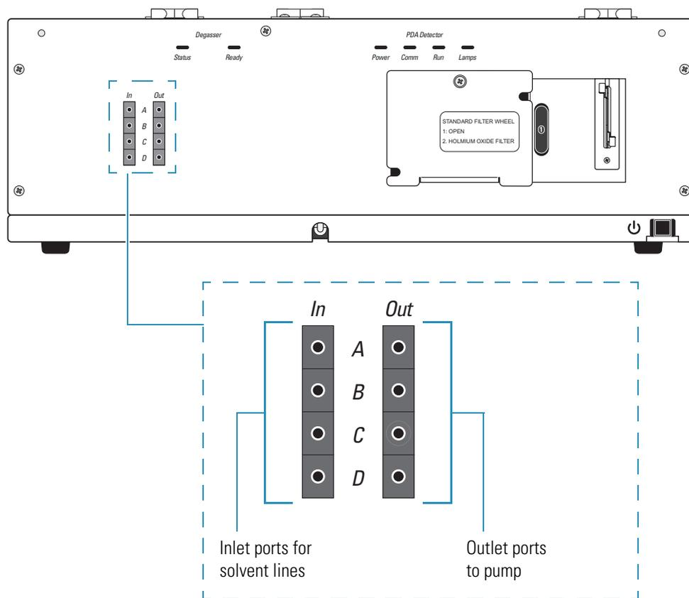
4. Connect the solvent lines with their colored flangeless fittings to the inlet ports of the degasser (Figure 28).
