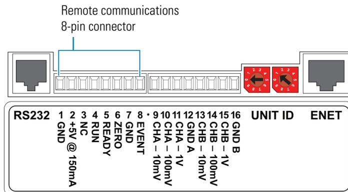
**Tip** When the UV8000 module is part of an LC system, connect the system interconnect cable to these terminals (see “Synchronizing the Instrument Modules During an Injection Sequence” on page 25).
