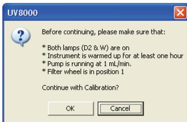
5. Make sure that the lamps are warmed up, that the pump is running at 1 mL/min, and that the filter wheel is in position 1 (Figure 39 on page 47).
