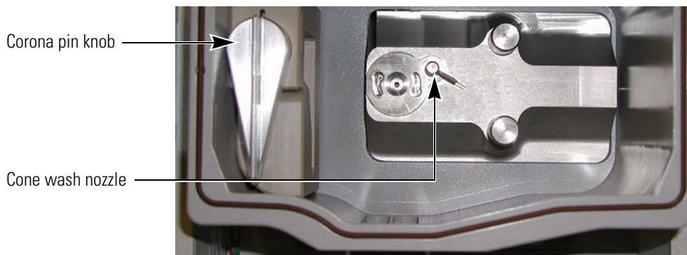
Figure 73. View of the source block, showing the cone wash nozzle turned to the right
