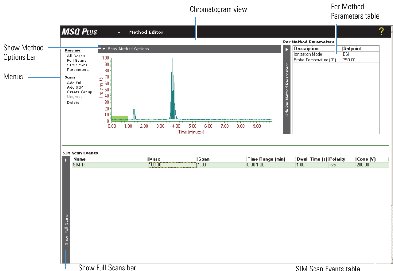
Figure 42. Method Editor with menus, Chromatogram view, Per Method Parameters table, and SIM Events table visible
