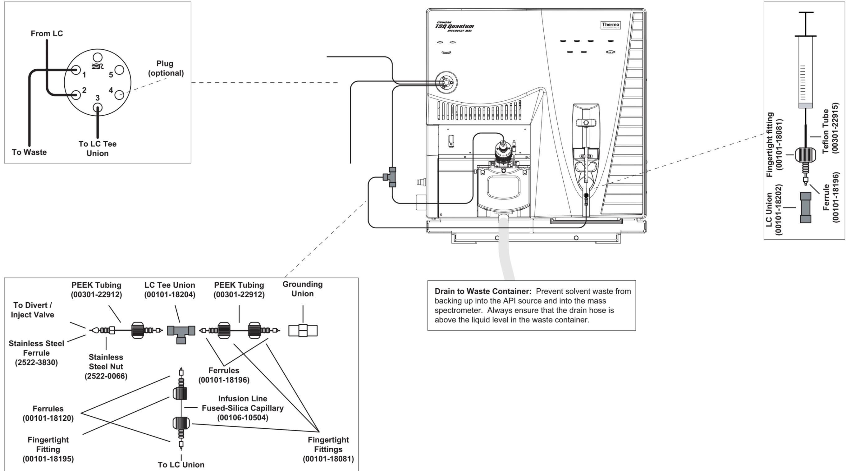
**Figure 12-6.** Plumbing diagram, showing APCI/MS sample introduction from the syringe pump connected via an LC TEE into the solvent flow from an LC
