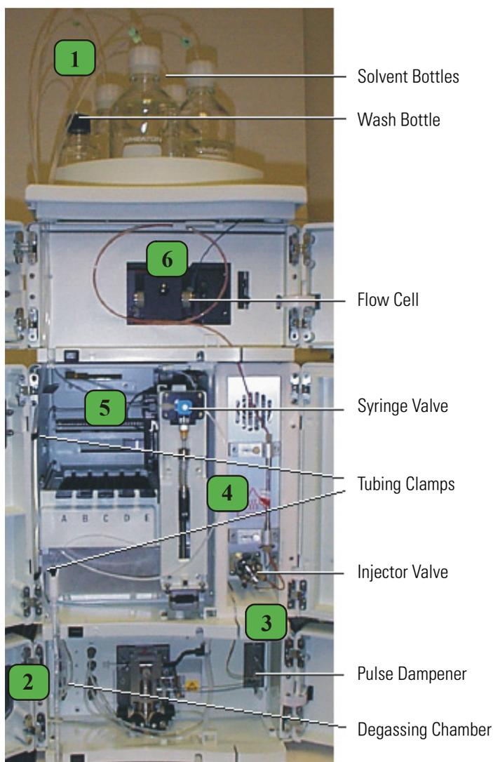
**Figure 4-4.** Surveyor LC system (with MS Pump) plumbing
