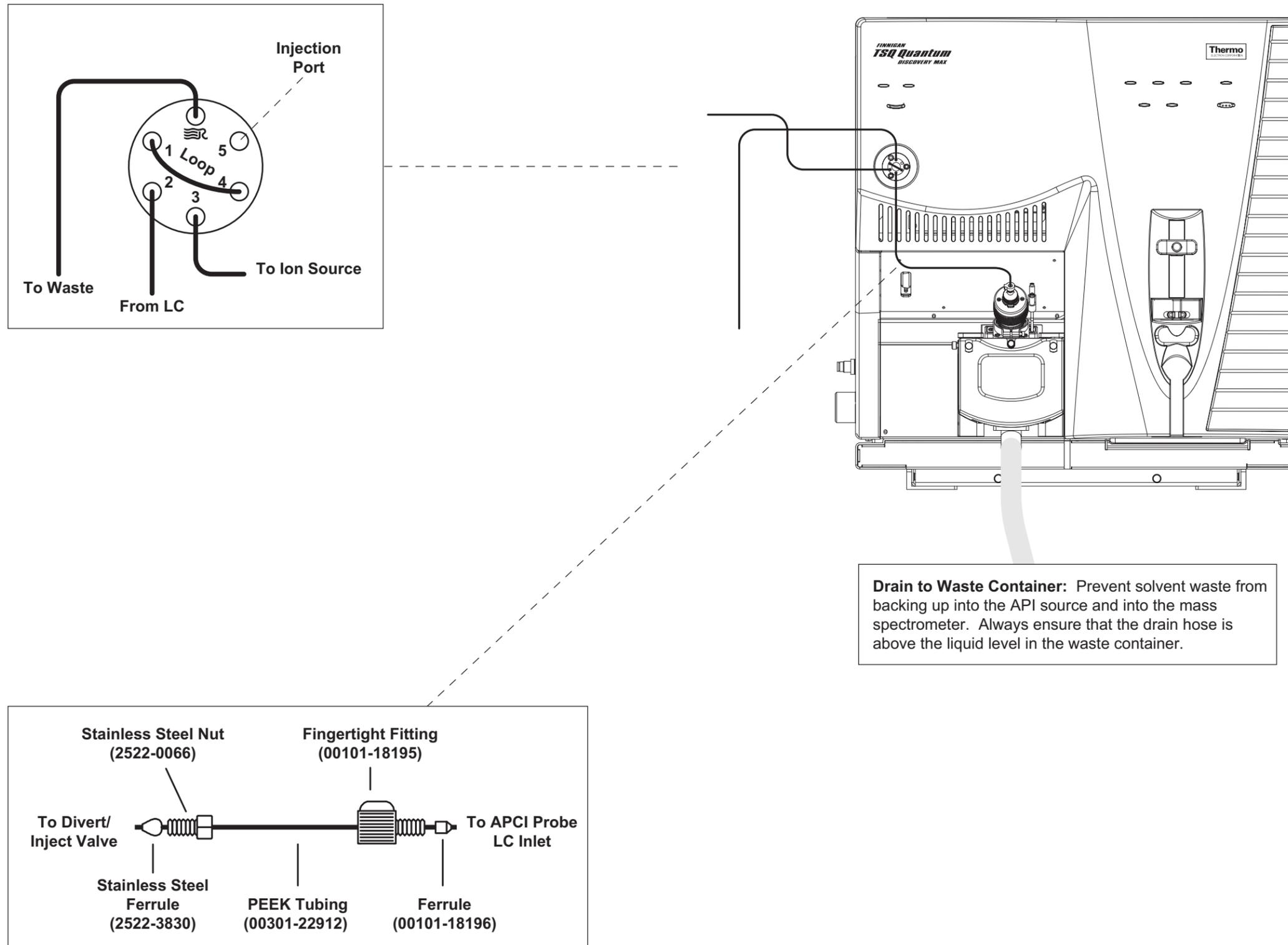
**Figure 12-7.** Plumbing diagram, showing APCI/MS sample introduction by loop injection into the solvent flow from an LC
