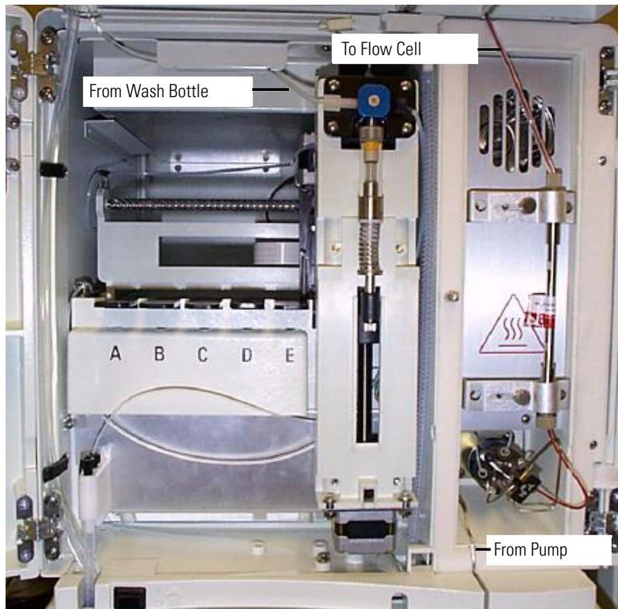
**Figure 4-7.** Surveyor Autosampler plumbing
