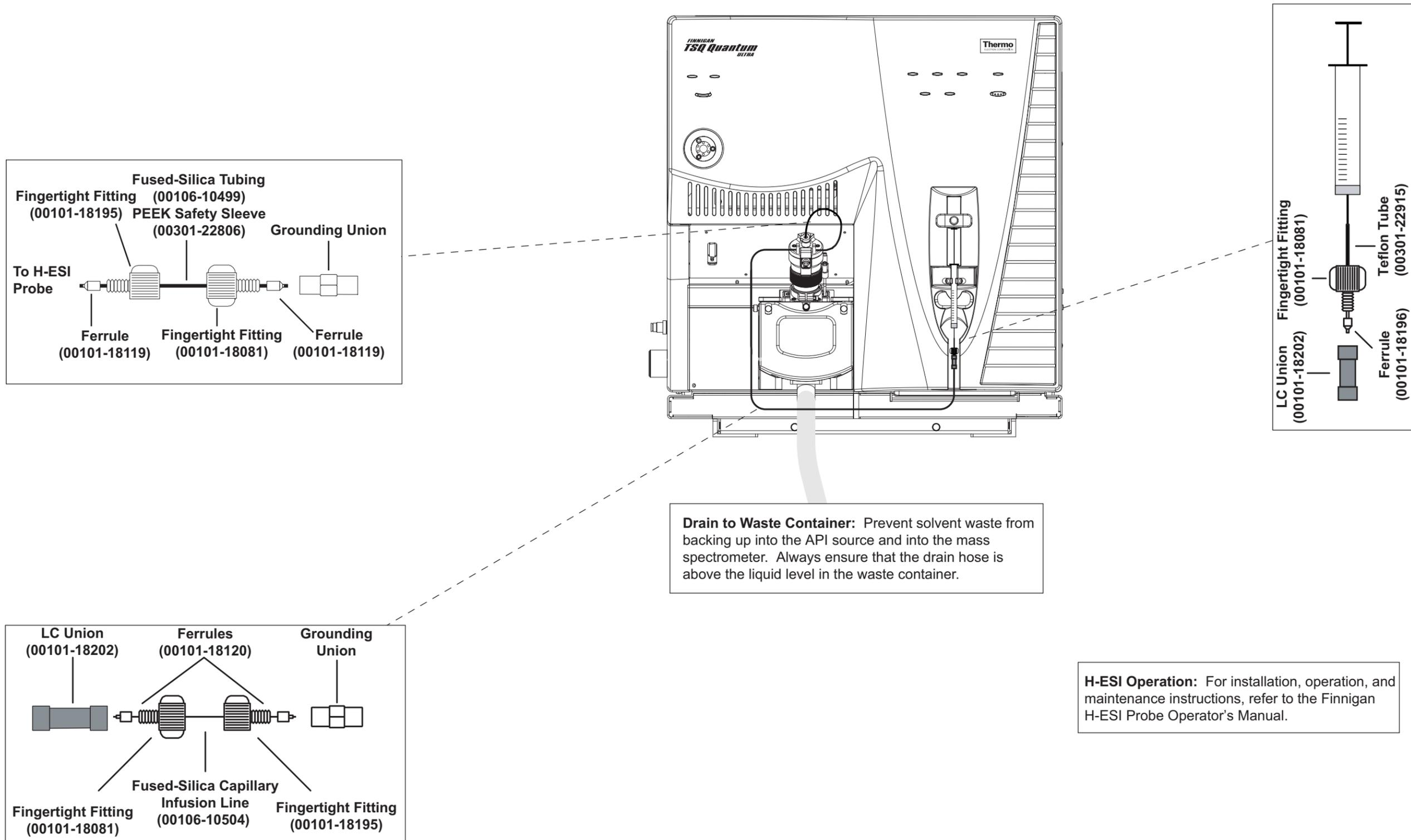
**Figure 12-1.** Plumbing diagram showing H-ESI/MS sample introduction from the syringe pump
