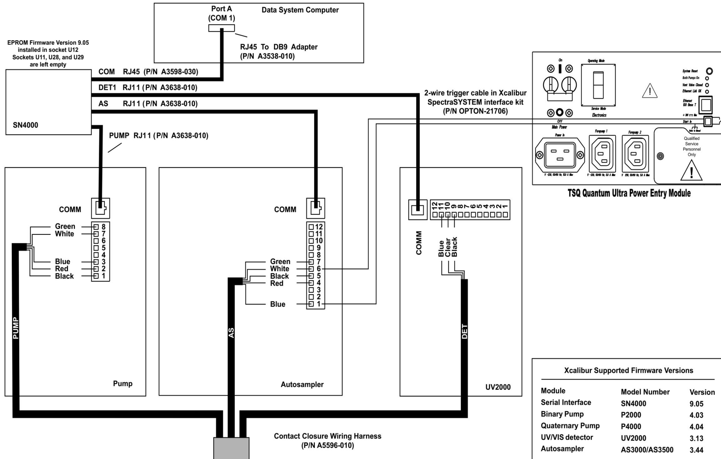
**Figure 5-1.** Schematic diagram showing the cable connections for the TSQ Quantum Ultra and a SPECTRASystem equipped with a pump, autosampler, and UV2000 detector
