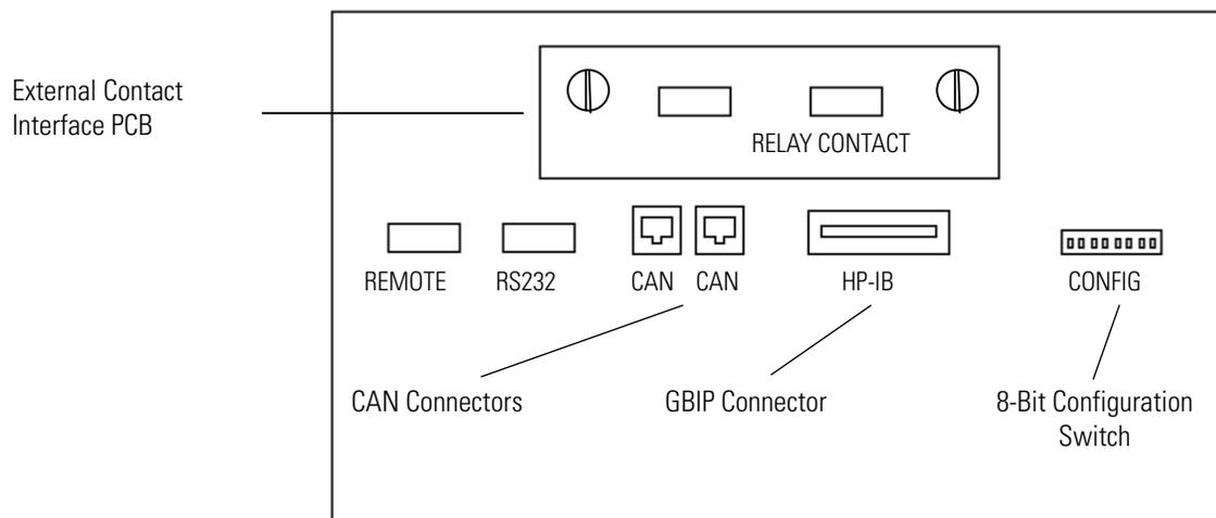
**Figure 6-8.** HP 1100 Series Autosampler rear panel
