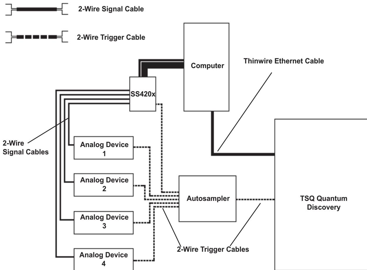
**Figure 10-1.** Wiring diagram showing four analog devices connected to the SS420x and autosampler. Each analog device is connected with a 2-wire signal cable and 2-wire trigger cable (contact closure).
