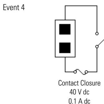
**Figure 6-4.** HP 1090 Series LC rear panel EVENT 4 connector
