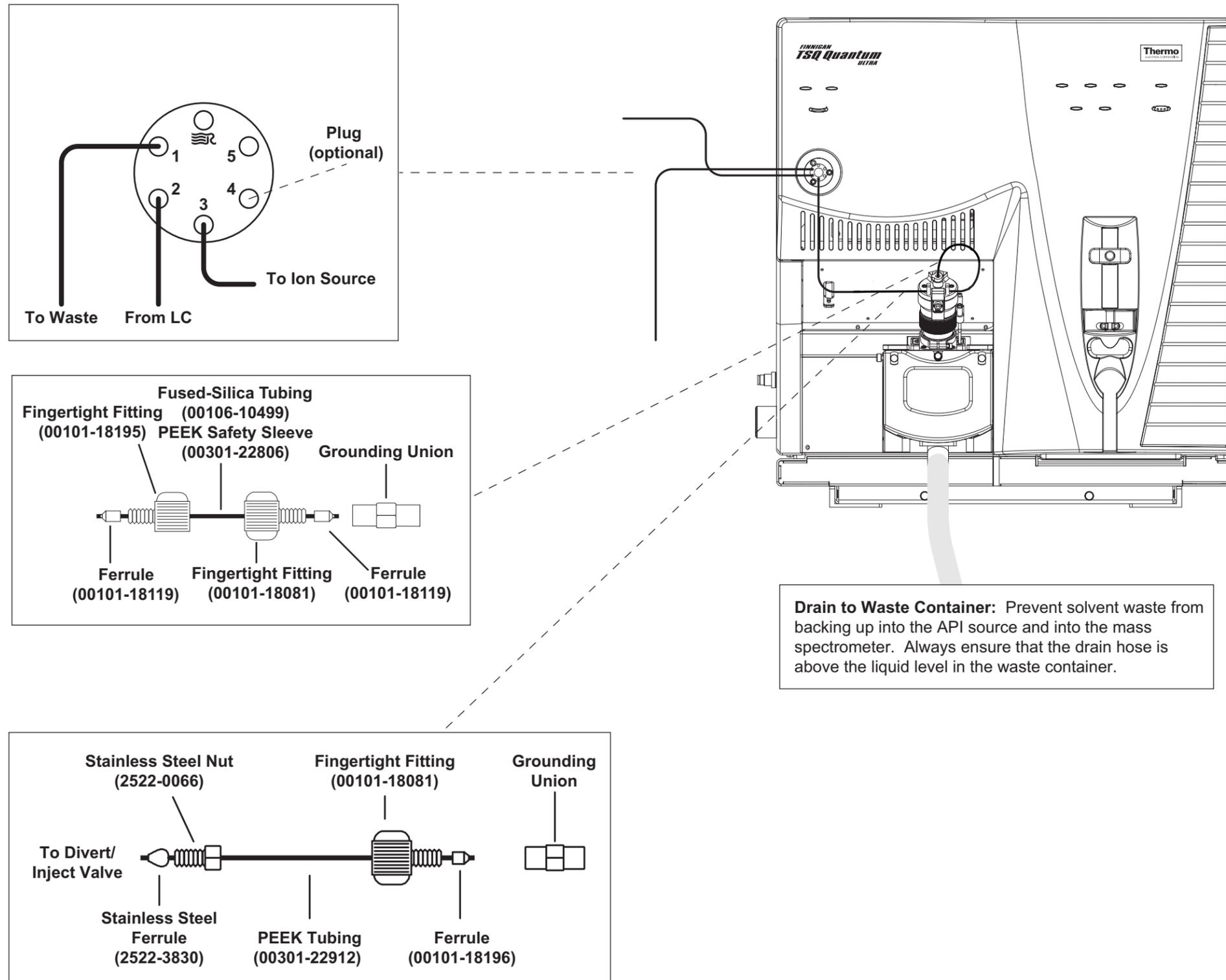
**Figure 12-4.** Plumbing diagram showing H-ESI/MS sample introduction from an LC autosampler with or without chromatographic separation
