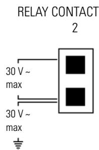
**Figure 6-1.** HP 1050 Series Autosampler rear panel RELAY CONTACT 2 connector
