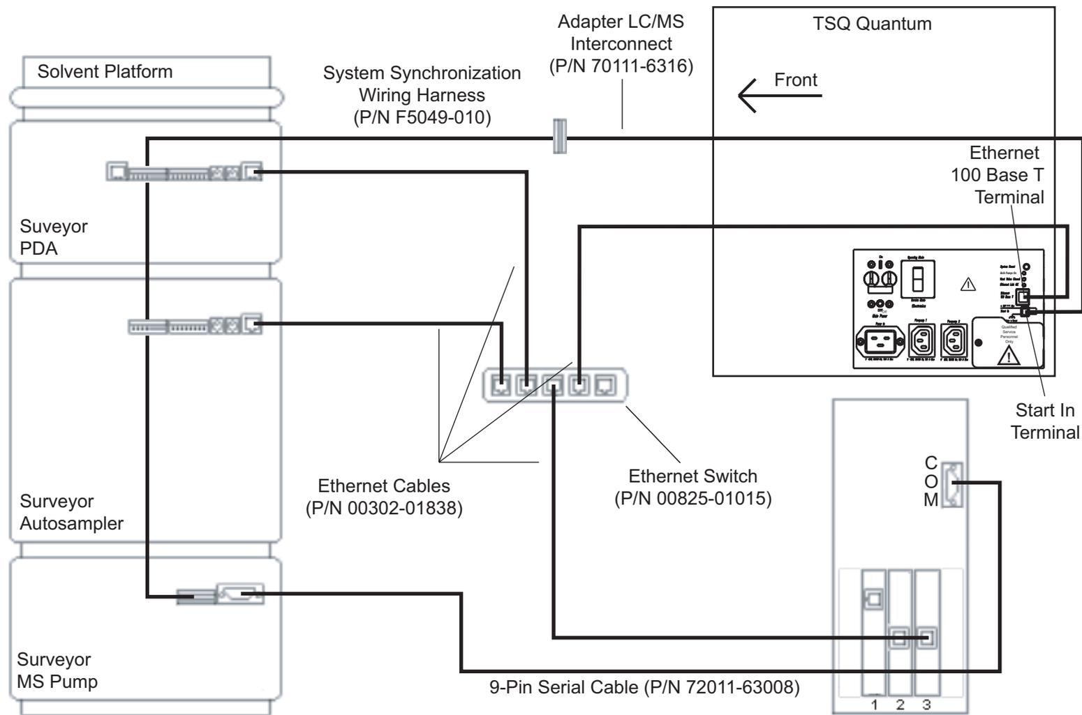
**Figure 4-2.** Cable diagram for the Surveyor LC system with an MS Pump, TSQ Quantum Ultra, and data system computer
