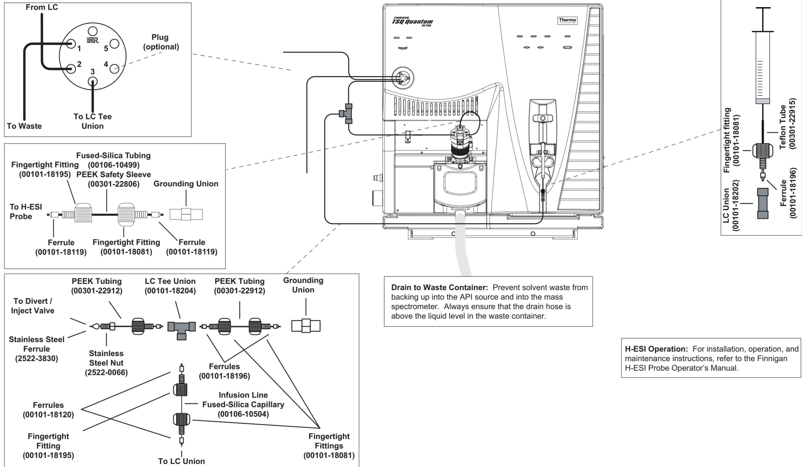
**Figure 12-2.** Plumbing diagram showing H-ESI/MS sample introduction from the syringe pump connected via an LC TEE union into the solvent flow from an LC
