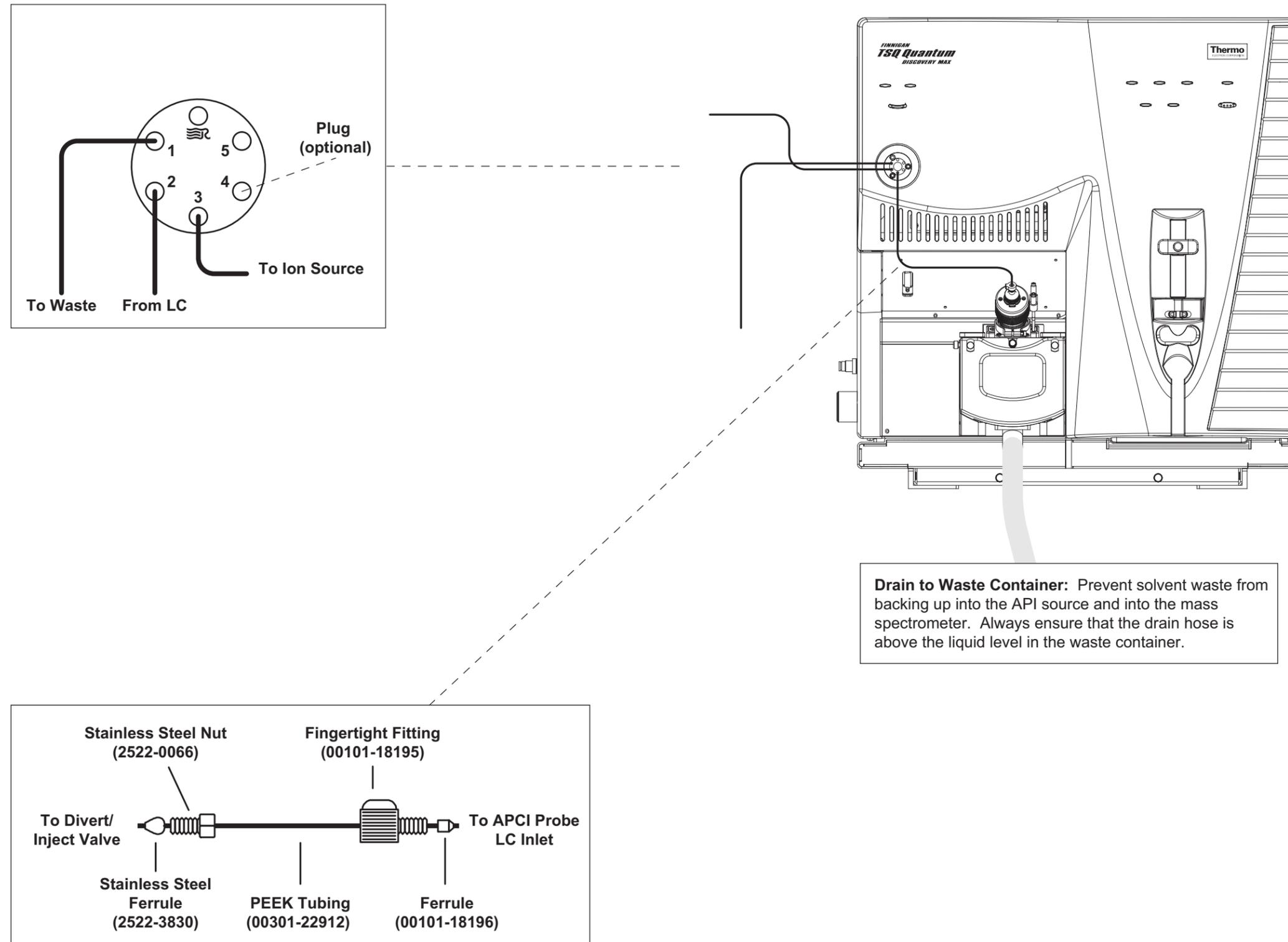
**Figure 12-8.** Plumbing diagram, showing APCI/MS sample introduction from an LC autosampler with or without chromatographic separation
