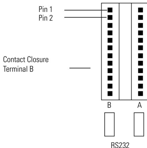
**Figure 8-1.** Waters Alliance 2690 Separations Module rear panel contact closure terminals
