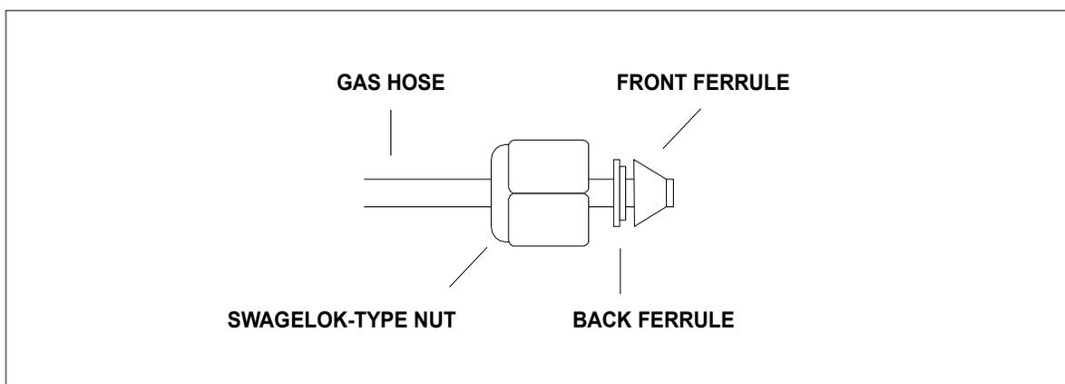
**Figure 1-1.** Proper orientation of the Swagelok-type nut and two-piece ferrule
