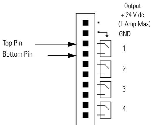
**Figure 9-1.** Gilson 215 Liquid Handler rear panel OUTPUT contact closure terminal
