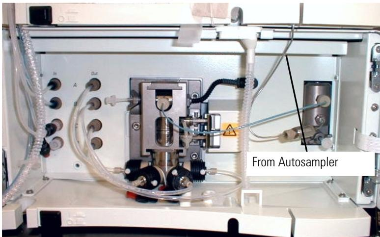
**Figure 4-5.** Surveyor MS Pump plumbing
