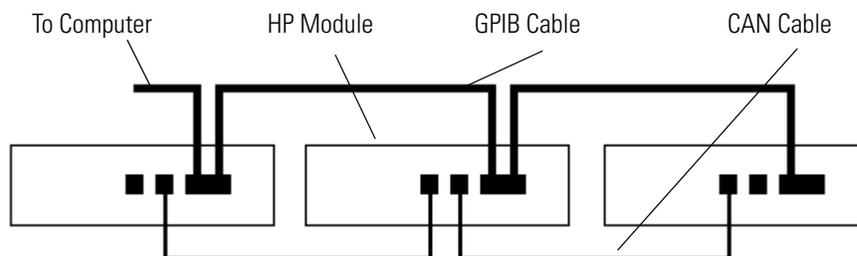
**Figure 6-7.** Daisy-chain interconnection of HP 1100 Series modules with CAN and GPIB cables
