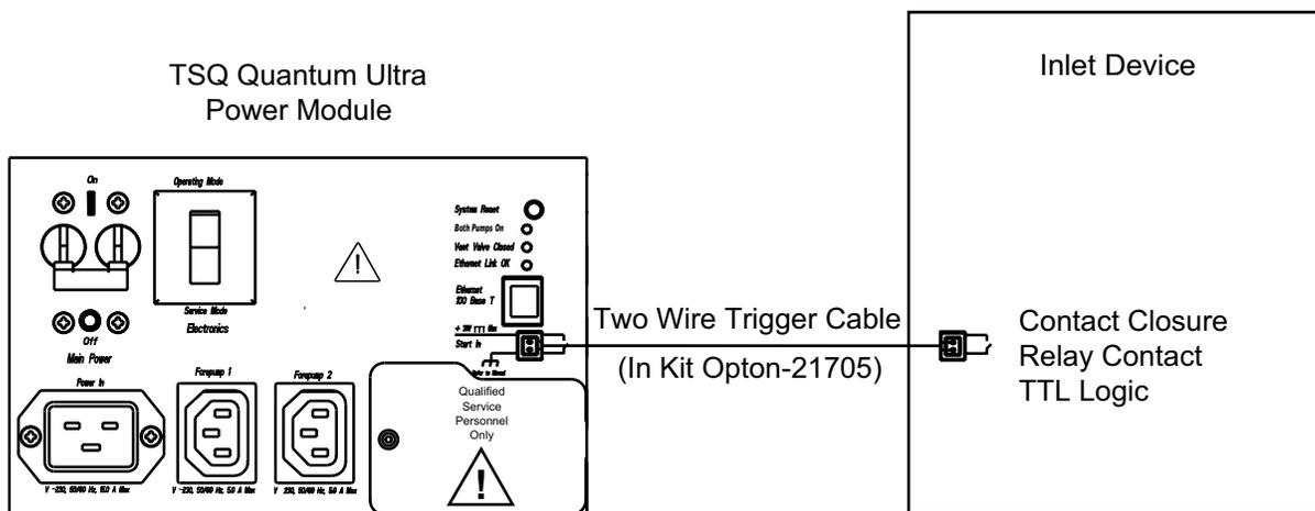
**Figure 3-1.** Portion of the power entry module showing contact closures for the TSQ Quantum Ultra and an external device
