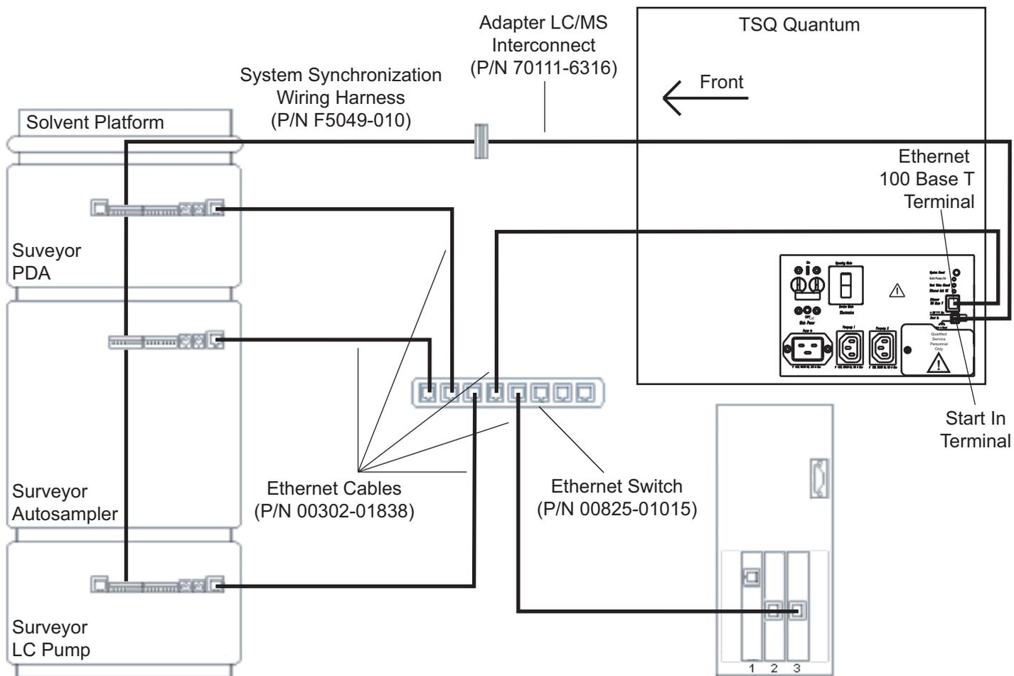
**Figure 4-3.** Cable diagram for the Surveyor LC system with an LC Pump, TSQ Quantum Ultra, and data system computer
