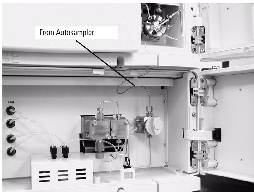
**Figure 4-6.** Surveyor LC Pump plumbing
