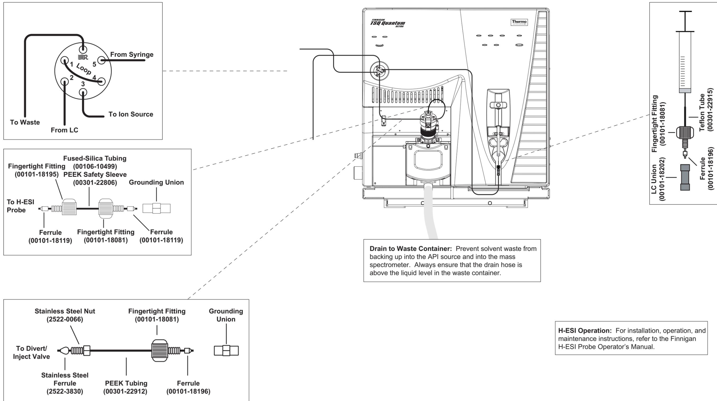
**Figure 12-5.** Plumbing diagram showing H-ESI/MS sample introduction by loop injection into the solvent flow from an LC
