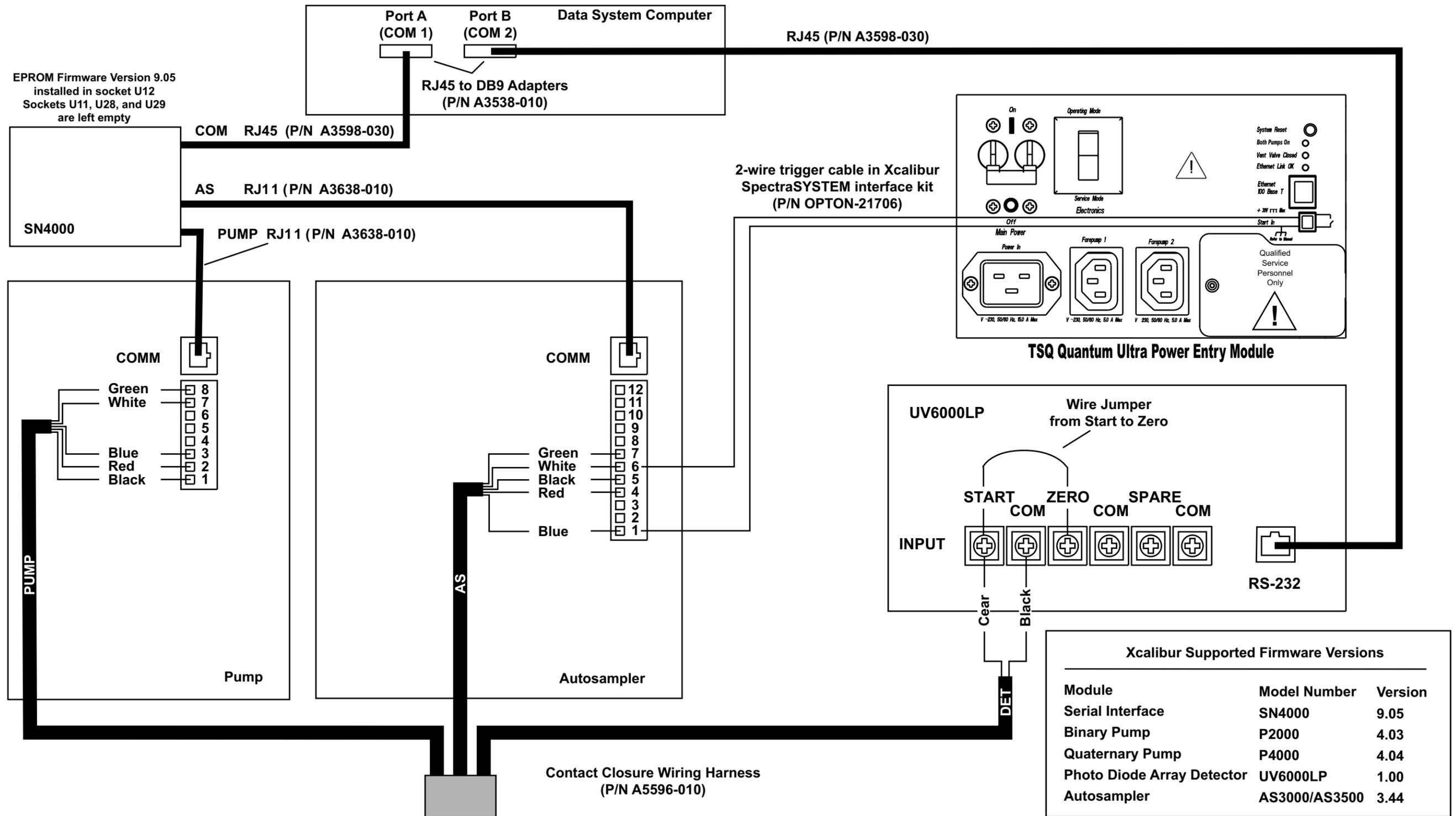
**Figure 5-3.** Schematic diagram showing the cable connections for the TSQ Quantum Ultra and a SPECTRASYSTEM equipped with a pump, autosampler, and UV6000LP detector
