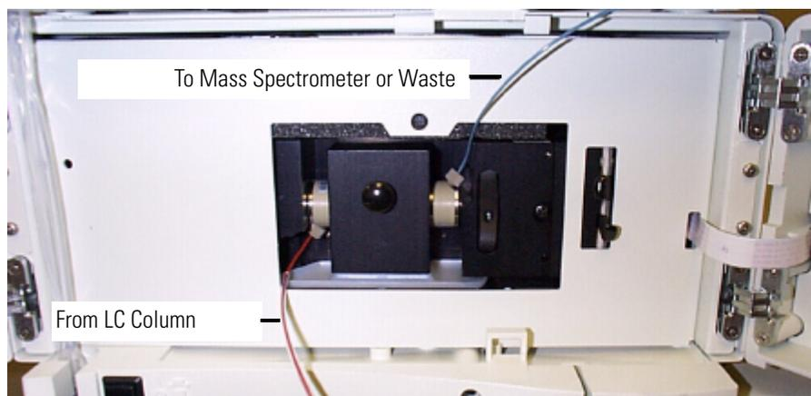
**Figure 4-8.** Surveyor LC System plumbing, showing the flow cell
