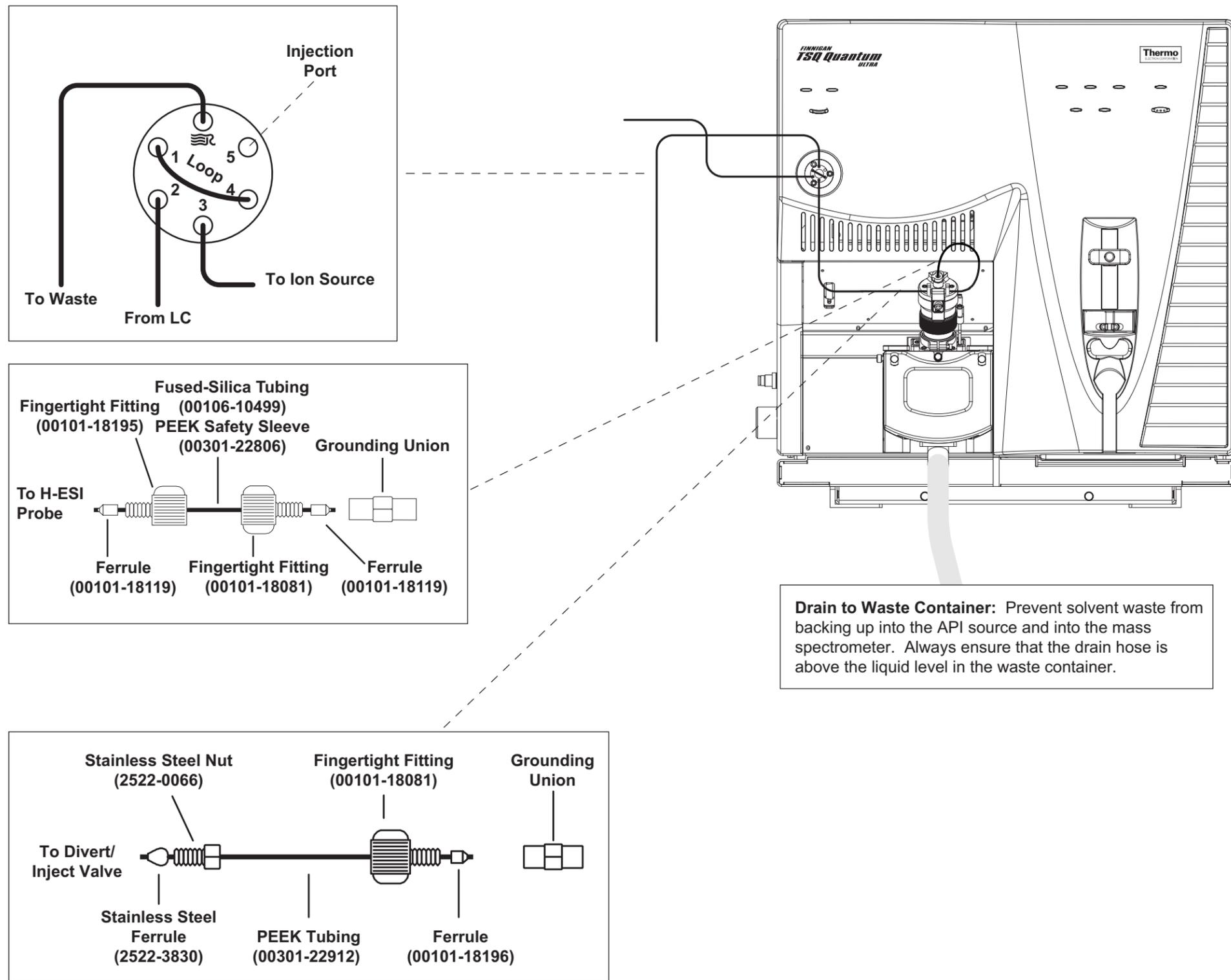
**Figure 12-3.** Plumbing diagram showing H-ESI/MS sample introduction by loop injection into the solvent flow from an LC
