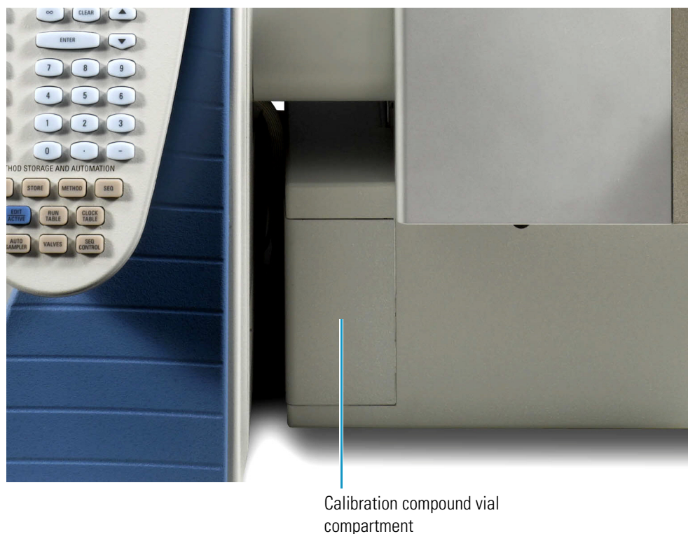
Figure 57. Location of the calibration compound vial compartment
