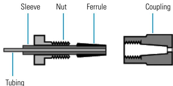
Disconnecting and then reconnecting coupling unions involving fused silica tubing and tubing sleeves is not recommended. Once you disconnect a coupling joint, you compromise the sleeve and ferrule component for further use. Discard or replace used fittings; do not reuse them.
