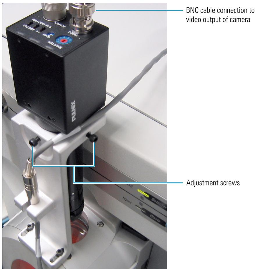
2. Connect one end of the BNC cable to the Video port on the top of the camera. Connect the other end of the BNC cable to the video capture card.
