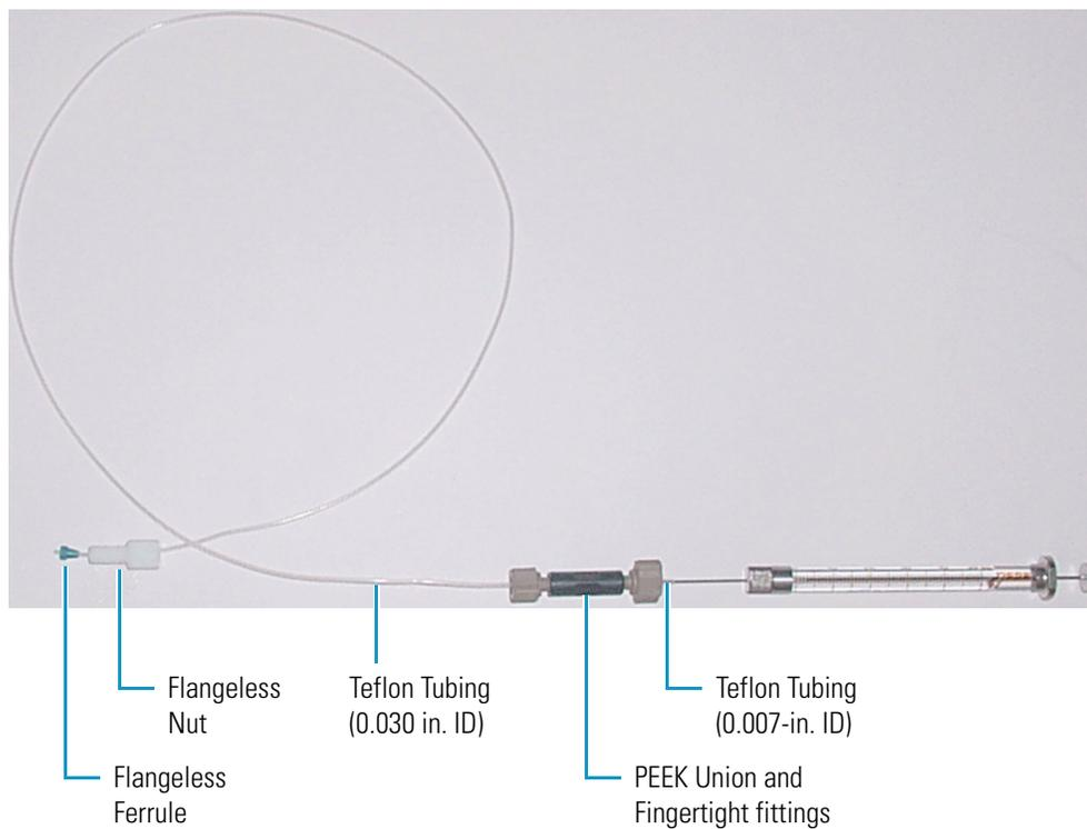
**Figure 67.** View of the static NSI probe, showing the gas inlet
