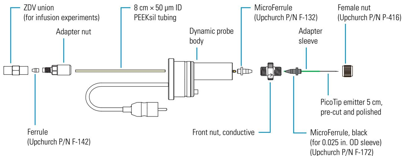
**IMPORTANT** To avoid performance failures, use these recommended parts. Order pre-cut, 8 cm length, 50  $\mu\text{m}$  ID, PEEKsil tubing (natural) from Upchurch Scientific. See [Figure 38](#). Order pre-cut and polished, 5 cm length, PicoTip emitters from New Objective, Inc. The performance of the dynamic nanospray probe depends on the tolerances of these components.
