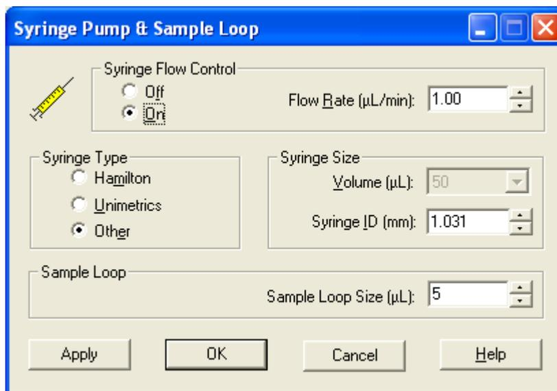
2. In the Syringe Flow Control group box, select the On option button to enable the Flow Rate spin box. Then, set the syringe pump flow rate to 1 µL/min by typing 1 in the Flow Rate combo box.
