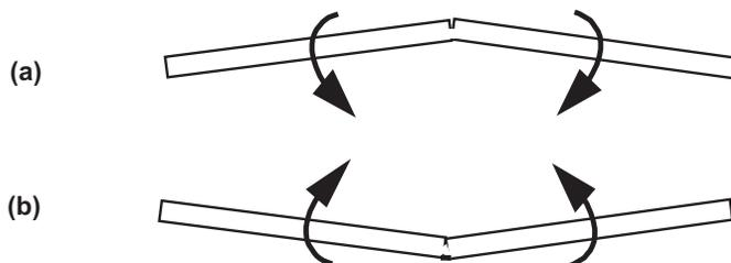
4. Examine the snapped-off end at a magnification of 10× to 30× to ensure that the cut is square and smooth. If the cut is not square or smooth discard the piece of tubing or cut its end again.
