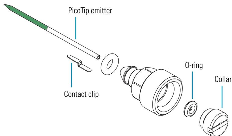
4. Using tweezers, gently push the emitter further into the nose cone tip until 5 to 8 mm of the emitter protrudes through the end of the tip. Ensure that the metal contact clip touches the coating on the emitter.
