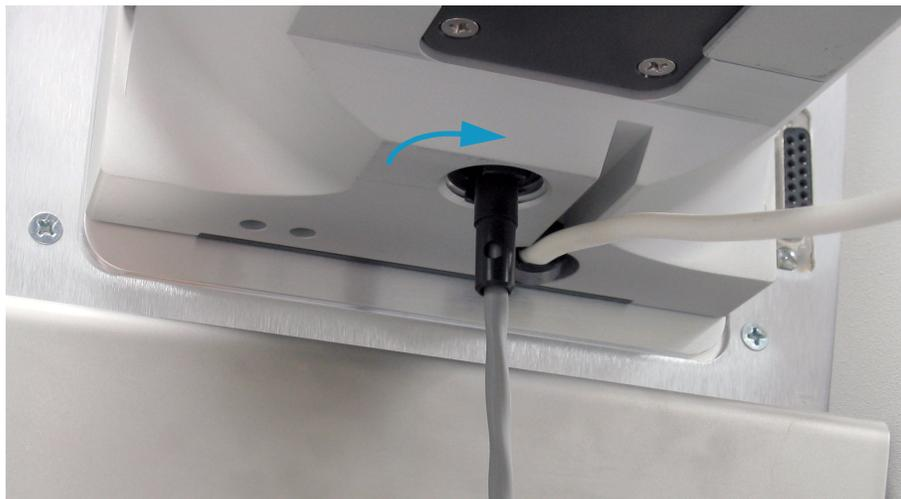
3. Route the LED cable through the bracket in the camera stand.
