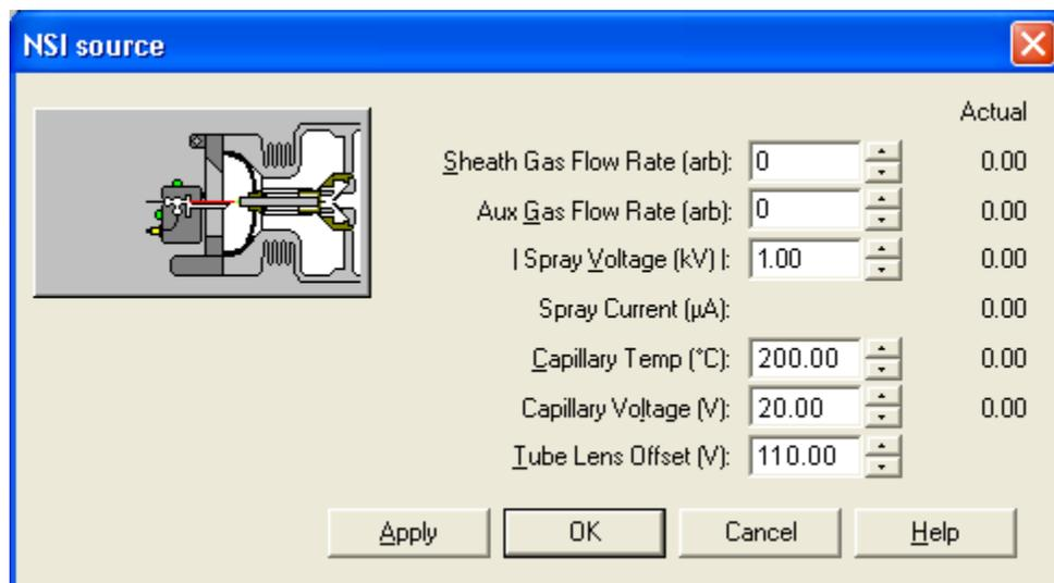
4. Ensure that the setting for the spray voltage is at ( $\pm$ )1.0 kV and that the setting for the sheath gas flow rate is at 0. Sheath gas is not used for a static NSI source.
