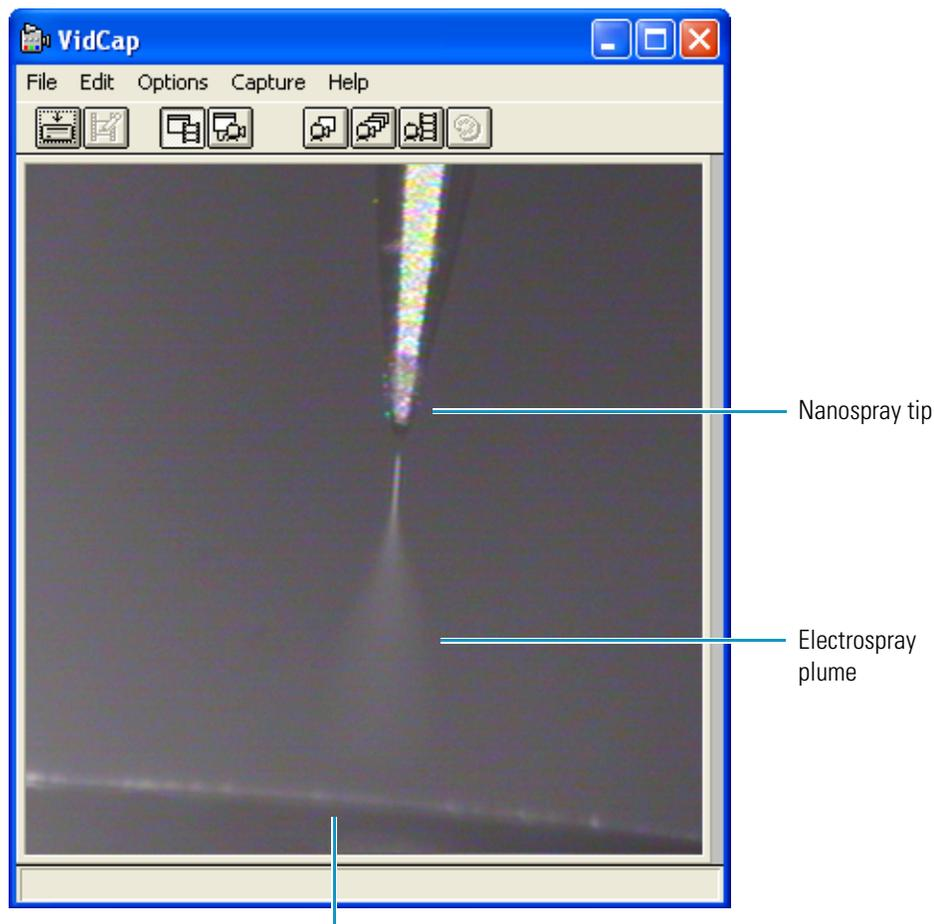
Light is positioned directly beneath ion transfer tube to backlight nanospray droplets. Note corona effect on inlet.
