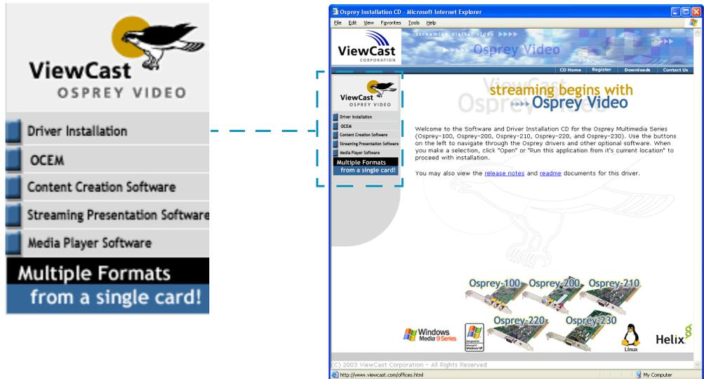
2. In the navigation bar on the left, click Driver Installation to expand the list of Microsoft operating systems supported by the Osprey video capture system. See Figure 87.
