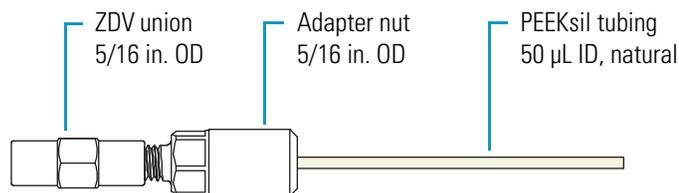
2. Connect the PEEKsil tubing to the dynamic nanospray probe:
