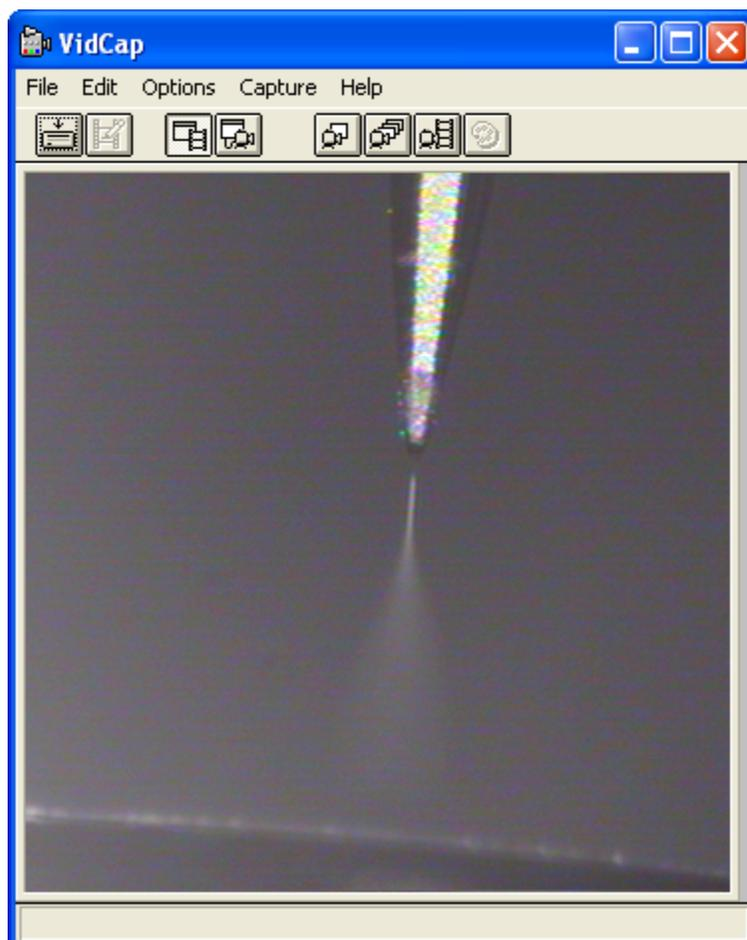
The installation of the Osprey MultiMedia Capture system is completed successfully if you can view the nanospray tip from the Osprey MultiMedia Capture application.
