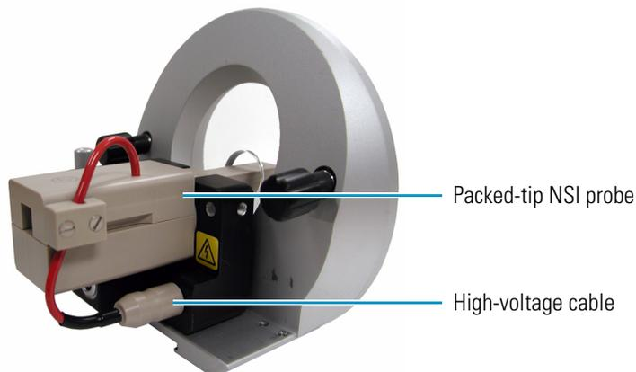
**Figure 59.** NSI source with static NSI probe
