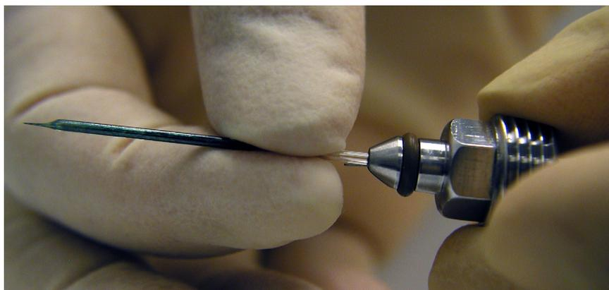
3. If you cannot fit the flat end of the emitter through the tip of the nose cone, remove the emitter and use a flat head screwdriver to adjust the collar inside the nose cone tip as follows (see [Figure 33](#) and [Figure 34](#)):
