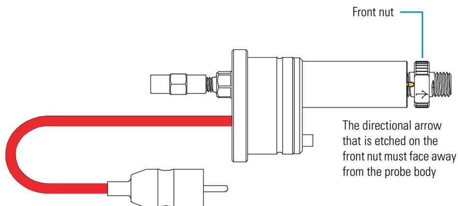
3. Connect a PicoTip emitter to the front of the probe as follows:
