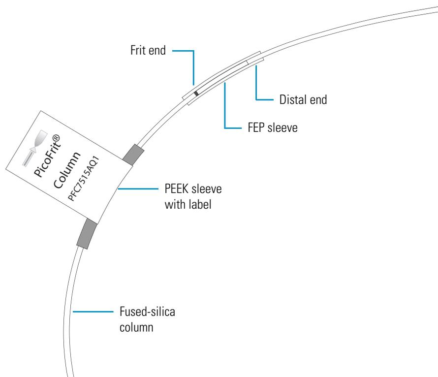
3. Remove the distal end of the column from the loop by pulling it free from the sleeve or by cleaving the fused silica tubing near the distal end. Leave the tapered tip end of the column in the FEP sleeve until the column is ready for mounting on the packed-tip NSI probe.
