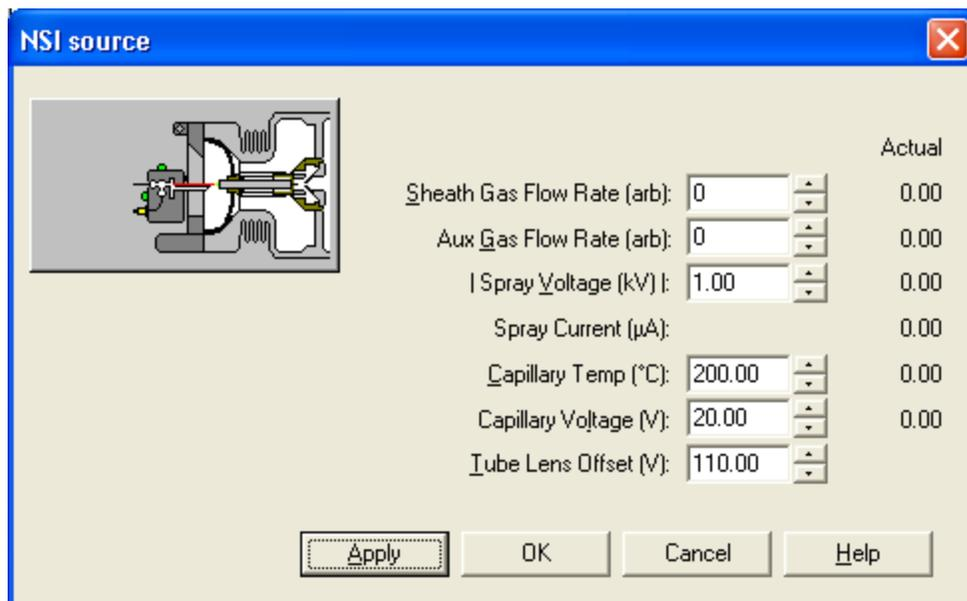
5. Ensure that the setting for the spray voltage is at ( $\pm$ )1.0 kV and that the setting for the sheath gas flow rate is at 0. Sheath gas is not used for a static NSI source.
