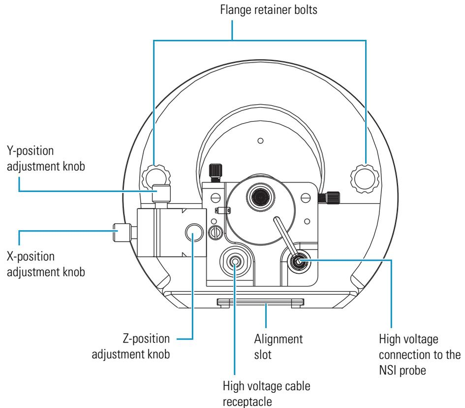
3. Align the NSI source alignment slot with the alignment tab on the NSI extension assembly. Then, slide the NSI source onto the extension assembly.
