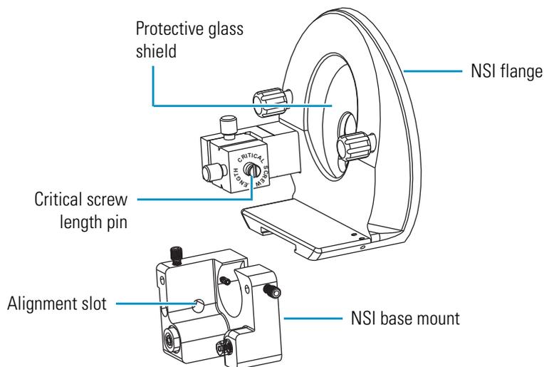
2. Using a #1 Phillips head screwdriver, tighten the screw that secures the NSI base mount to the NSI flange.
