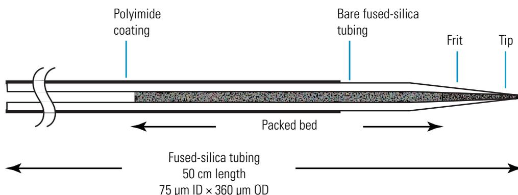
PicoFrit columns are shipped in lengths of 50 cm fused-silica tubing. The ends of the column are protected by a piece of clear FEP tubing forming a loop. The PicoFrit column is stored in solvent, which keeps the distal end and the tapered tip end of the column at the same pressure during storage and shipping, and prevents the column from drying out.
