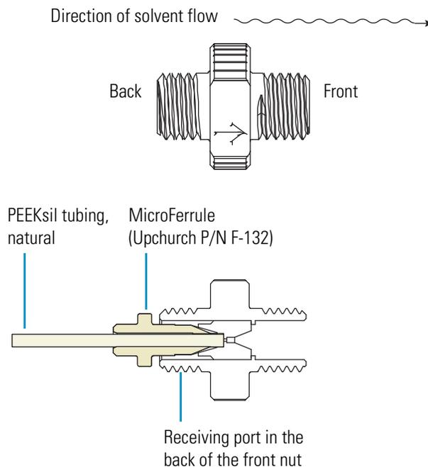
The directional arrow that is etched on the front nut must face away from the probe body. See [Figure 44](#).
