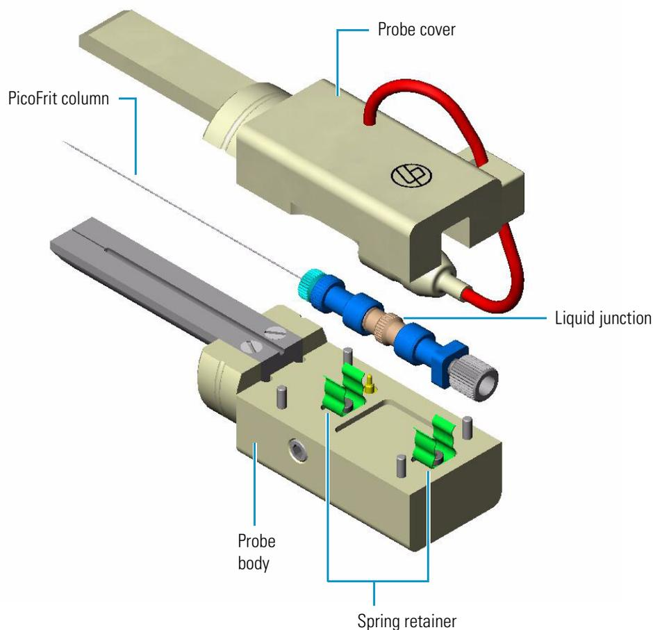
**Figure 51.** Liquid junction of the packed-tip NSI probe
