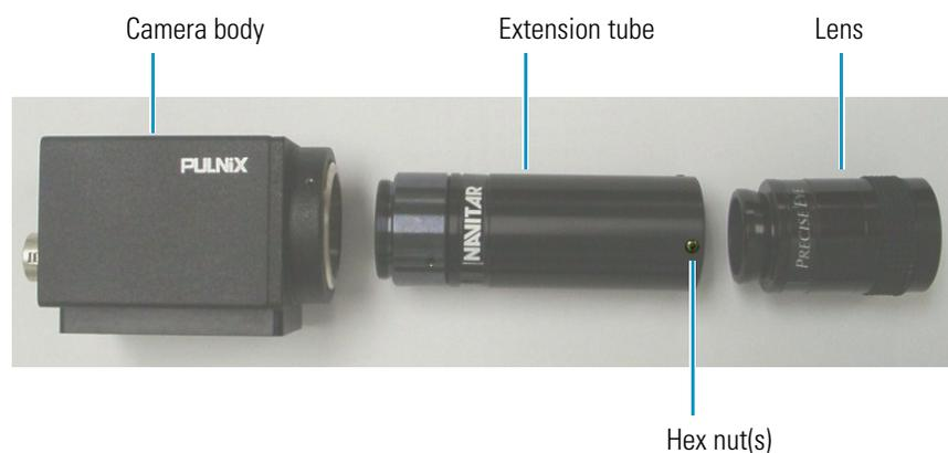
The CCD camera and optics system is now assembled and is ready to be installed on the camera stand as described in the next section, [“Installing the Camera Assembly.”](#)
