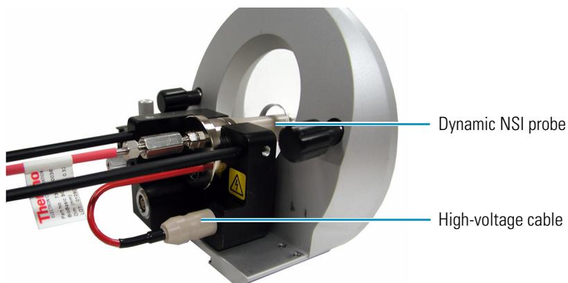
**Figure 58.** NSI source with packed-tip NSI probe
