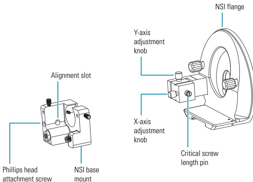
The flange contains the XYZ stage, which is used to make fine adjustments to the position of the NSI probe. The NSI base mounts to the NSI flange and holds the NSI probe. A dynamic NSI source is shown in [Figure 3](#).
