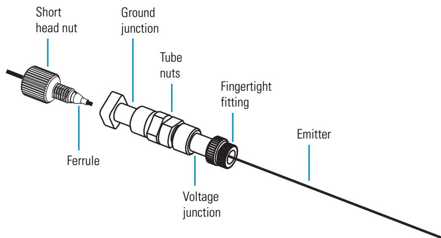
8. Using the fingertight fitting, connect a new emitter to the voltage junction of the liquid junction.
