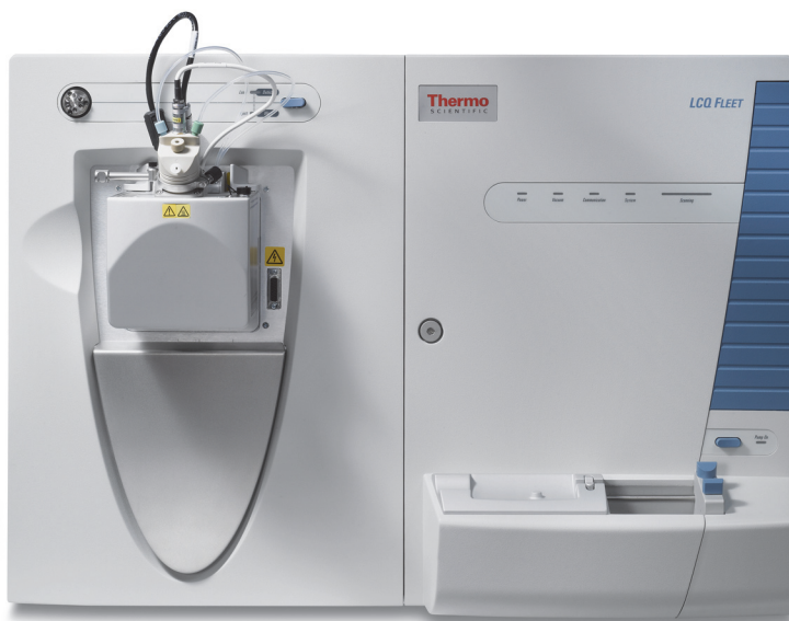
Figure 1. LCQ Fleet MS with the Ion Max-S API source
