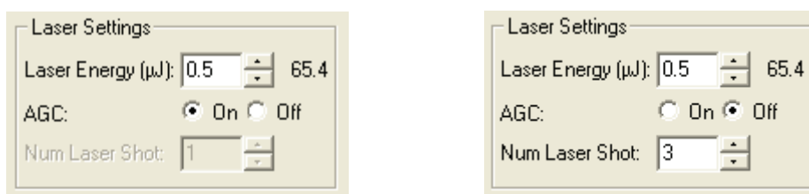
Figure 2. AGC controls on the Control page of the MALDI Source dialog box in Tune Plus
