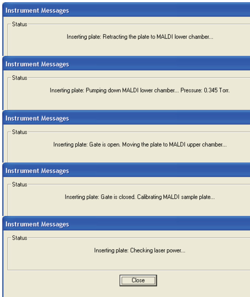
Figure 34. Instrument Messages dialog box during the plate loading process
