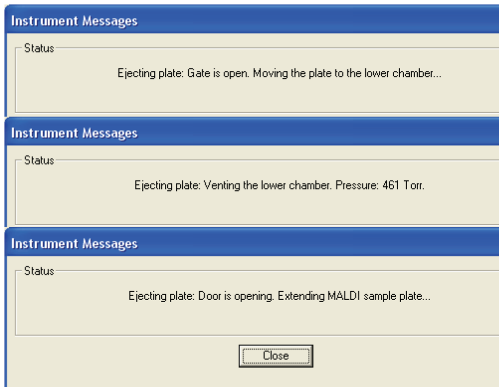
Figure 38. Instrument messages that appear during the ejection process
