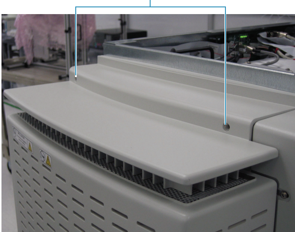
Figure 46. Removing the screws from the optics module cover Optics module cover screws
