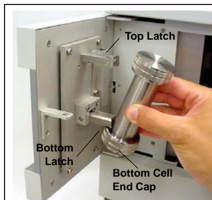
3. Raise the cell so that the bottom end cap lifts the bottom latch.
