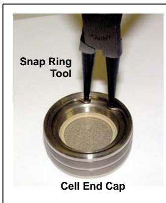
Figure 5-1. Removing the Snap Ring
