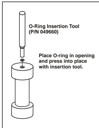
Figure 3-8. Installing a Cell End Cap O-Ring
