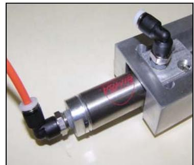
14. Start turning the push screw tool clockwise until the opposite side of the alignment tool touches the back of the cylinder. With the cylinder shaft still extended, fully tighten the valve body mounting screws that you partially tightened in [Step 8](#).
