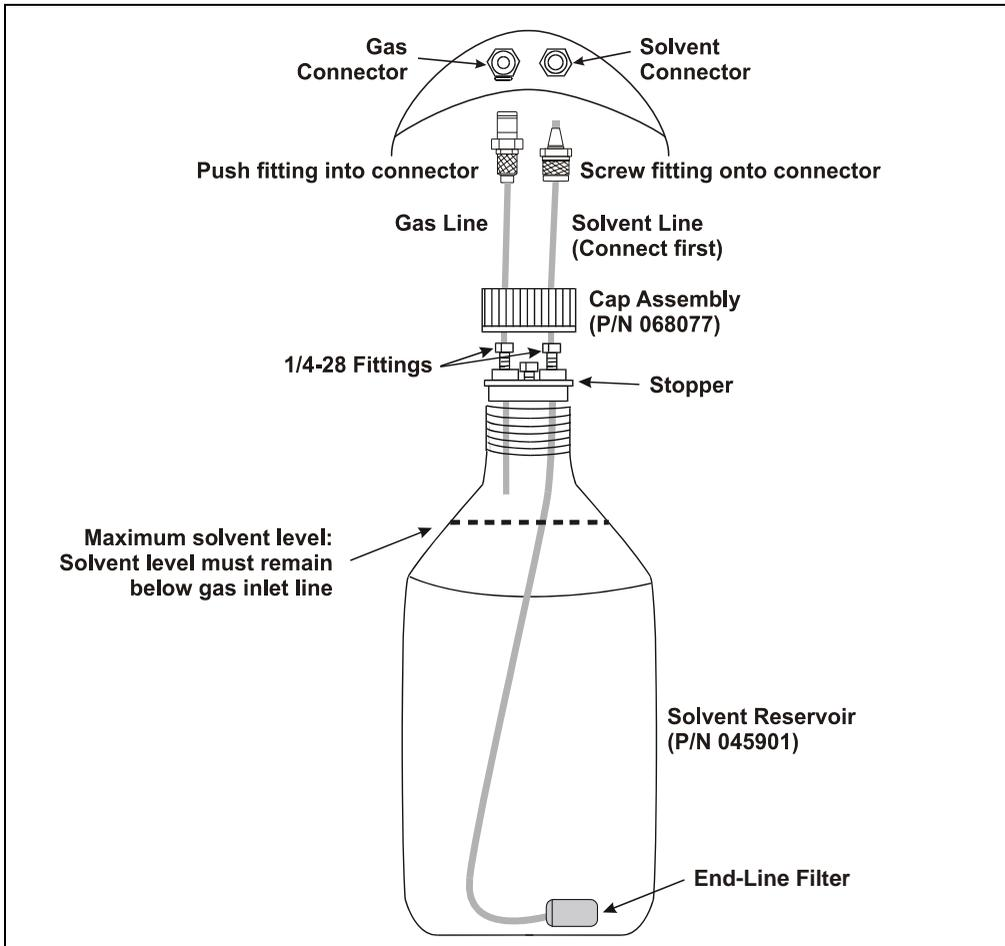
Figure 3-1. Solvent Reservoir Connections
