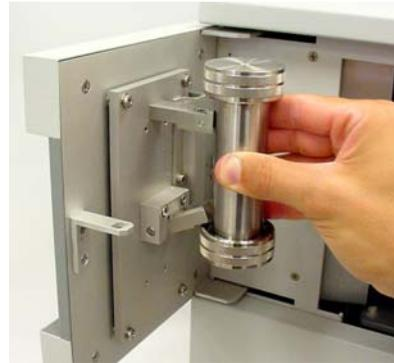
4. Straighten the cell until it is vertical, and then lower it until the top end cap rests on the top latch of the cell holder.
