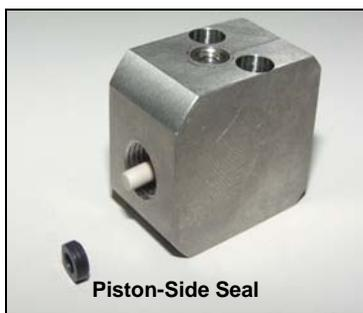
5. Insert the pointed end of the seal removal tool into the valve body. Slide the tool between the valve body and O-ring, and then pull the O-ring out of the valve body.
