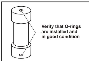
Figure B-9. Inspecting Cell O-Rings
