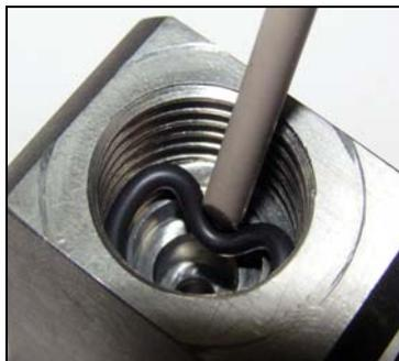
6. Using a cotton-tipped swab (or other tool with a soft tip), thoroughly clean the inside of the valve body. If necessary, moisten the area with IPA (isopropyl alcohol) or acetone to remove all debris, sediment, and precipitates.
