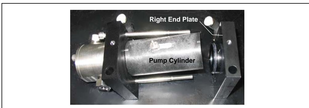
*Figure 5-14. Removing the Pump Right End Plate*
