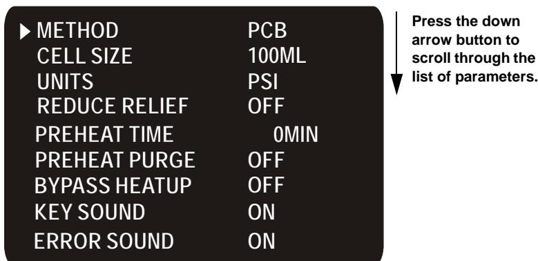
Figure B-8. Setup Screen (All Parameters Shown)
