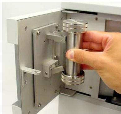
4. Straighten the cell until it is vertical and then lower it until the top end cap rests on the top latch of the cell holder.
