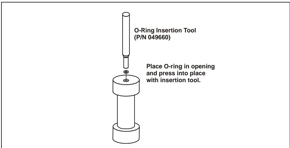
Figure 5-4. Installing the Cell O-Ring
