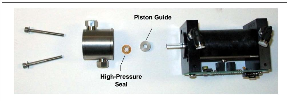
Figure 5-12. Replacing the Dionex ASE 150 Piston High-Pressure Seal
