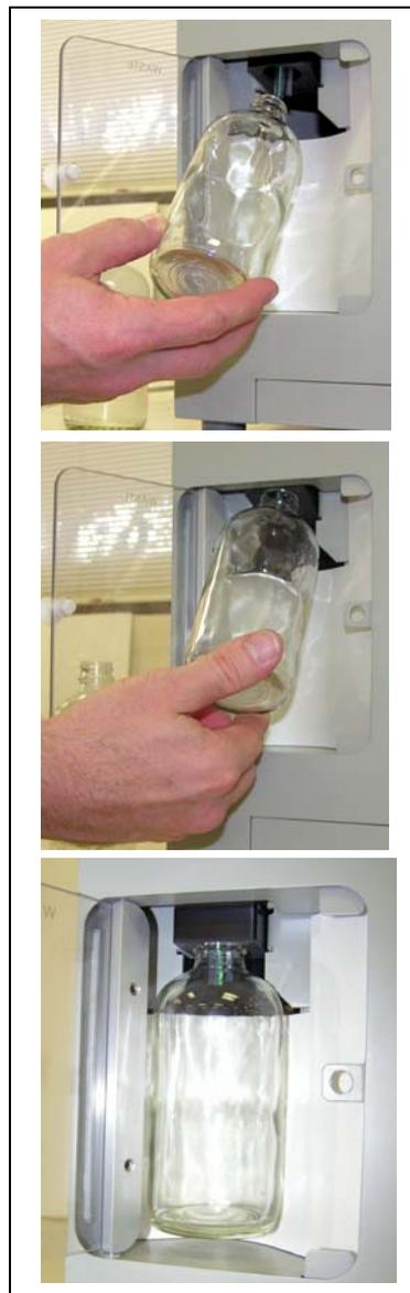
Figure B-5. Installing the Waste Bottle
