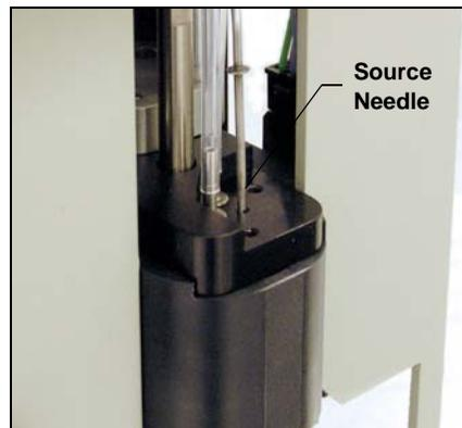
*Figure 5-24. Removing the Source Needle from the Needle Block*
