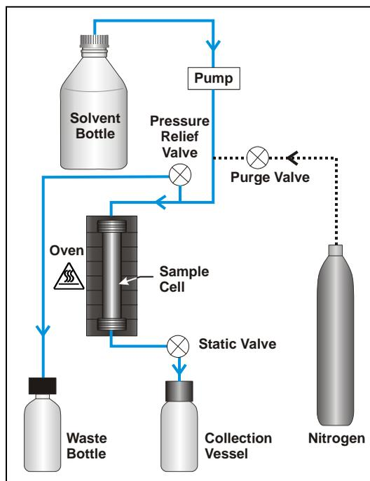
Figure 2-4. Extraction Process Schematic
