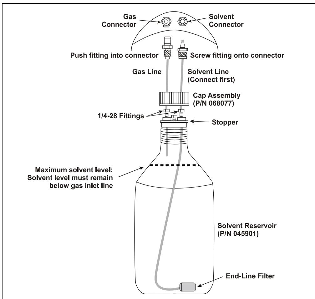
*Figure B-4. Solvent Reservoir Connections (Top View)*
