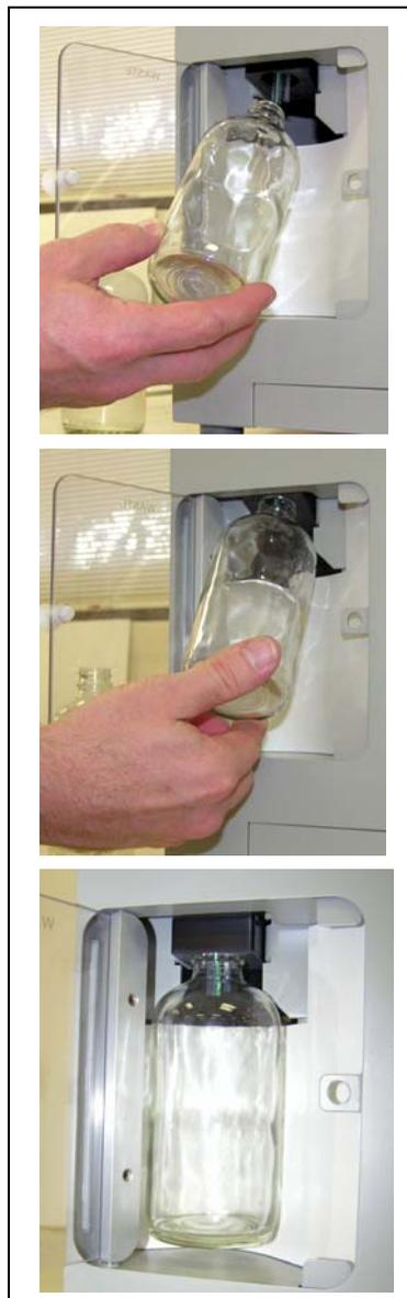
Figure 3-11. Installing the Waste Bottle
