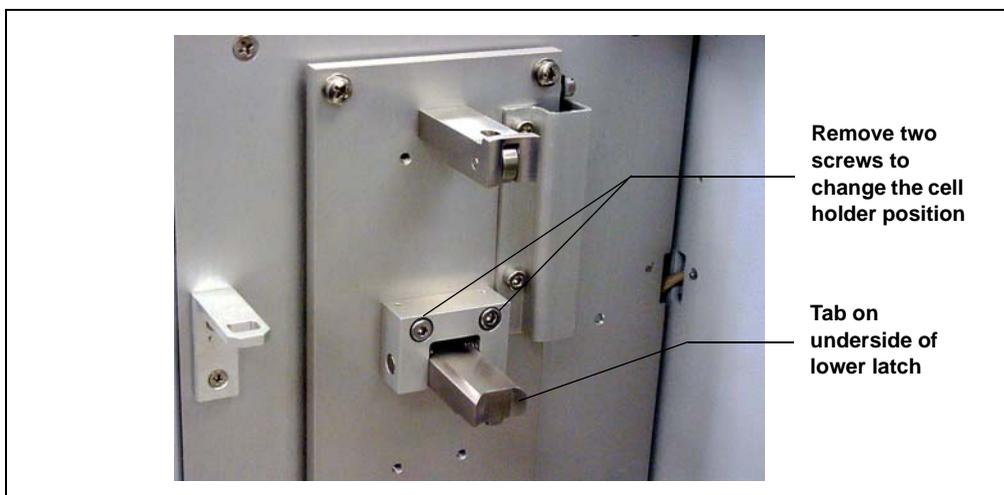
Figure B-6. Removing the Cell Holder Lower Latch
