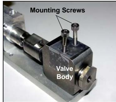
8. Remove the piston from the static valve:
