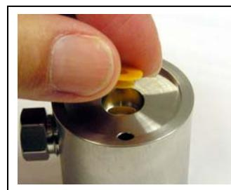
If you had to pry the piston guide out of the pump head ([Step 4](#)), install a new piston guide (P/N 066109) as described above. The original piston guide may have been scratched during removal, so do not use it again. A scratched guide will not seal properly.
