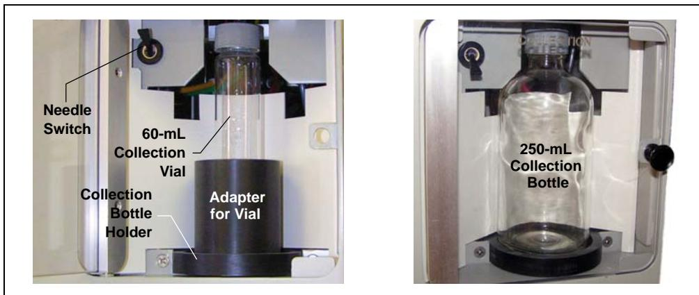
Figure B-12. Installing the Collection Vessel
