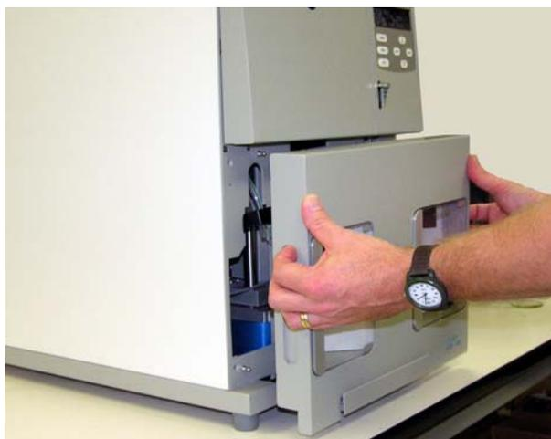
*Figure 5-5. Removing the Lower Front Trim Panel*
