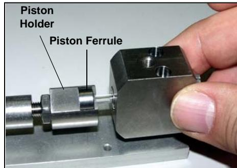
8. Replace the two mounting screws in the valve body and screw them loosely into the valve body to secure the body to the base plate. **Do not fully tighten the screws yet.**
