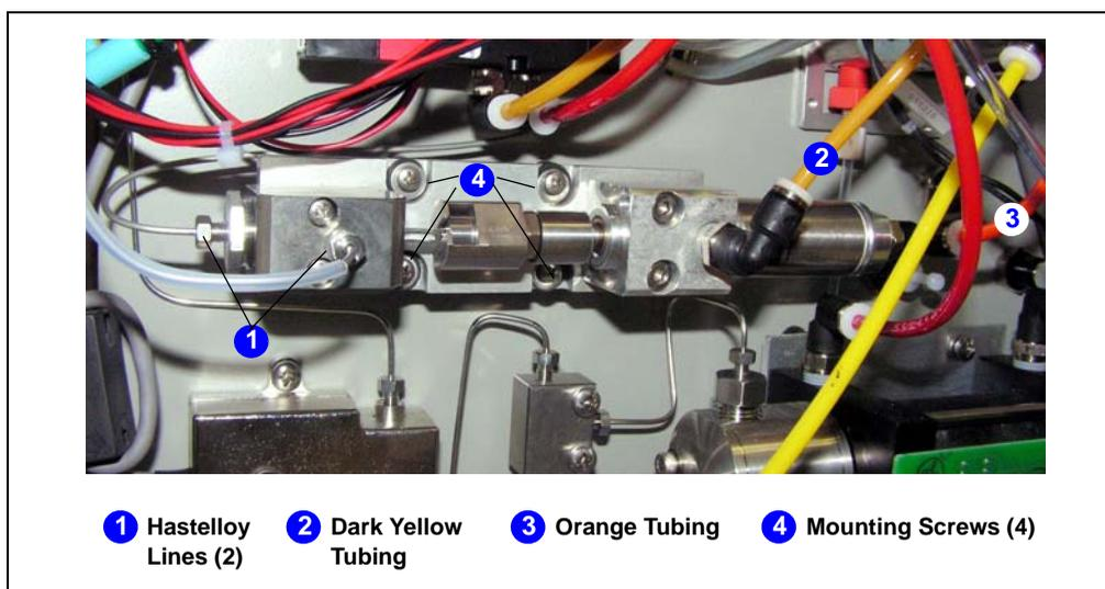
Figure 5-20. Removing the Static Valve
