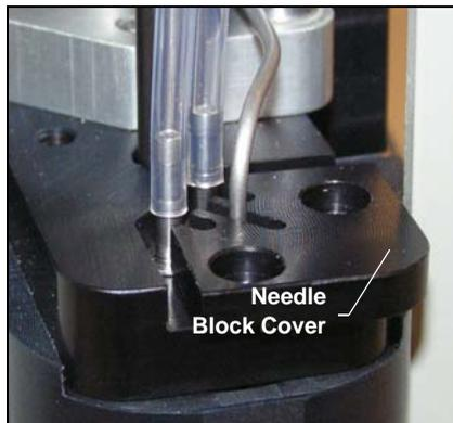
*Figure 5-23. Removing the Needle Block Cover*
