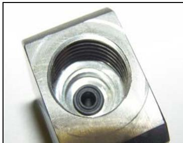
7. Use the inlet-side seal insertion tool (P/N 067395) to press the new seal into place.
