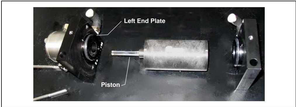
*Figure 5-15. Removing the Pump Left End Plate*
