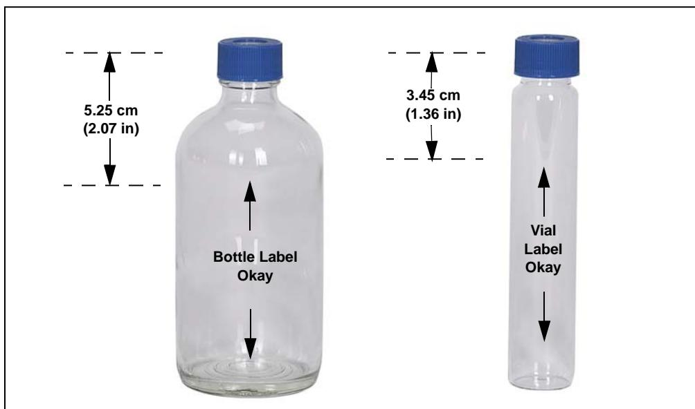
Figure 3-9. Placement of Collection Vessel Labels
