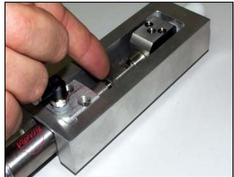
12. Reconnect the gas source and turn on the gas supply. Check the dark yellow and orange lines to see which one is dispensing gas; connect this line to the press fitting on the back of the valve cylinder.
