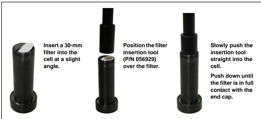
Figure 3-5. Installing a 30-mm Cell Filter in a 34-mL, 66-mL, or 100-mL Cell (Zirconium Cell Shown)
