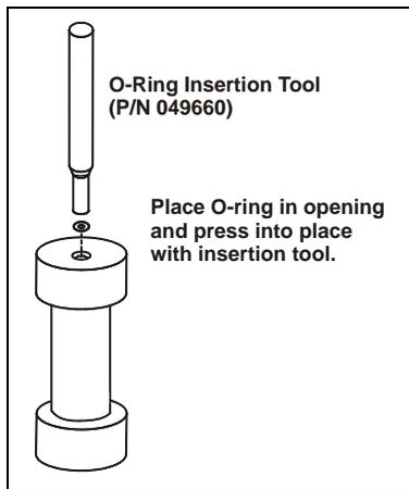
Figure B-10. Installing Cell O-Rings
