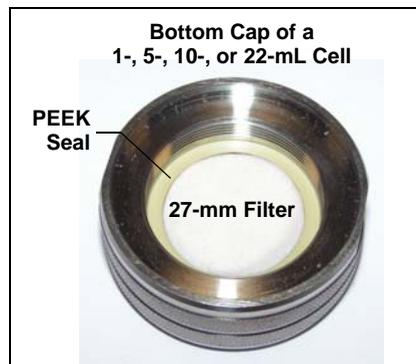
Figure 3-3. Installing a 27-mm Cell Filter
