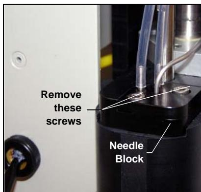
*Figure 5-22. Removing the Needle Block Screws*
