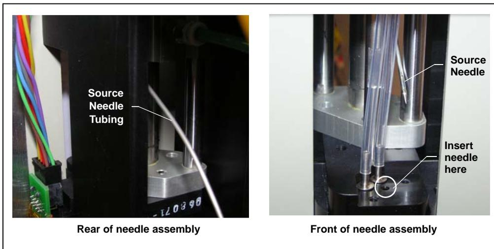
Figure 5-26. Routing the New Source Needle to the Needle Block
