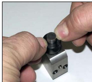
6. Place a new seal (P/N 066165), with the O-ring side facing up, into the inlet gland (large opening) of the valve body.
