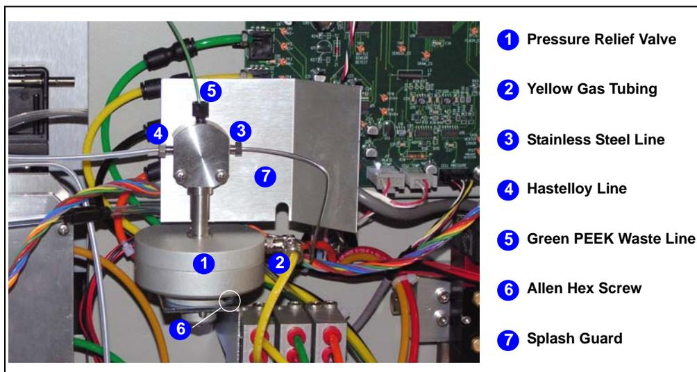
Figure 5-18. Connections to the Pressure Relief Valve
