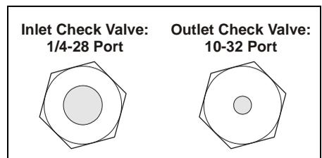
Figure 5-9. Check Valve Housings
