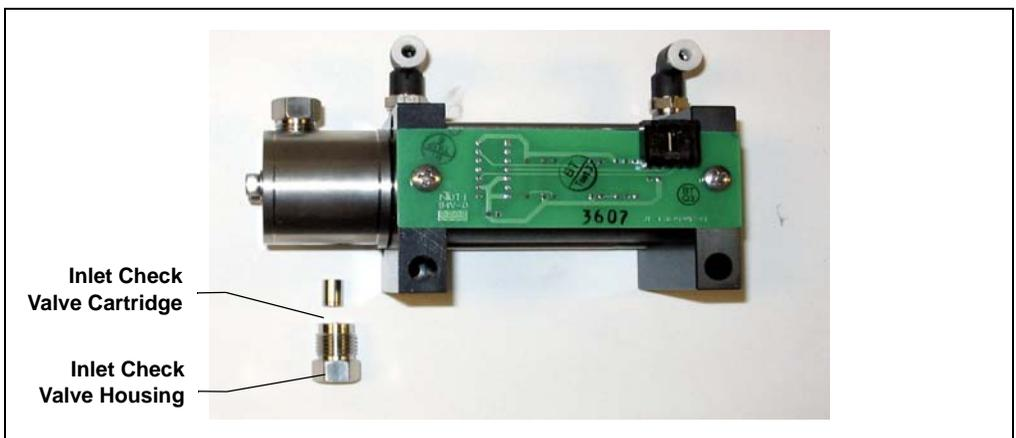
Figure 5-8. Disassembled Dionex ASE 150 Pump Inlet Check Valve
