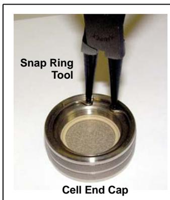
Figure 5-1. Removing the Snap Ring
