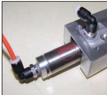
14. Start turning the push screw tool clockwise until the opposite side of the alignment tool touches the back of the cylinder. With the cylinder shaft still extended, fully tighten the valve body mounting screws that you partially tightened in [Step 8](#).
