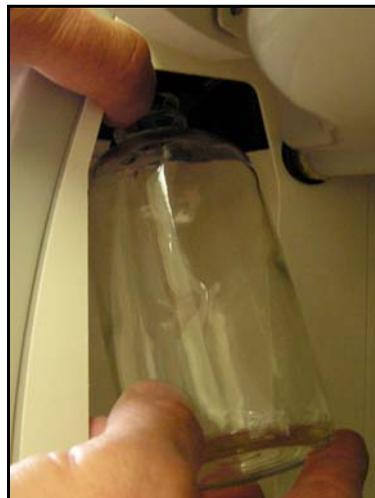
*Figure B-9. Installing the Waste Bottle*
