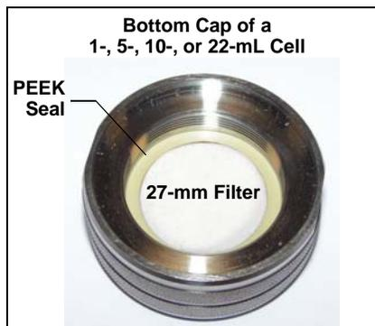
Figure 3-4. Installing a 27-mm Cell Filter
