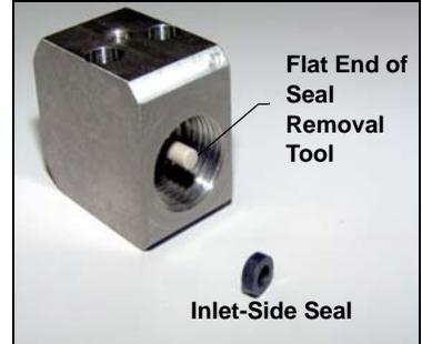
5. Pull the seal removal tool out of the valve body.
