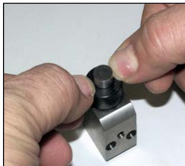
**NOTE:** If there is no audible snap, check the seal for damage. An undamaged seal will lie completely flat in the valve body, with no visible edges. If the seal is damaged, remove it from the valve body and order a replacement seal.
