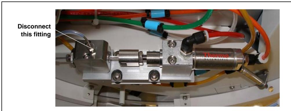
Figure 5-27. Disconnecting the Source Needle Fitting from the Static Valve
