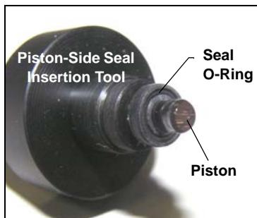
5. Rest your thumbs on the back of the tool and press down firmly (with equal pressure) on both the left and right sides of the tool. You should hear a snap as the new seal is seated in the valve body. Remove the piston and the tool from the valve body.
