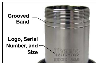
Figure 3-5. Sample Cell Top (Larger Cells)
