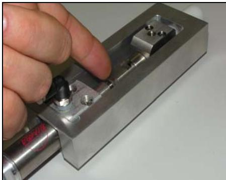
12. Reconnect the gas source and turn on the gas supply. Check the red and orange lines to see which one is dispensing gas; connect this line to the press fitting on the back of the valve cylinder.
