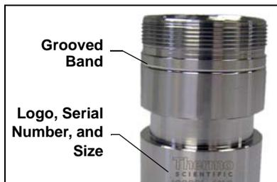
Figure 3-3. Sample Cell Orientation (Smaller Cells)
