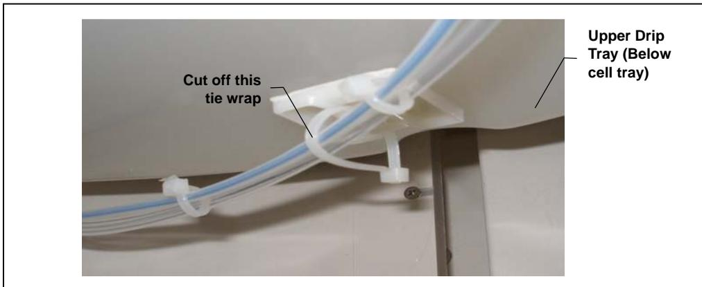
*Figure 5-20. Tie Wrap Removal*
