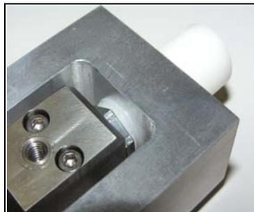
15. Turn the push screw tool counterclockwise. Remove the alignment tool from the valve.
