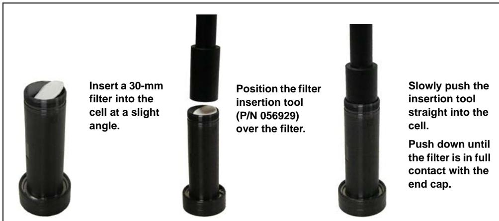
Figure 3-6. Installing a 30-mm Cell Filter in a 34-mL, 66-mL, or 100-mL Cell (Zirconium Cell Shown)
