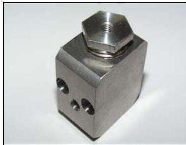
5. Reinstall the nut on the piston side of the valve body and tighten with a flathead screwdriver.
