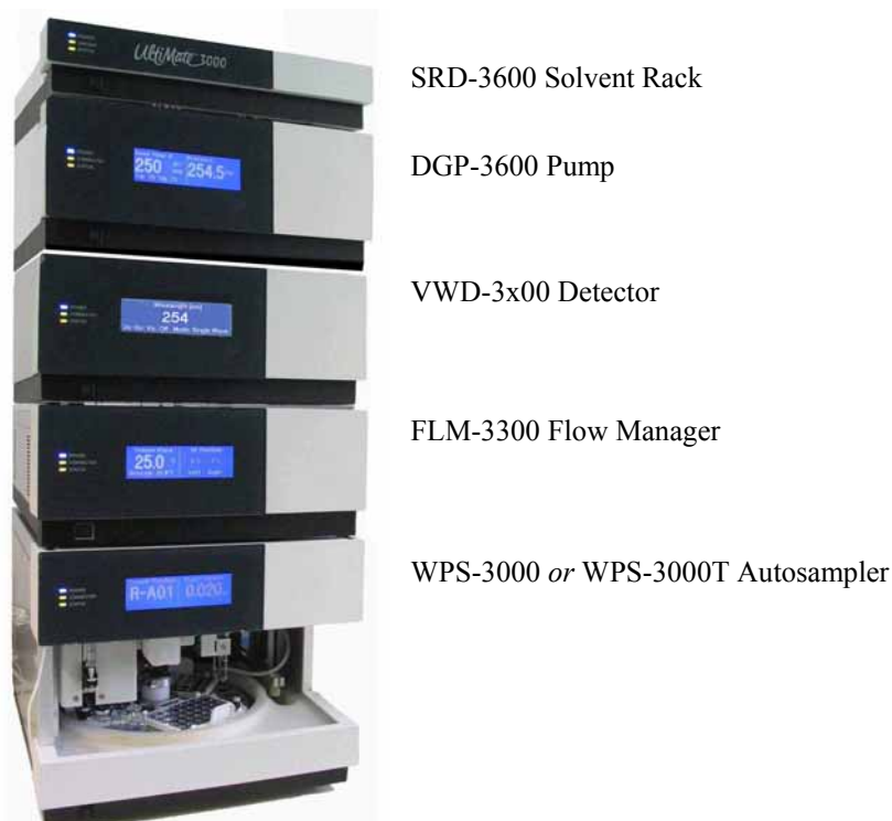
Fig. 11: Module arrangement for preconcentration
