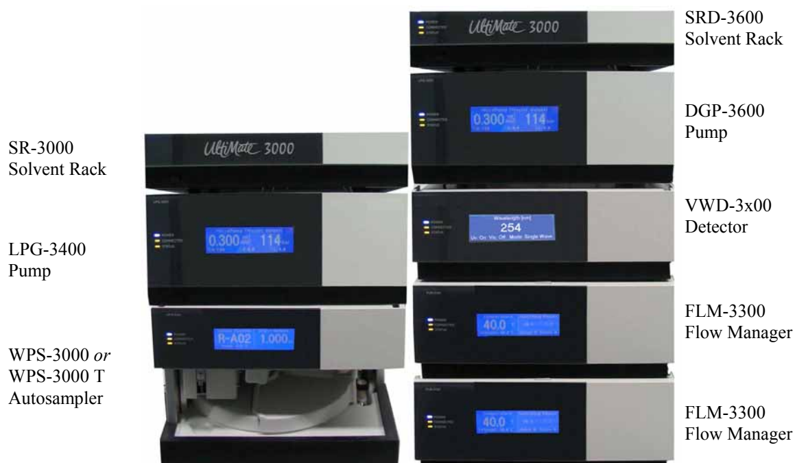
Fig. 17: Module arrangement for comprehensive 2D LC
