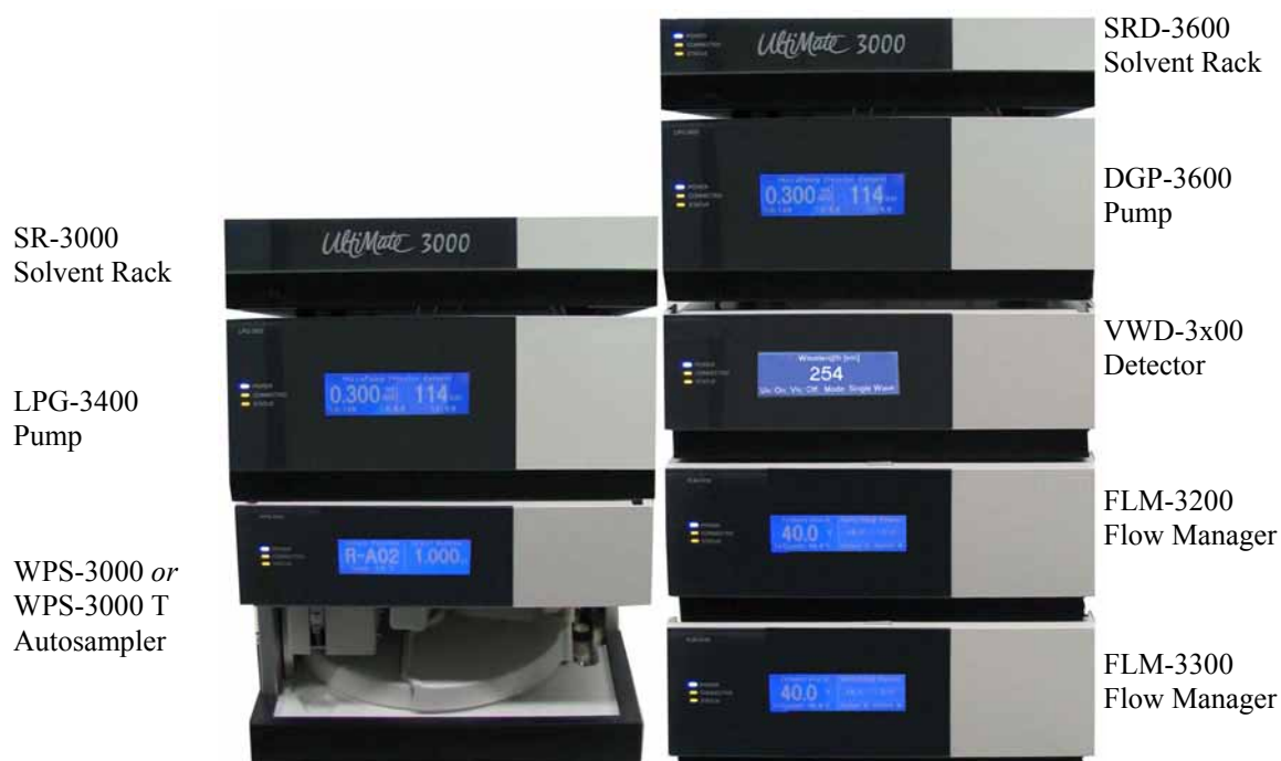
Fig. 20: Module arrangement for parallel LC
