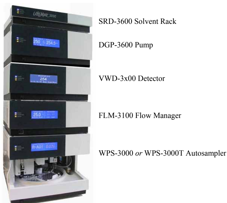
Fig. 14: Module arrangement for 2D LC salt plug
