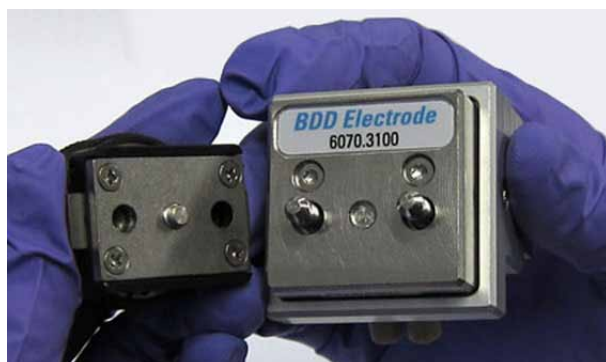
Fig. 42: Holding the side tabs and installing the torque knob
