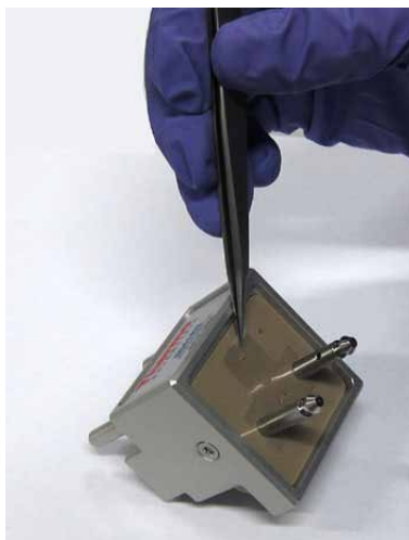
Fig. 39: Installing the gasket
