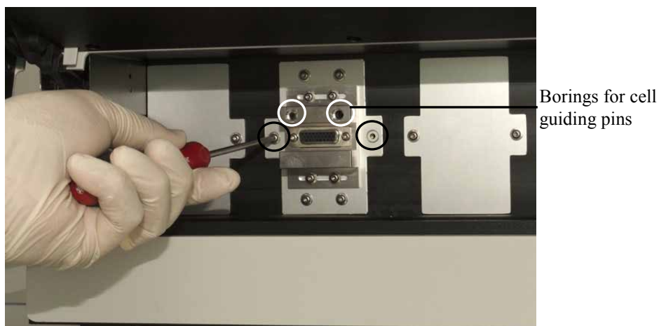
Fig. 33: Tightening the attachment screws
