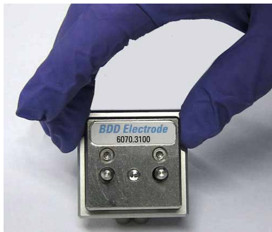
Fig. 41: Installing the working electrode (here: Boron-doped diamond electrode)
