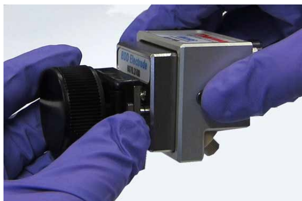
Fig. 38: Removing torque knob from the cell
