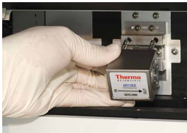
Fig. 35: Installing the coulometric cell to the potentiostat module
