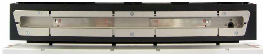
Fig. 21: View into the column compartment
