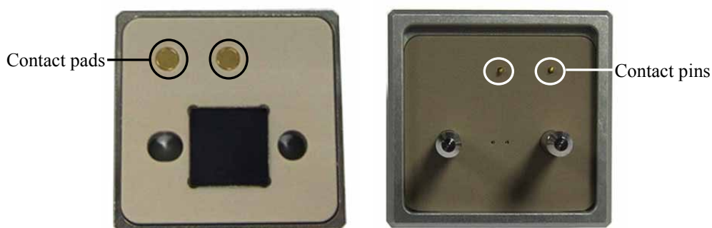
Fig. 40: Left: Contact pads on a BDD working electrode Right: Contact pins on the cell body
