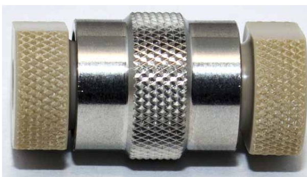
Fig. 44: Filter holder with lock nuts installed
