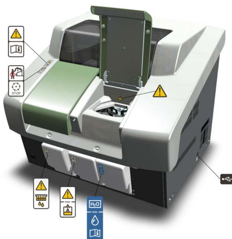
Figure 1. Safety labeling outside analyzer
