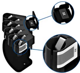
Figure 13. Barcode label, rack ID label and infolabel on 18-position sample rack for tubes (ID numbers 451 - 499)
