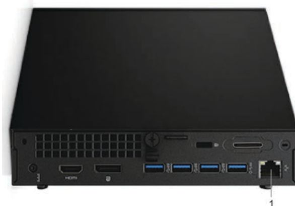
1 - Ethernet port for network connection
