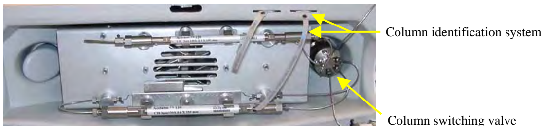
Fig. 23: TCC-100 with column switching valve(here: 2-position/6-port) and 2 columns (here: with column identification system for both columns)
