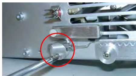
Fig. 14: Holders (top parts) for the eluent preconditioners
