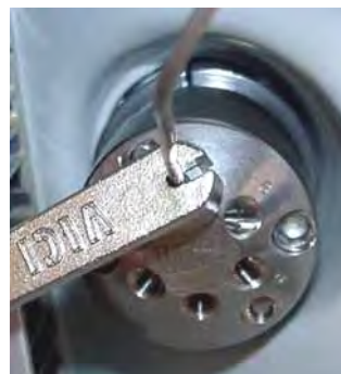
Fig. 25: Connecting the capillaries
