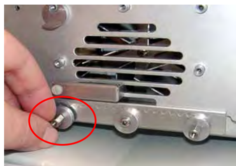
Fig. 20: Tightening the retaining screws (2)
