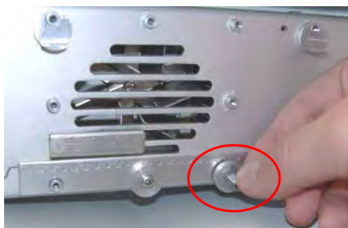
Fig. 20: Tightening the retaining screws (2)
