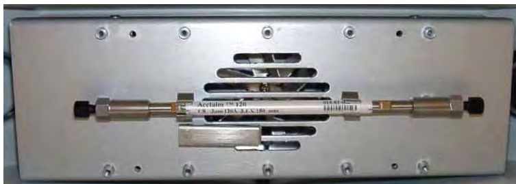
Fig. 9: Column in column clip
