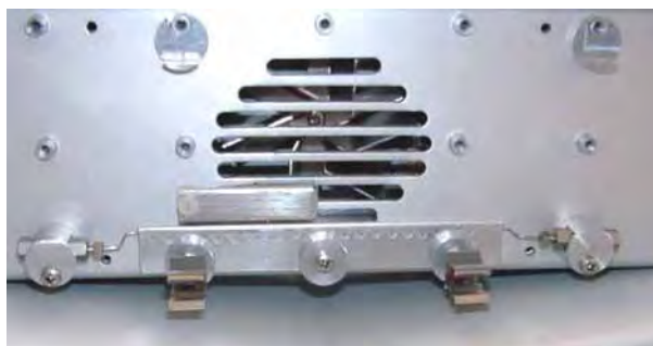
Fig. 22: Eluent preconditioner with column clips
