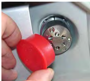
Fig. 24: Removing the plastic cap
