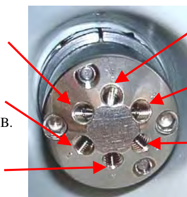
Fig. 26: Typical example for the connections on a 2-position/6-port column switching valve
