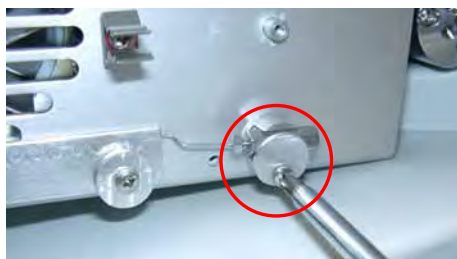
Fig. 14: Holders (top parts) for the eluent preconditioners
