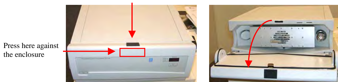
Fig. 7: Tilting the front panel downward
