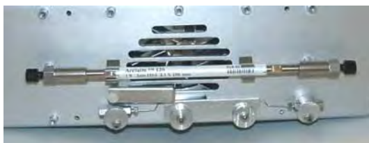
Fig. 16: Column and eluent preconditioner installed
