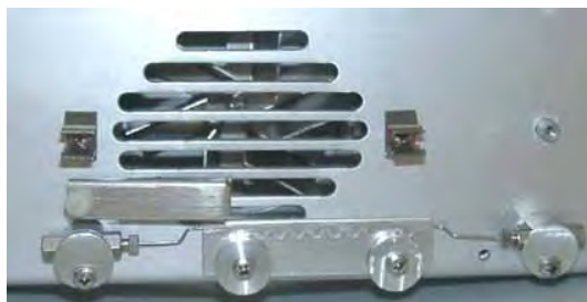
Fig. 15: Installed eluent preconditioner
