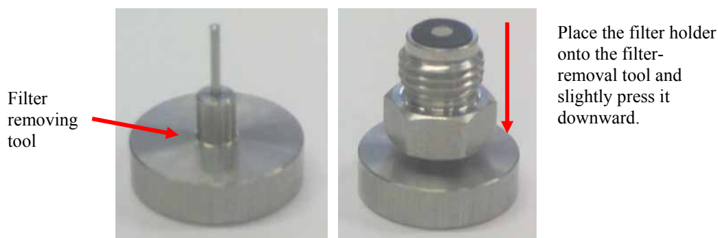
Fig. 43: Removing the inline filter
