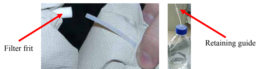
Fig. 8: Connecting the solvent lines to the reservoir
