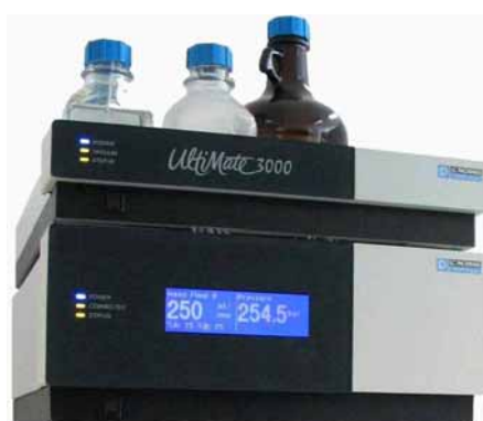
Fig. 7: Pump with solvent rack
