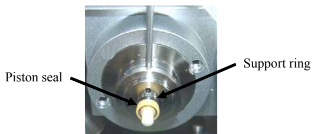
Fig. 54: Piston seal on pump head bushing of the rear-seal wash system
