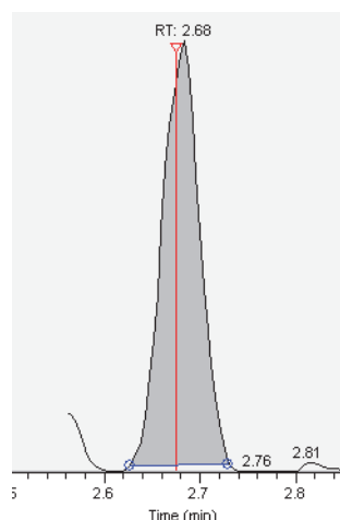
Figure 51. Integrated alprazolam peak
