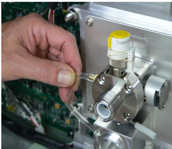
Figure 3-29. Removing the foreline hose from its connection
