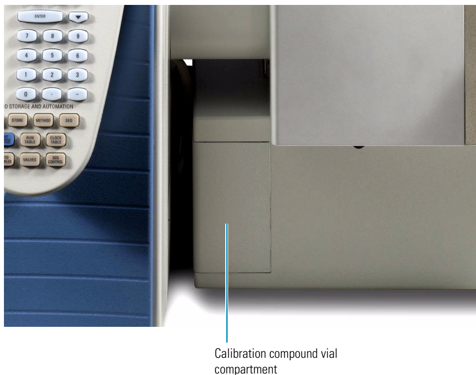
Figure 64. Location of the calibration compound vial compartment
