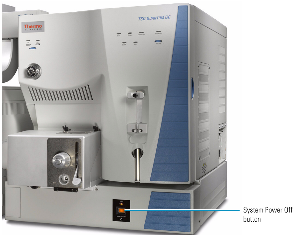
Figure 29. System Power Off button on the front of the electronics module
