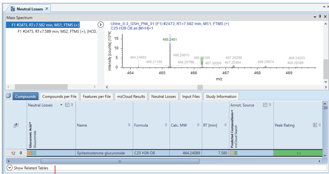
Figure 22. Result file from a processing workflow with the Search Neutral Losses node (with column fixing enabled and a compound pinned to the top of the table))
