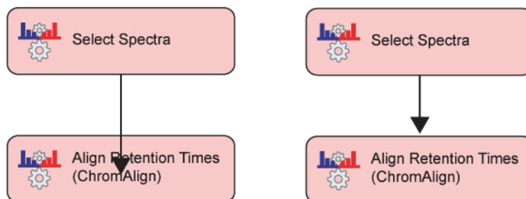
Figure 80. Connecting the Select Spectra node to the Align Retention Times node (LC study)
