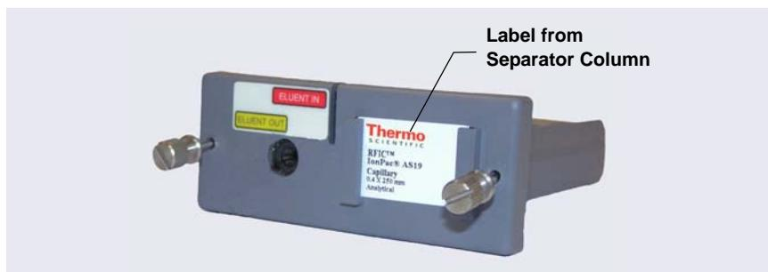
**Figure 4-9.** Capillary Column Tray with Column Label
