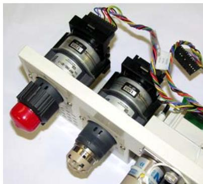
**Figure B-25.** High-Pressure Valve Installation
