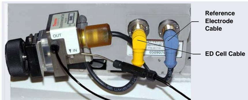
**Figure B-14.** ED Cell Installed on ED
