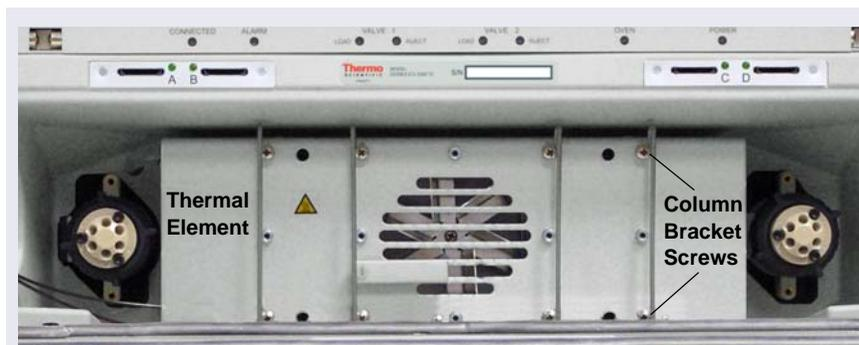
**Figure 3-9.** TC Column Bracket Positions
