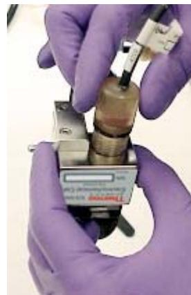
**Figure B-12.** Installing the pH-Ag/AgCl Reference Electrode In the Reference Electrode Well
