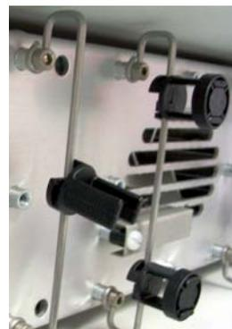
**Figure 3-12.** Column Clips Installed
