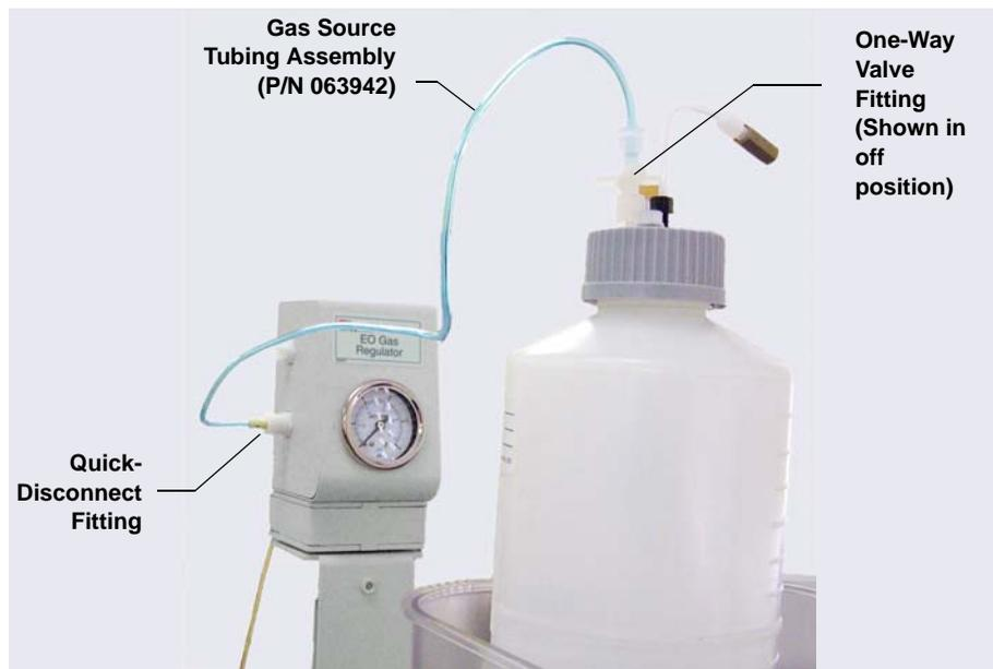
**Figure A-3.** Gas Connections to Reservoir
