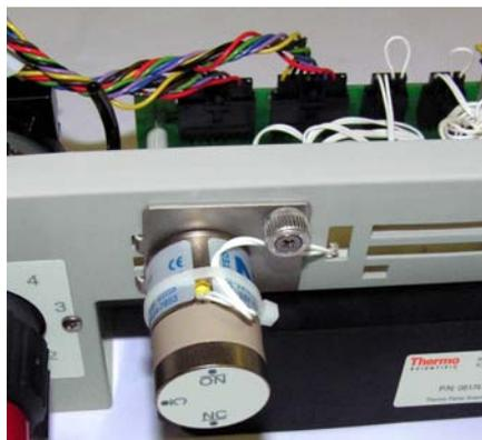
**Figure B-27.** *Low-Pressure Valve Installation (Left Valve Mounting Position)*
