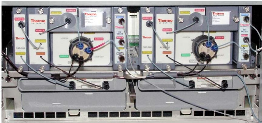
**Figure 4-19.** Completed IC Cube Plumbing for a Dual Conductivity Detection System
