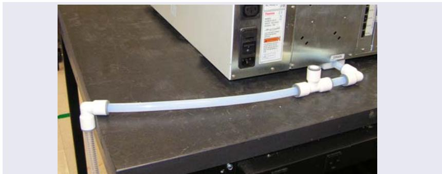
**Figure 3-31.** *Drain Line Routed to Side of Bench*
