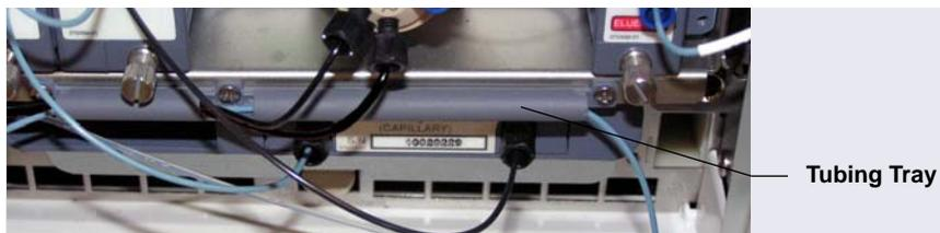
**Figure 4-18.** IC Cube Tubing Trays (System #2 of Dual System Shown)
