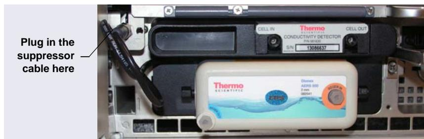
**Figure 3-8.** *Installing the Suppressor (Left-Side Installation)*
