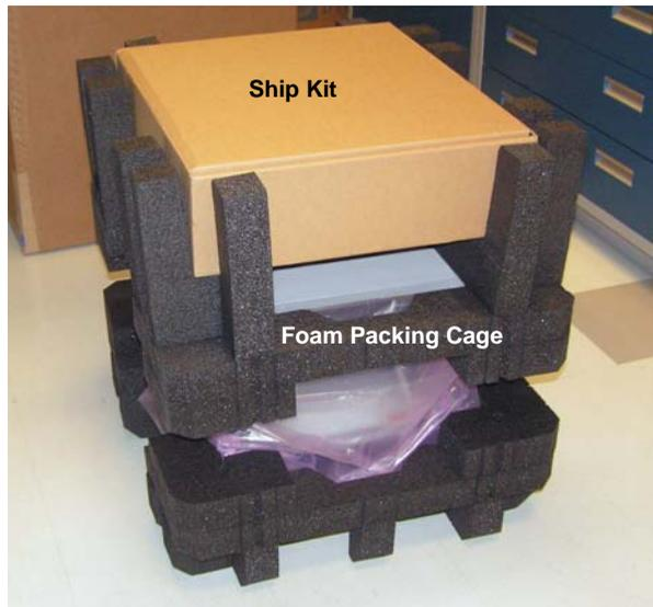
**Figure 2-3.** Ship Kit on top of the module
