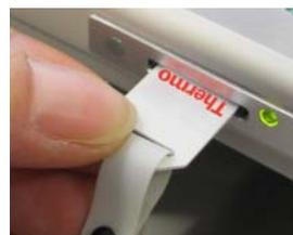
**Figure 3-14.** Inserting a Column ID Chip Card
