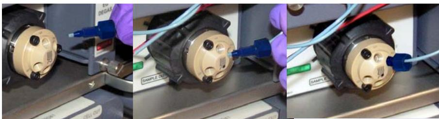
**Figure 1-3.** Ferrule and Fitting Bolt Placement for Tubing Connections
