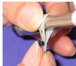
**Figure 3-13.** Attaching the Column ID System to the Column
