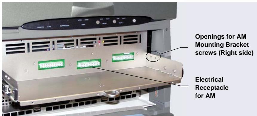
*Figure B-28. DC with Top Component Tray Pulled Forward*
