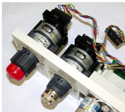
Figure B-23. High-Pressure Valve Installation
