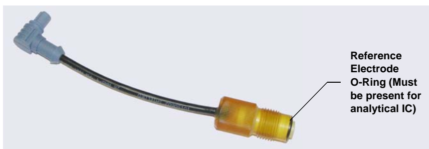
Figure B-12. pH-Ag/AgCl Reference Electrode O-Ring
