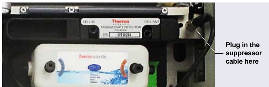
Figure 3-8. Installing the Suppressor (Right-Side Installation)
