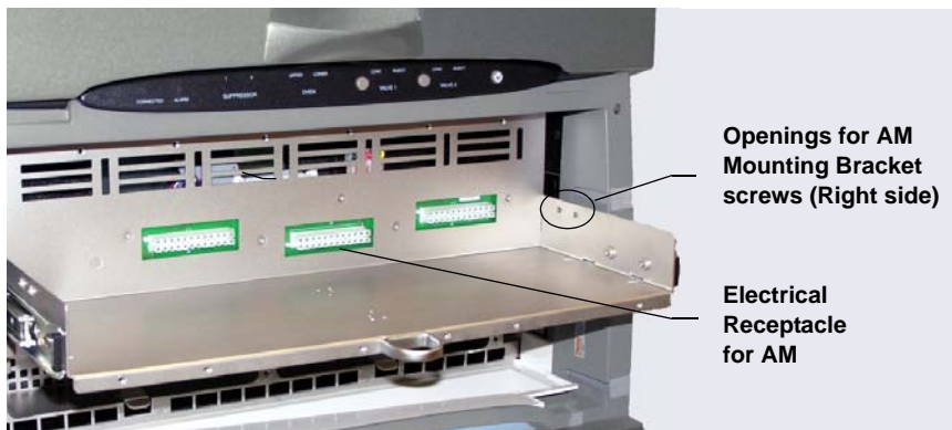
Figure B-26. DC with Top Component Tray Pulled Forward
