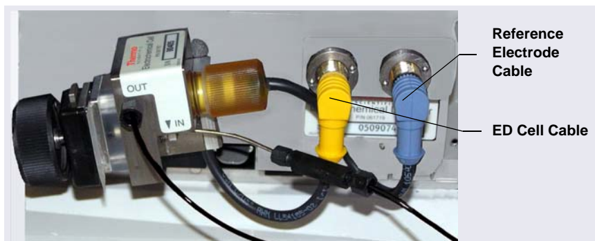
Figure B-13. ED Cell Installed on ED
