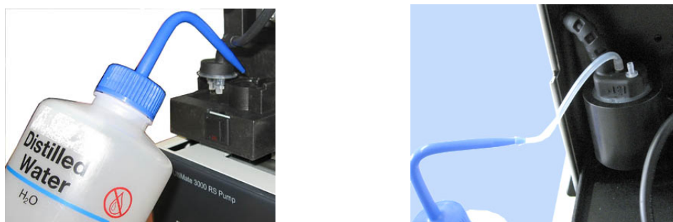
Fig. 10: Filling liquid into the seal wash system (examples) (left: RS, SD, and BM pumps; right: NCS-3x00RS)
