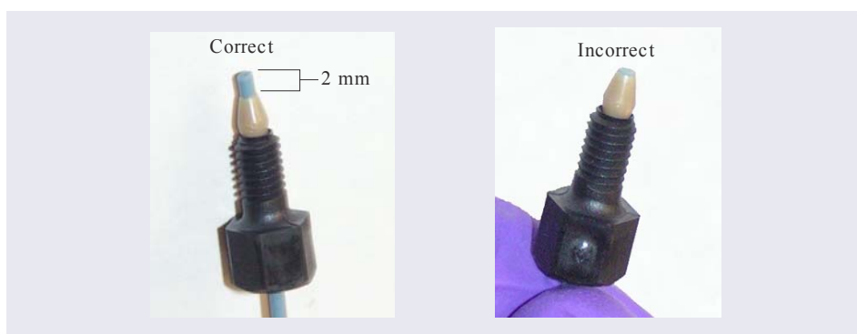
Figure 17 Correct and Incorrect Ferrule and Fitting Bolt Placement for Capillary Tubing Connections
