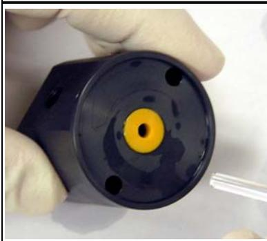
7. Verify that the O-ring is installed in the spacer.
