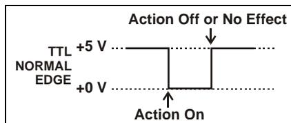
The action of the positive (rising) edge depends on the function. For example, for the **Load/Inject** function, the positive edge switches the injection valve to the Inject position. For the **Pump On/Off** function, the positive edge turns off the pump. For the **Autozero** function, the positive edge has no effect.
