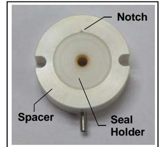
4. To install the new backup piston seal:
