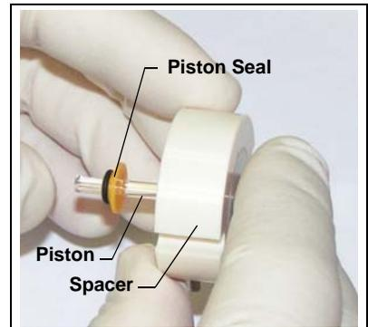
4. Insert the piston and seal into the pump head.
