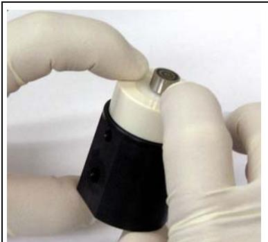
6. Remove the spacer and piston and verify that the seal is flush with the surface of the pump head.
