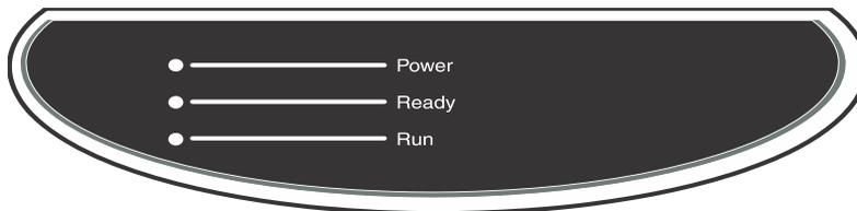
Three status LEDs (described below) are on the Dionex Easion front door.
