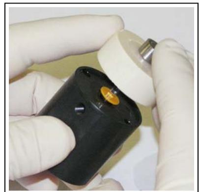
5. To seat the seal, push down on the spacer until it is flush with the pump head. A clicking sound indicates that the seal is correctly seated.
