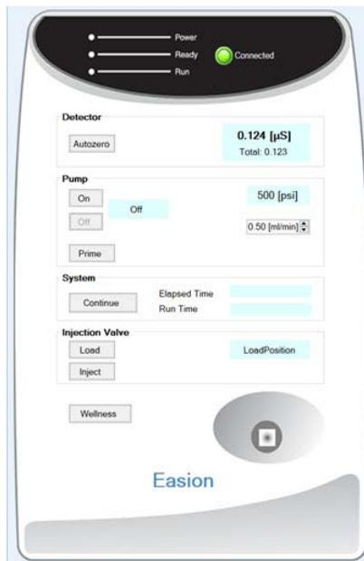
Figure 2-10. Dionex Easion: Chromeleon ePanel Status and Control Functions
