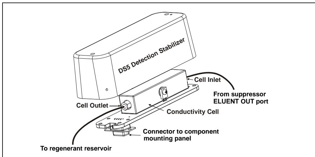
Figure 2-9. Conductivity Cell and Dionex DS5 Detection Stabilizer
