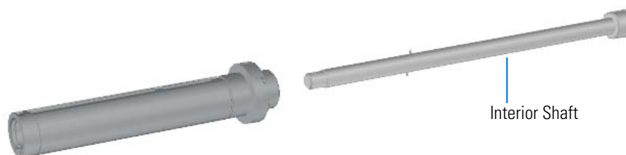
Figure 197. Reinserting the Interior Shaft
