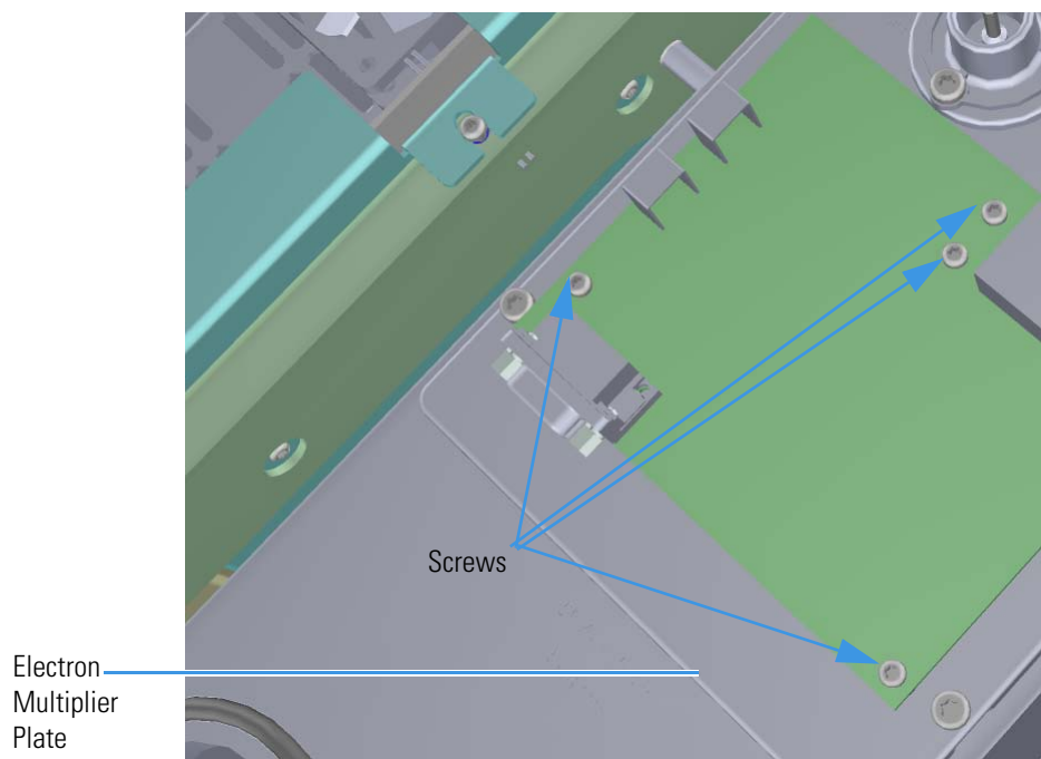
Figure 259. Removing the Electrometer Board
