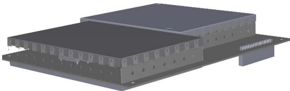
Figure 291. Replacing the Rod Driver Board
