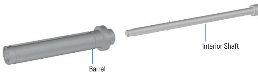
Figure 194. Removing the Interior Shaft
