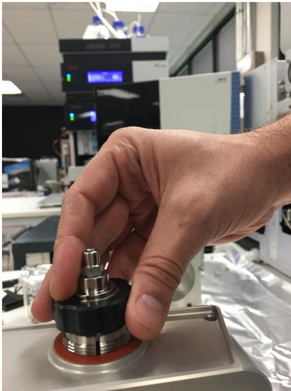
*Figure 98: Removal of APCI probe assembly*
