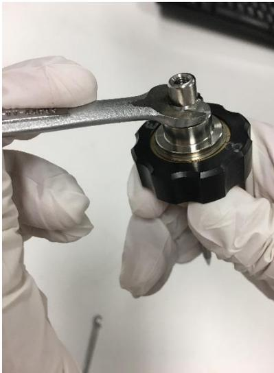
*Figure 99: Loosening the nut on the APCI probe*
