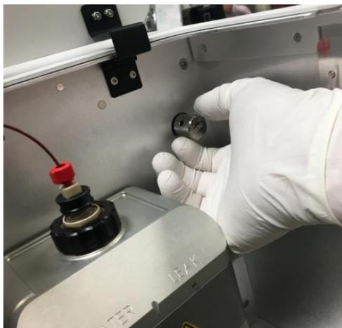
*Figure 90: Venting the mass spectrometer*
