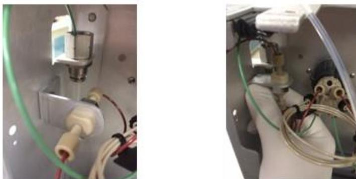
Figure 55: LC to MS inlet assembly
