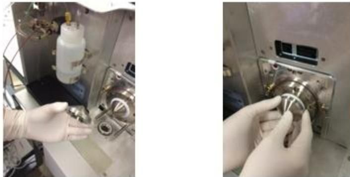
Figure 47: Installation of sweep cone
