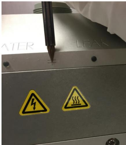
*Figure 94: Capillary assembly alignment marks on source housing*
