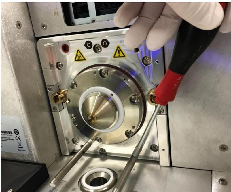
Figure 122: Tightening spray chamber pins
