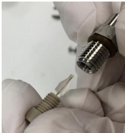
*Figure 102: Removing the clear ferrule and PEEK capillary*
