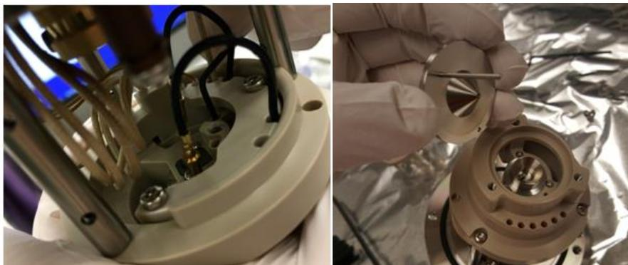
Figure 119: Removing the Skimmer Cone
