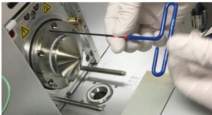
Figure 108: Screwing in the set screws
