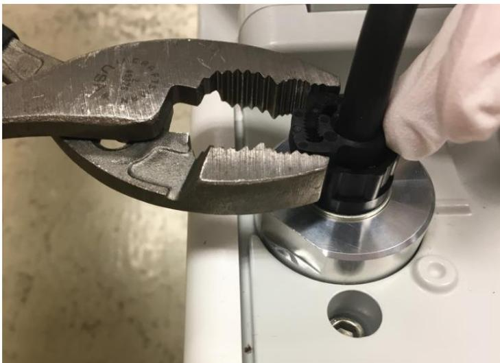
*Figure 19: Tightening the clamp with a tool*
