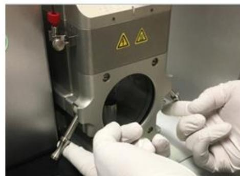
Figure 45: Removal of source housing
