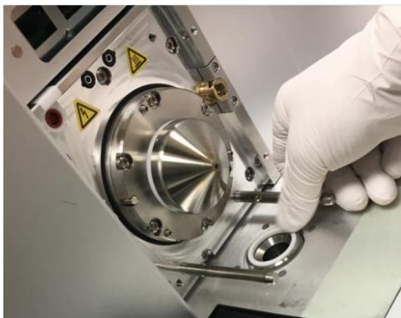
*Figure 48: Reinstalling the Source Housing*
