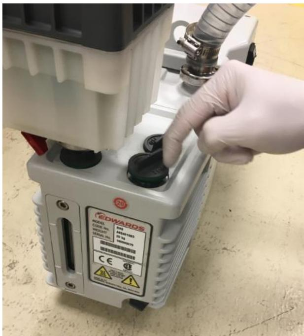
Figure 38: Unscrewing the oil reservoir cap
