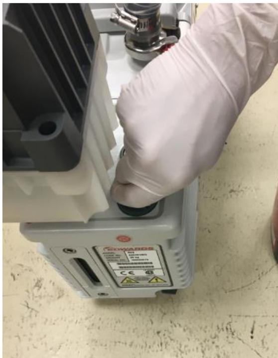
Figure 40: Closing and tightening the oil reservoir cap
