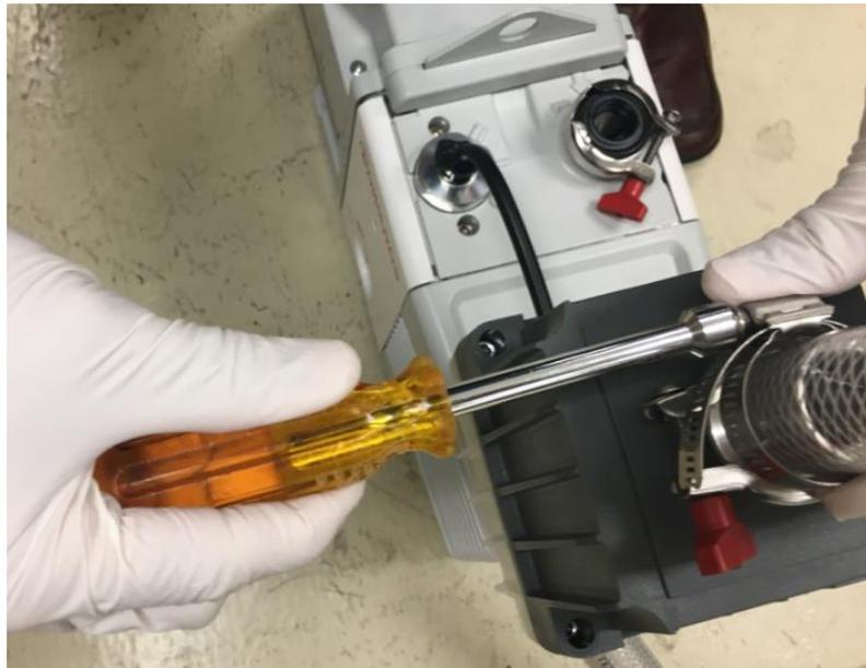
*Figure 35: Tightening the clamp with a nut driver*
