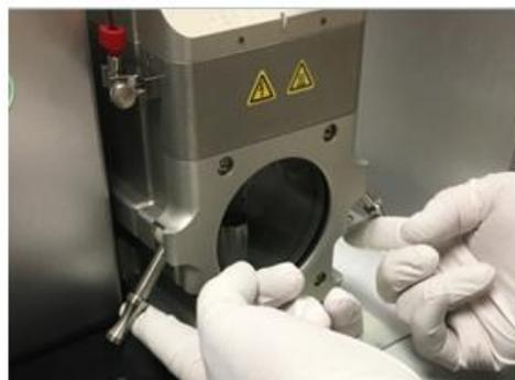
Figure 43: Removal of the source housing
