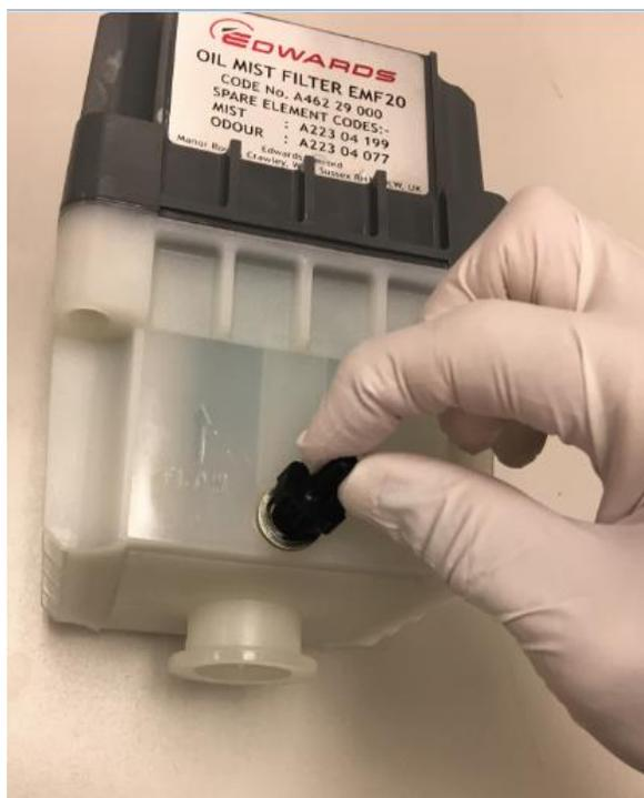
Figure 23: Installing the skinny hose adapter
