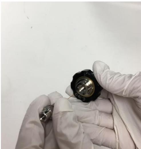
Figure 103: Threading capillary assembly into APCI probe
