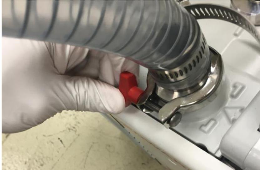
*Figure 21: Installing the clamp for the exhaust hose*
