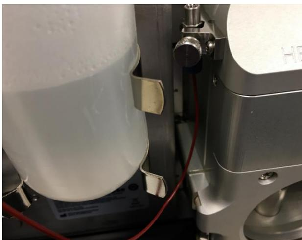
*Figure 49: Reattaching the PEEK tubing to the grounding union*
