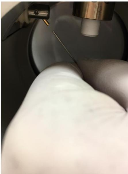
*Figure 106: Removing and reinstalling the APCI needle*
