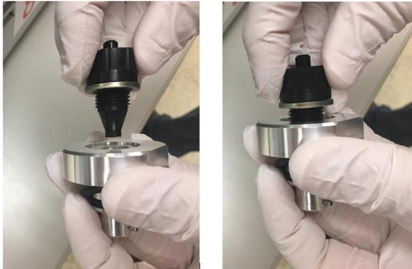
*Figure 10: Screwing the adapters together*
