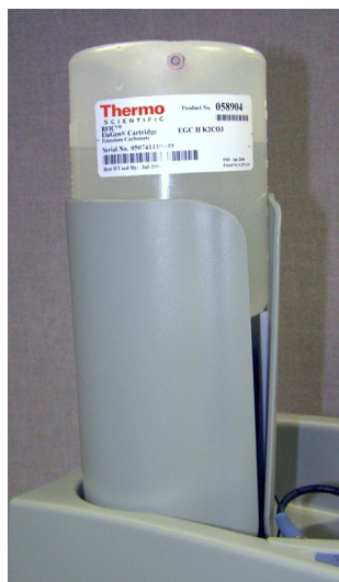
Figure 62. Dionex EGC installed in the holder
