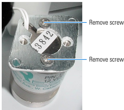
Figure 41. Removing the eluent valve mounting plate
