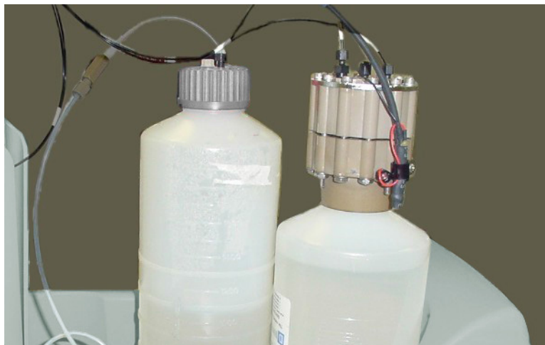
Figure 49. Dionex EGC in the service area
