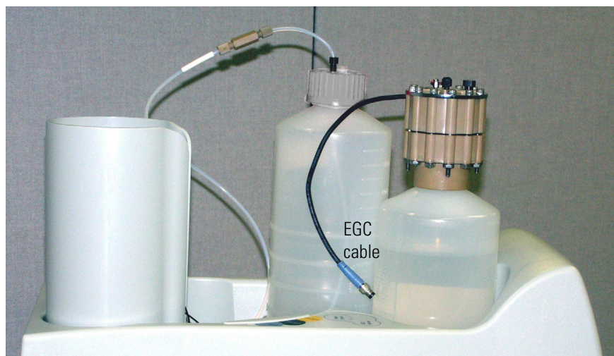
Figure 61. Dionex EGC in the service area
