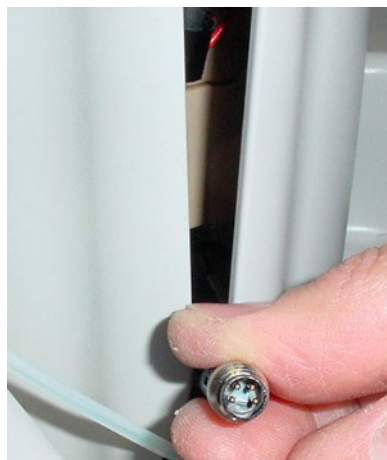
Figure 63. Connecting the Dionex EGC electrical cable
