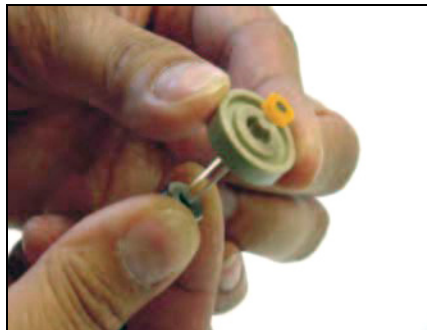
Figure 32. Removing the piston rinse seal from the seal guide
