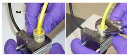
Figure 10-76. Installing the PdH Reference Electrode Nut
