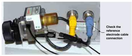
Figure 9-8. ED Cell Electrical Connections
