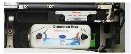
5. Unplug the suppressor cable from the detector.
