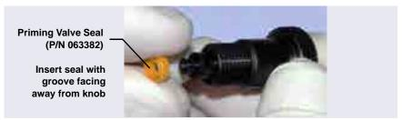
Figure 10-13. Replacing the Priming Valve Seal
