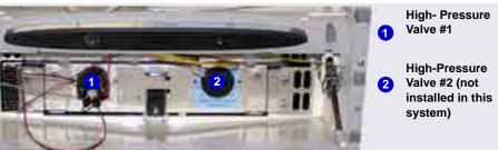
Figure 9-5. High-Pressure Valves #1 and #2 (in DC Lower Compartment)
