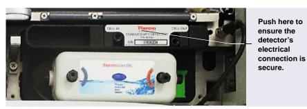
Figure 9-3. Conductivity Detector Connection
