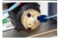
Follow these guidelines when tightening a high-pressure 10-32 fitting bolt (P/N 22000-98001) and high-pressure 10-32 double-cone ferrule (P/N 043276):
