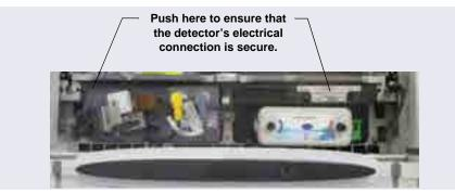
Figure 9-1. Detector Connection
