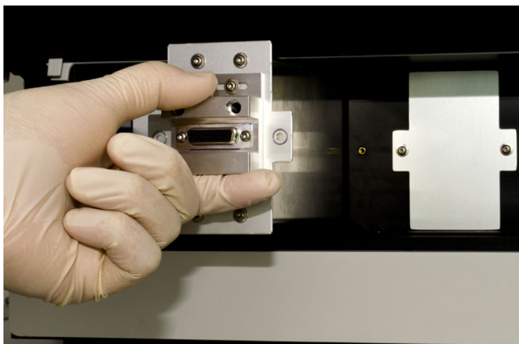
Fig. 30: Pulling out the potentiostat module (here: Bay B)
