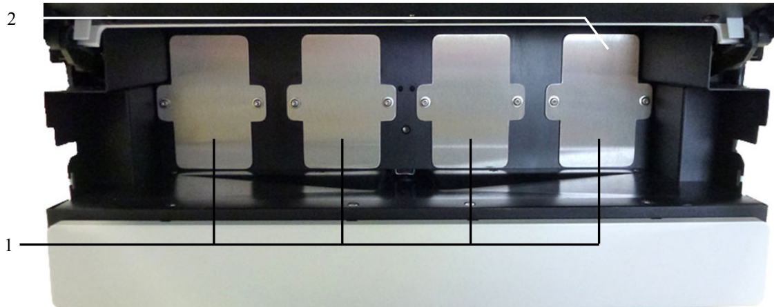
Fig. 5: Bays in the detector
