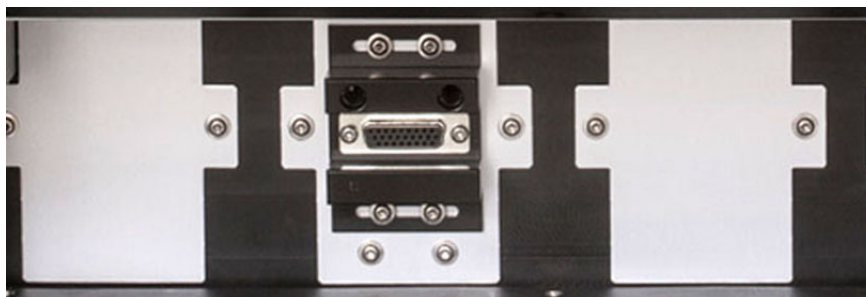
Fig. 14: Potentiostat module installed
