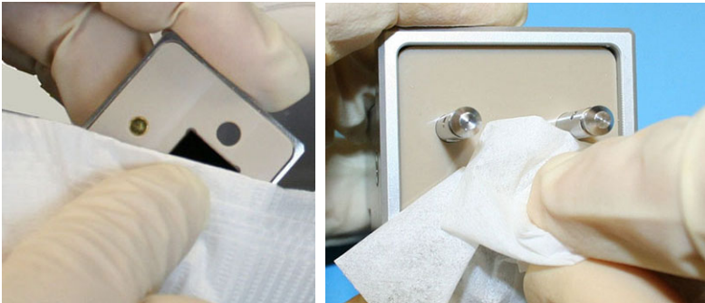
Fig. 14: Drying the components (left: drying working electrode; right: drying cell body)
