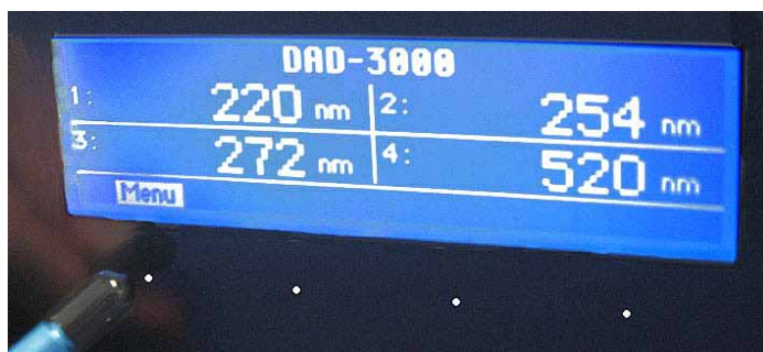
Fig. 19: Showing the function keys (here: under Chromeleon control)
