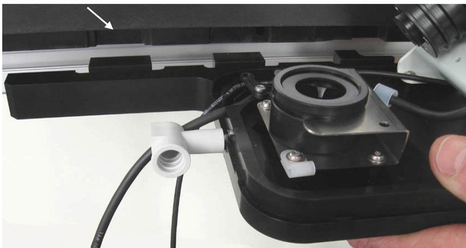
*Fig. 8: Installing the flow cell carrier*
