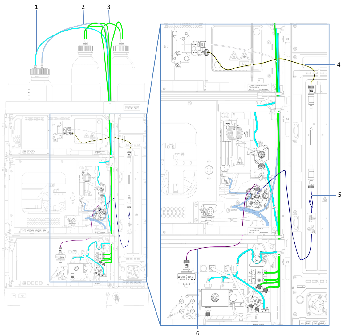
Figure 24: Solvent and wash flow connections in the Vanquish Access system
