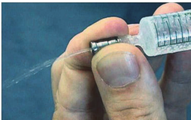
Figure 41. Cleaning the check valve
