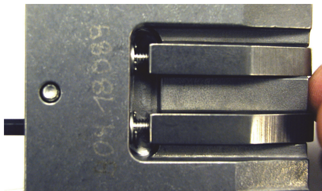
Figure 62. View of piston guide bushings and backing rings held snugly by holding hooks
