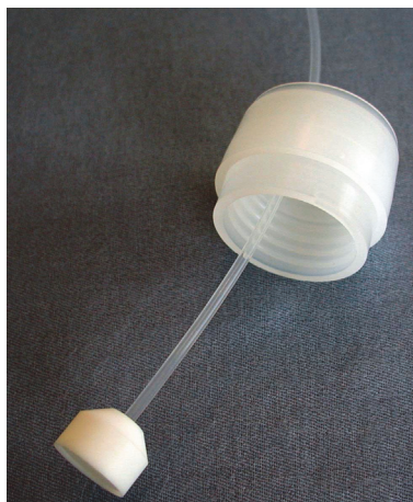
Figure 13. Solvent reservoir cap assembly
