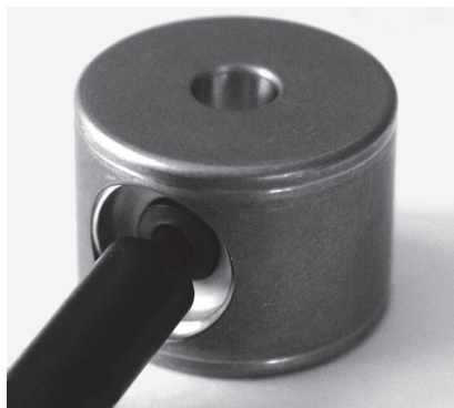
Figure 43. Removing the used primary piston seal
