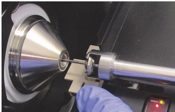
5. Clean the ion transfer tube as described in the MS hardware manual.
