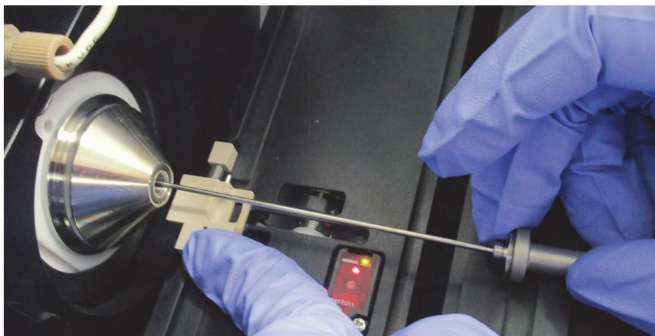
Once you push the tube past the vent ball, the vacuum draws the tube into the spray cone.
