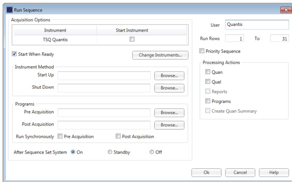
4. If the Start Instrument check box is selected, click **Change Instruments**. Then, in the Change Instruments in Use dialog box, clear the Start Instrument check box and click **OK**.
