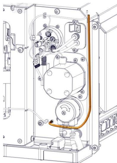
*Figure 99: Routing the needle wash inlet line*
