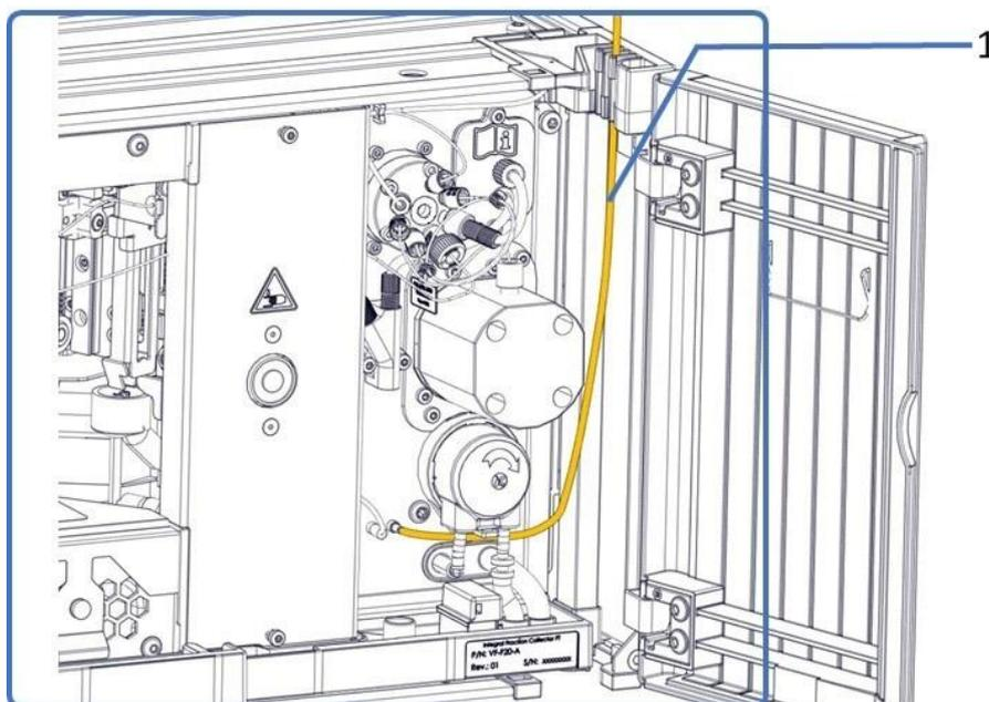
*Figure 30: Needle wash line connection*
