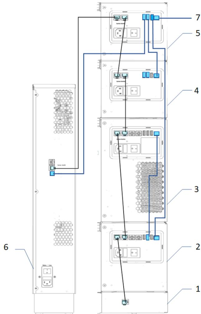
Figure 22: USB and system interlink cable connections
