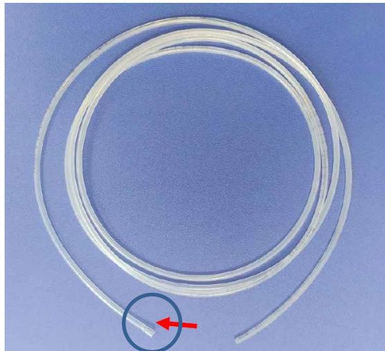
*Figure 98: Needle wash inlet line from reservoir to wash pump, the arrow shows the pre-widened end to be applied to the wash pump inlet*
