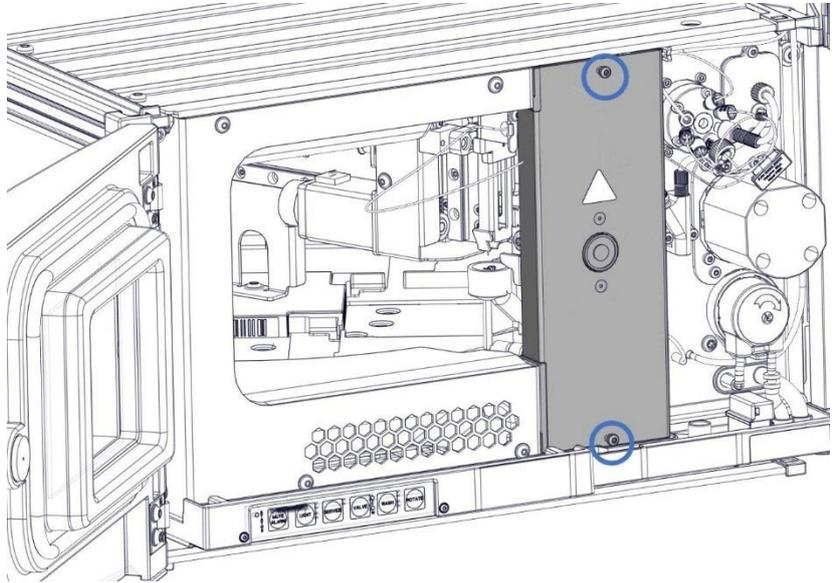
*Figure 70: Tightening two screws and secure the front plate*
