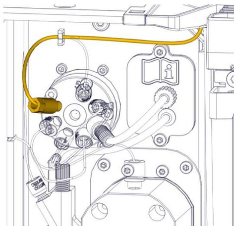
Figure 78: Install the replacement flush solvent tubing
