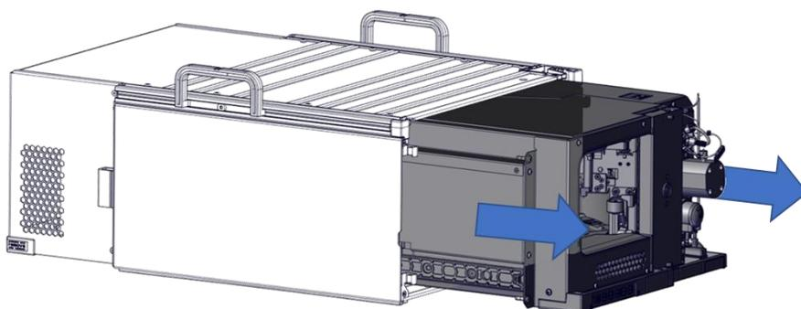
Figure 94: Pulling out the slide-in module
