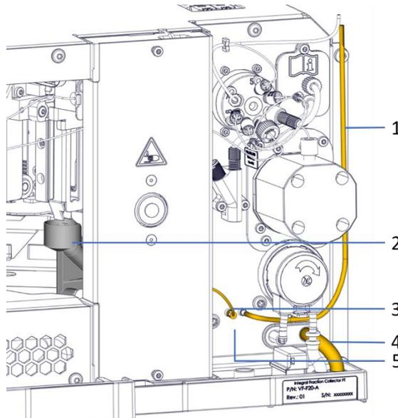
Figure 29: Needle wash components in the device
