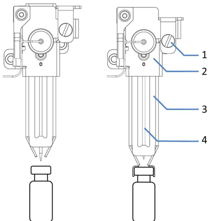
Figure 57: left - **AboveVial** pusher position, right - **InVial** pusher position
