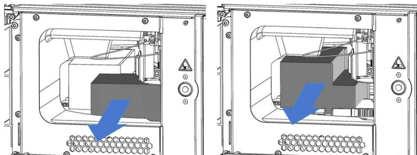
*Figure 16: Remove two carousel protection foams*
