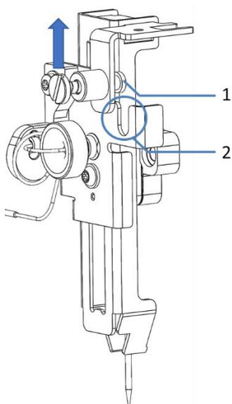
Figure 58: Moving the pusher up by hand
