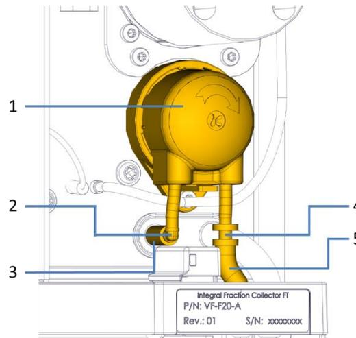
Figure 89: Configuration of drain pump head with tubing (waste tubing)
