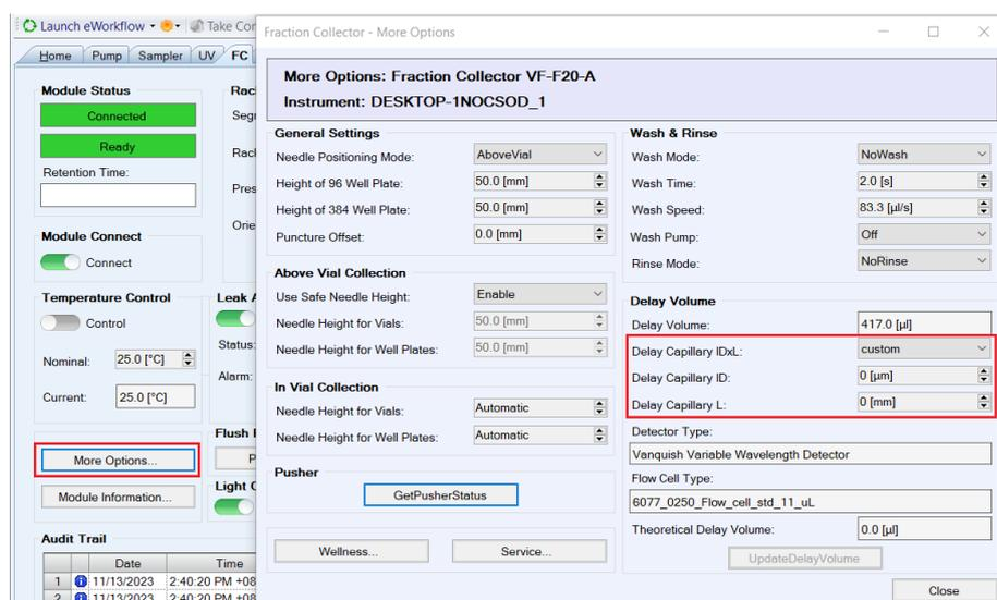
Figure 52: Delay volume capillary drop down menu
