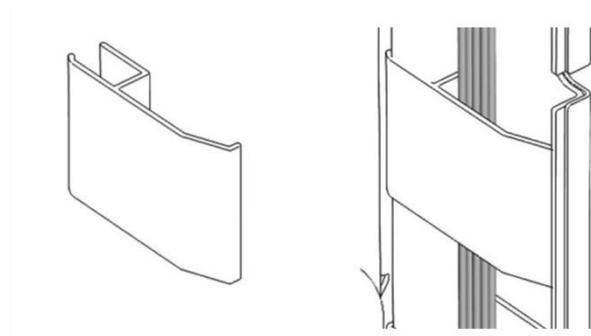
Figure 24: Tubing bracket (left), tubing bracket installed (right)
