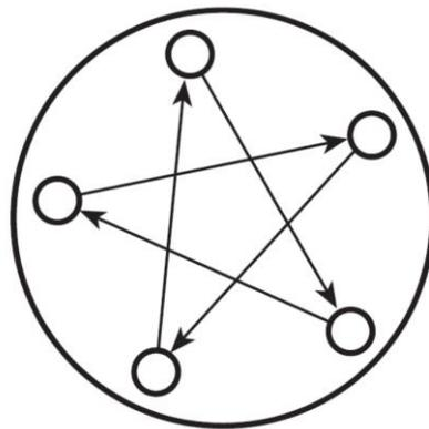
Figure 90: Loosening and tightening order
