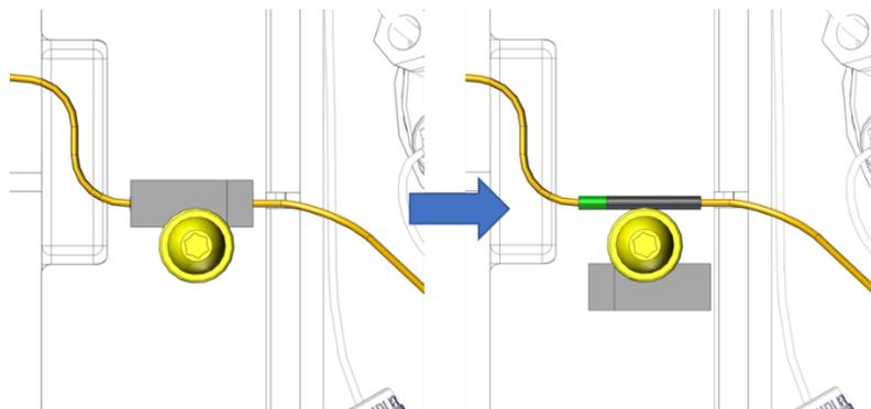
*Figure 80: Loosening the attachment screw to release needle capillary*
