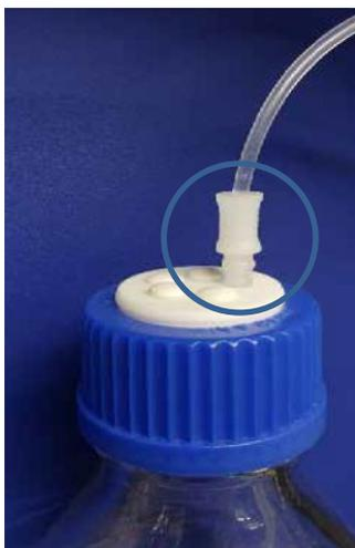
*Figure 100: Needle wash inlet line and retention guide at the reservoir*
