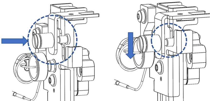
Figure 59: Engaging the lock tab with U-shape slot
