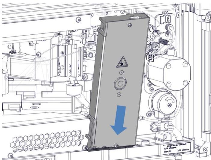
*Figure 69: Putting front plate into place by slightly pushing downward to the bottom*
