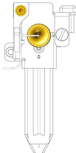
Figure 81: Removing the needle capillary
