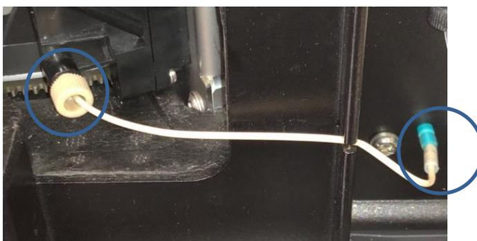
Figure 97: Needle wash outlet line from wash pump to wash port
