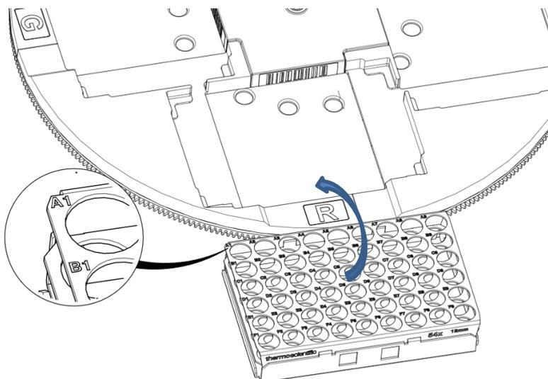
Figure 44: Correct orientation in the carousel (here with a sample rack)
