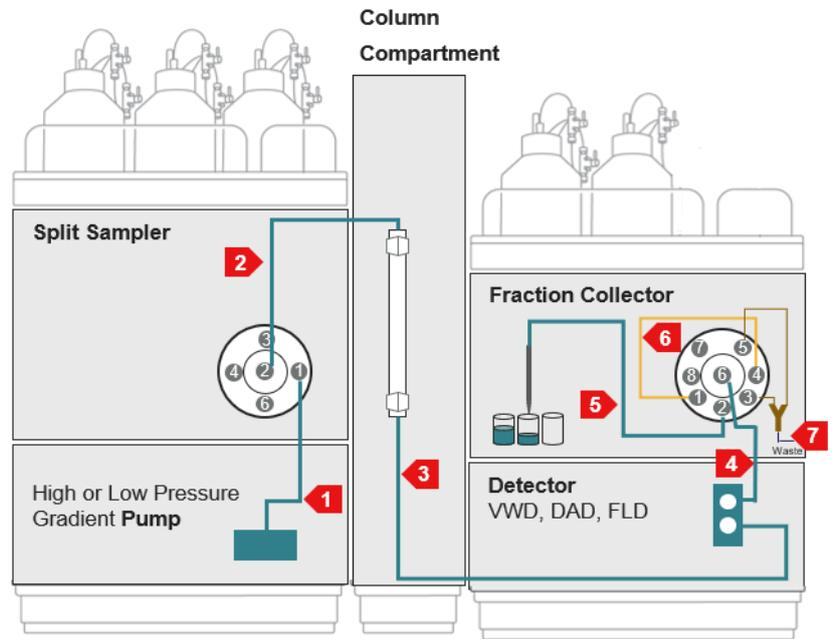
Figure 26: Flow path connection in a two stacks configuration
