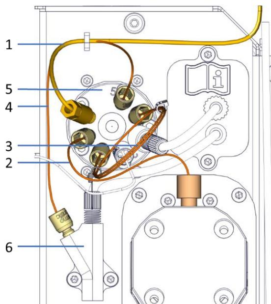
Figure 72: Configuration of flush purge lines
