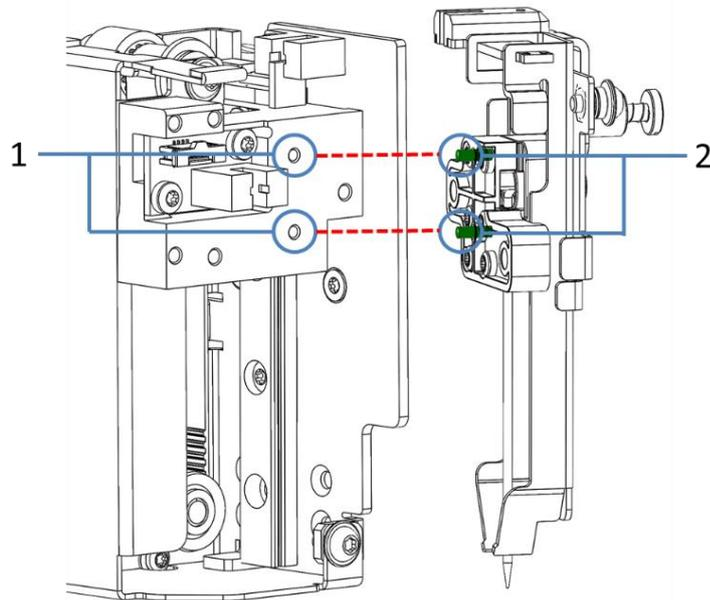
Figure 87: Install the needle unit via two aligning pins
