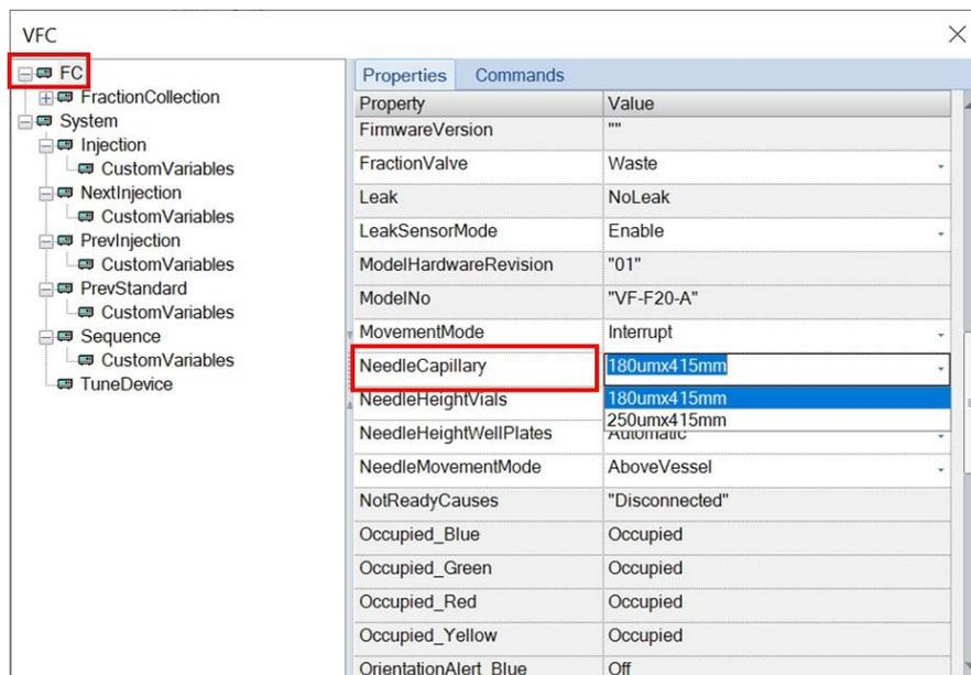
Figure 41: Set the type of needle capillary.
