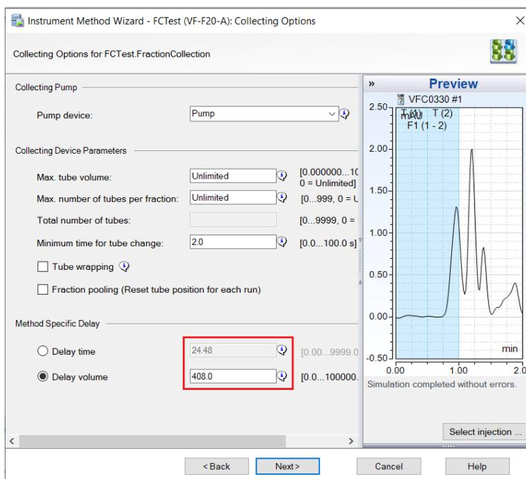
Figure 51: Method specific delay volume and time
