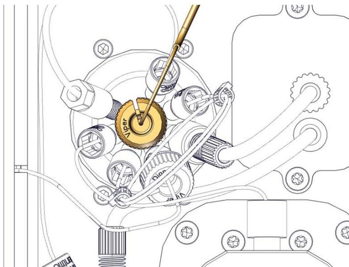
Figure 39: Connecting delay capillary to central port of fraction collection valve
