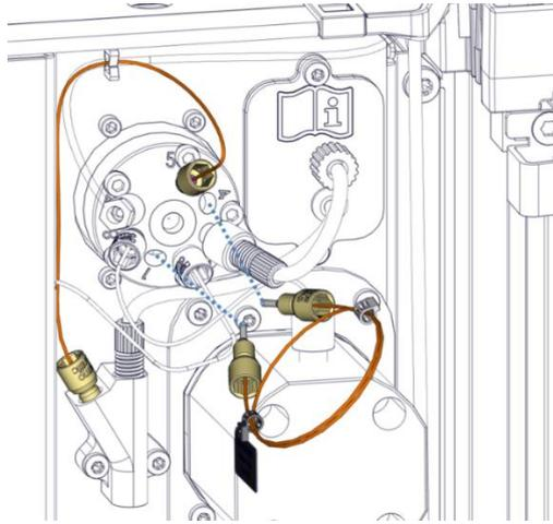
*Figure 76: Installation of flush buffer loop and flush waste tubing*
