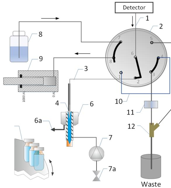
Figure 7: Draw of fresh flush solvent from solvent container to fill flush pump
