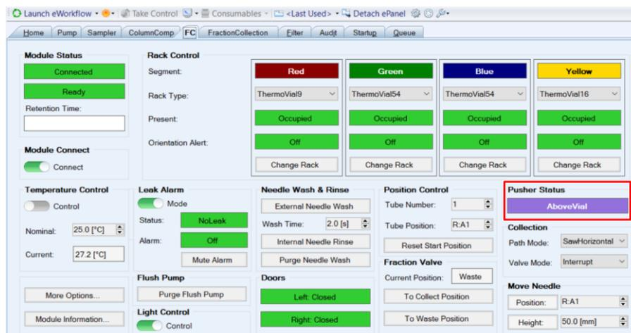
Figure 64: Vial Pusher Position on ePanel (AboveVial)
