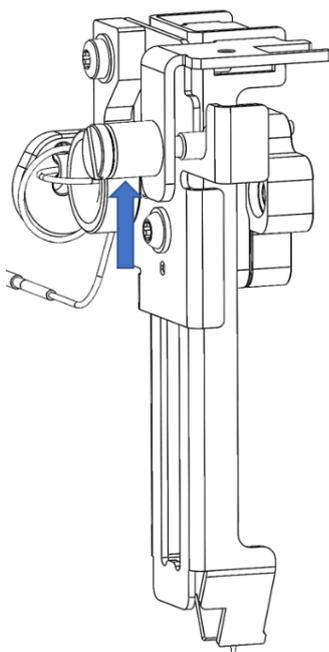
Figure 61: Moving the lock pin up by hand
