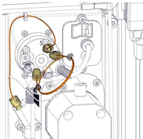
Figure 75: Remove flush buffer loop and flush waste tubing
