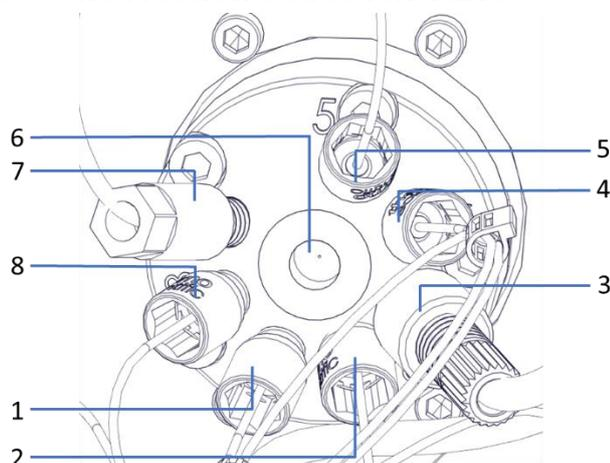
Figure 33: Fraction collection valve with connected capillaries except port 6
