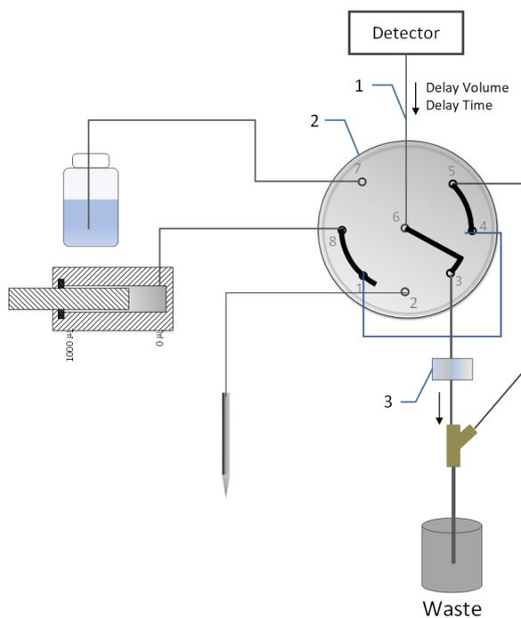
Figure 49: Fraction collection valve located at waste position when running delay volume determination
