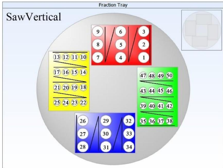
Figure 46: Collection path mode = saw vertical
