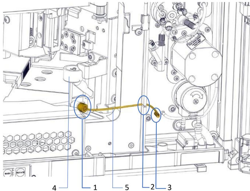
Figure 71: Needle wash outlet line
