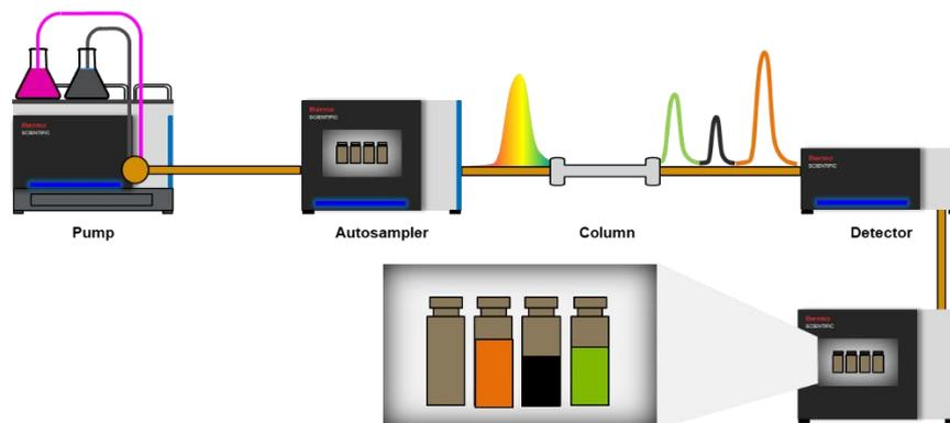
Figure 1: Operating principle of a purification LC system
