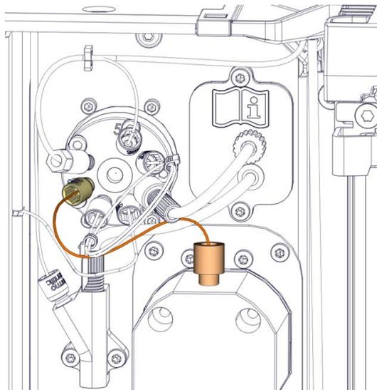
*Figure 77: Flush purge line connected to fraction collection valve and flush pump*
