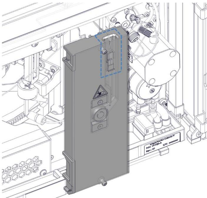
*Figure 68: Connecting the cable connector and putting into the foam top slot*
