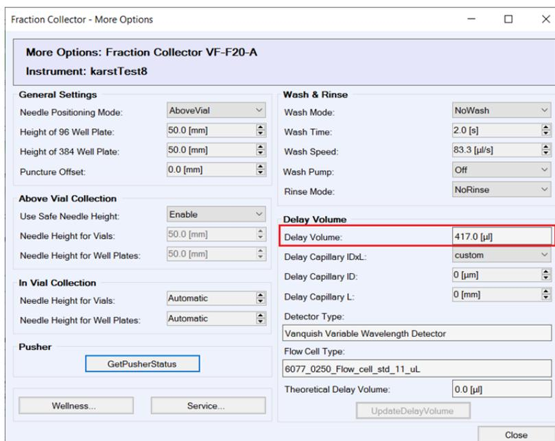
Figure 50: Checking the measured delay volume in the FC ePanel tab
