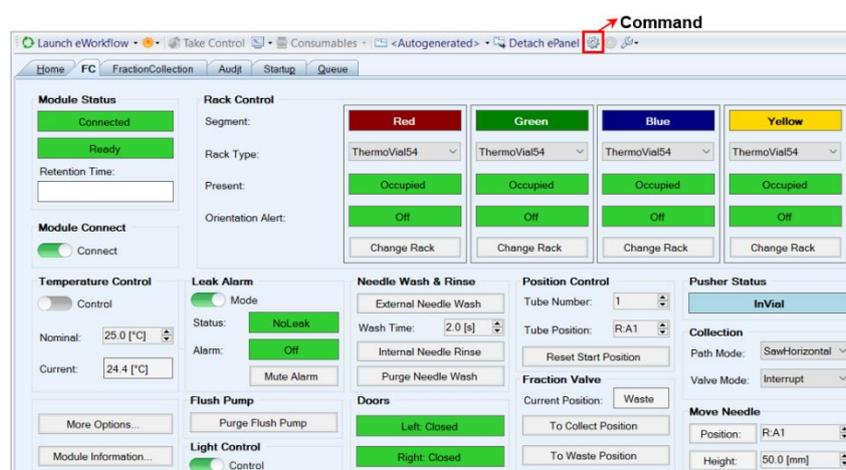
Figure 40: Selecting the Command configuration page
