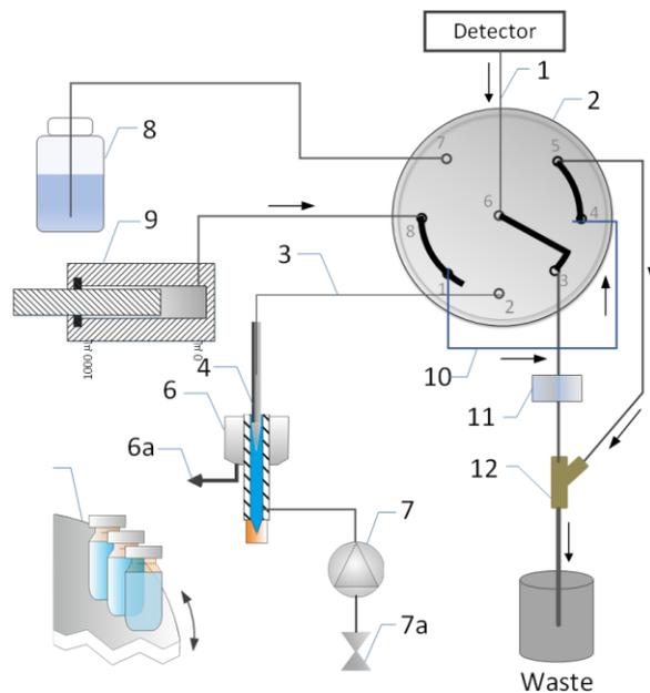
Figure 8: Dispense liquid out to flush buffer loop and drain to waste
