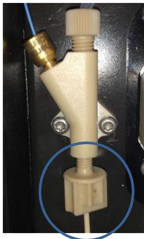
*Figure 101: Assembled waste line at the outlet of Y-connector*
