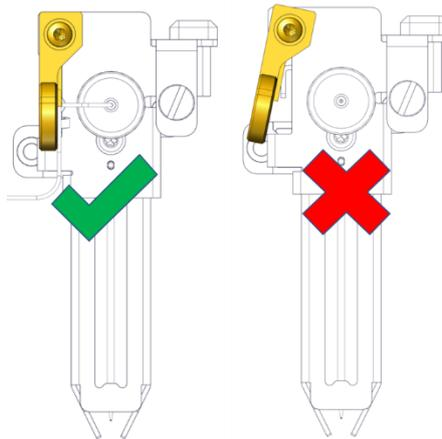
Figure 84: left – correct alignment, right: wrong alignment
