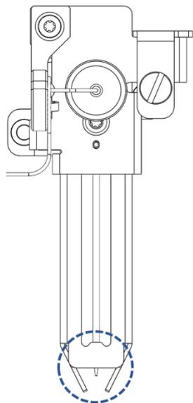
Figure 62: Checking the needle tip higher than the pusher tip
