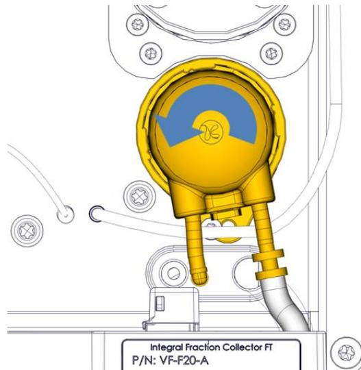
Figure 90: Drain pump rotate counterclockwise to release the pump head from pump motor
