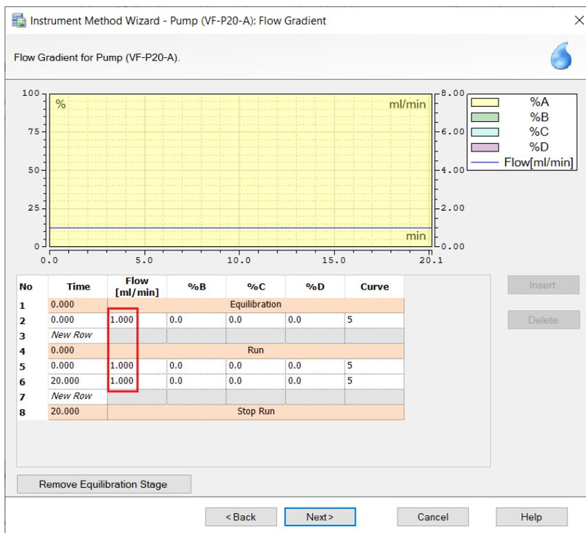
Figure 55: Pump Flow Rate on Flow Gradient page in instrument method
