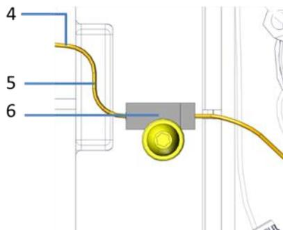
Figure 85: Route and secure the needle capillary on the front surface of the device
