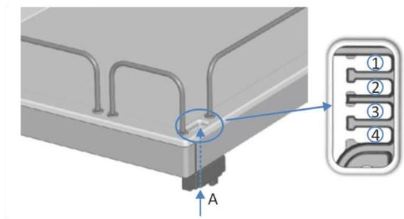
Figure 31: Guide hole and tubing guides in the solvent rack
