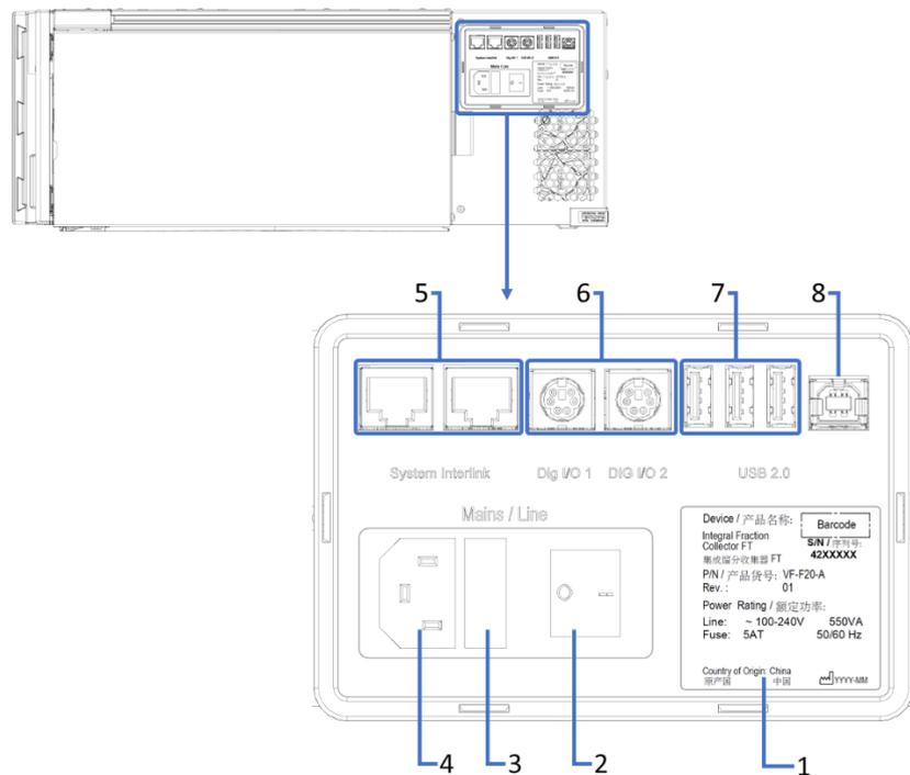
Figure 21: Electrical connectors on the right side of the device
