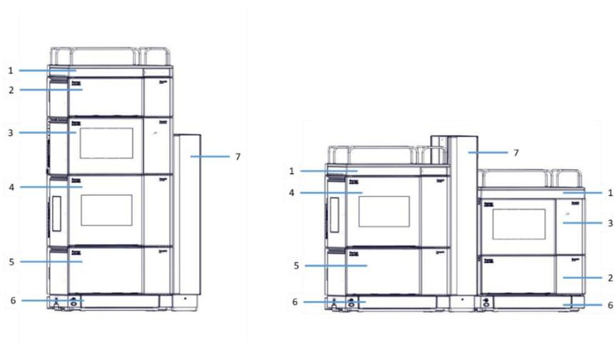
Figure 20: Vanquish system, standard configuration (examples): left - one stack, right - two stacks
