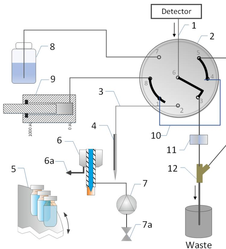
Figure 2: Fluidic configuration of the fraction collector in idle state (fraction collection valve in waste position)
