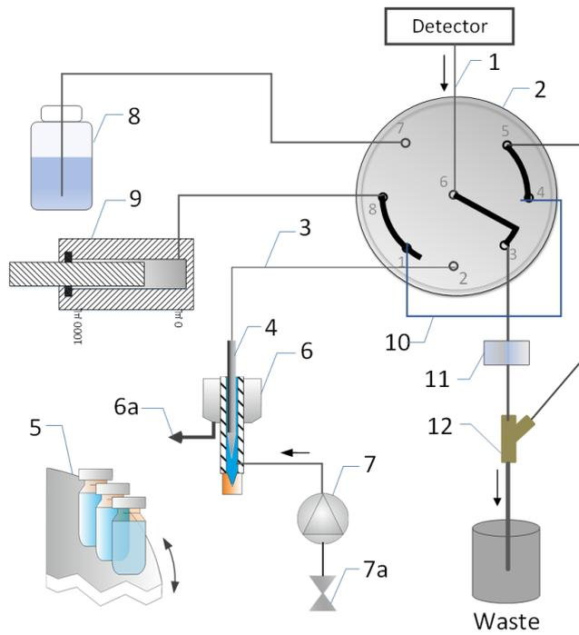
Figure 5: External Needle Wash in needle wash port with fraction collection valve in waste position
