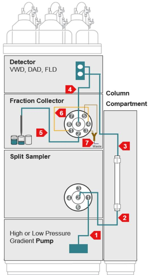
Figure 25: Flow path connection in a one stack configuration
