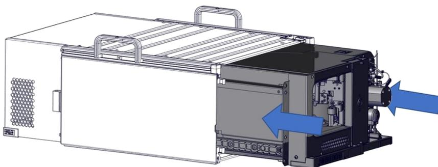
*Figure 95: Inserting the slide-in module*
