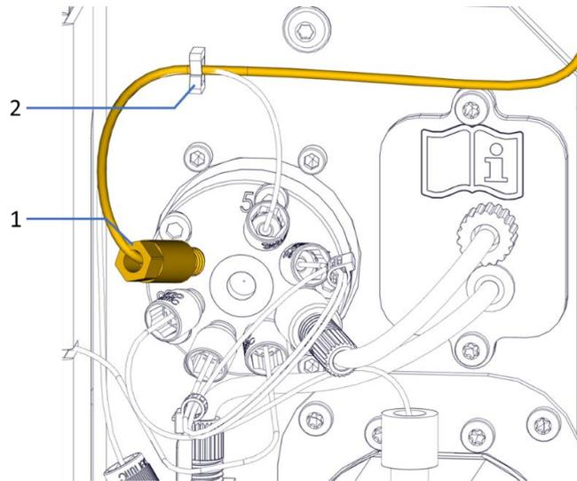
Figure 35: Holder for the flush solvent tubing
