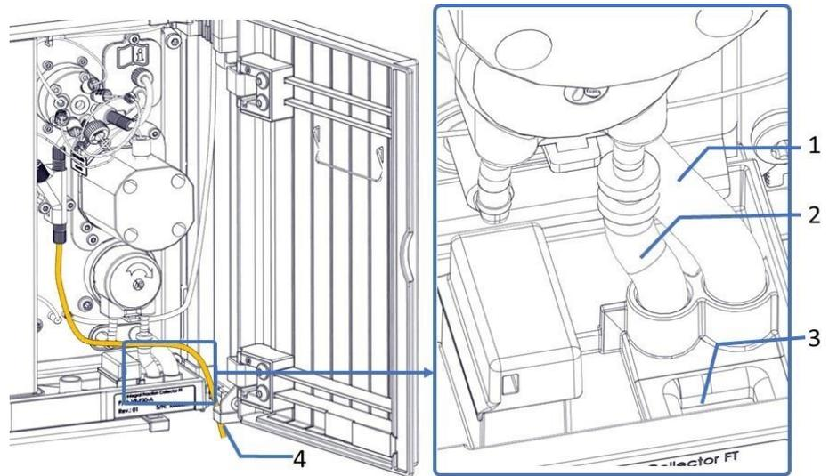
Figure 28: Drain ports in the leak tray and waste line from Y-connector to waste container
