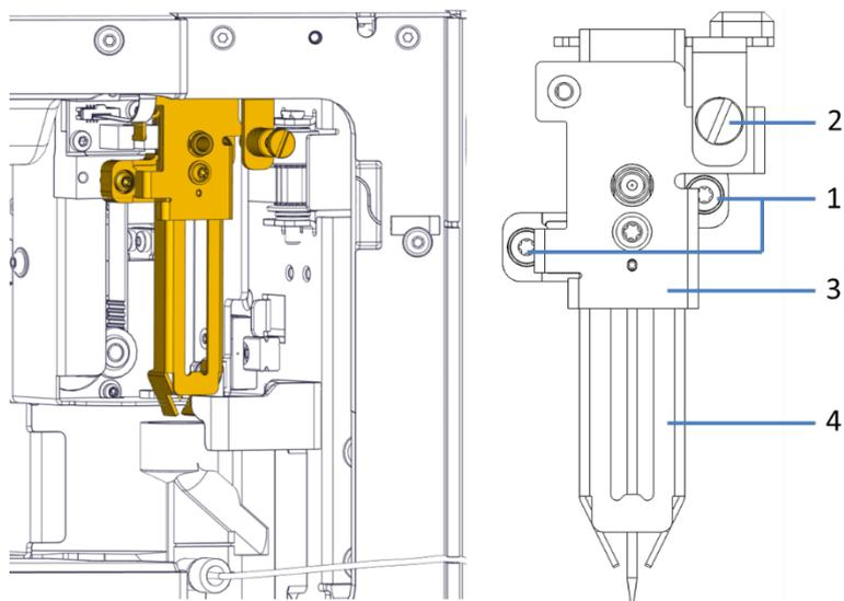
Figure 86: Removing the needle unit
