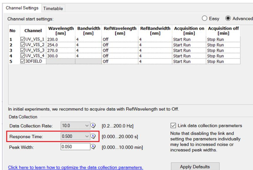
Figure 56: Detector Response Time in Channel Settings in Instrument Method
