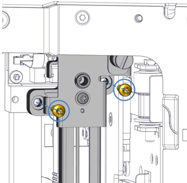
Figure 88: Tighten the needle unit with two attachment screws
