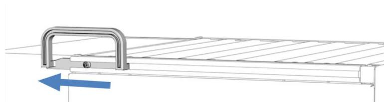
Figure 15: Sliding off the carrying handle from the left rail
