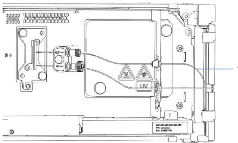
Figure 38: Removing the detector waste line
