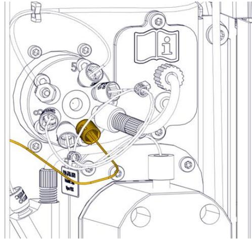
Figure 83: Connect Viper fitting to fraction collection valve port 2
