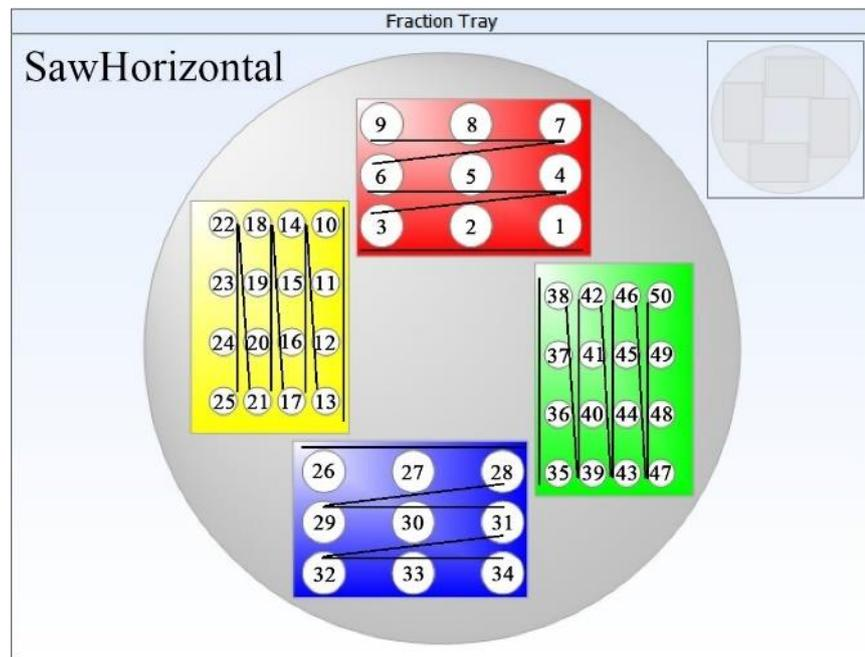
Figure 48: Collection path mode = saw horizontal
