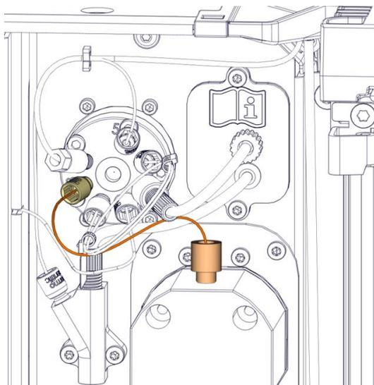
Figure 74: Flush pump to fraction collection valve capillary
