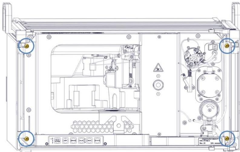
Figure 93: Captive screws on the slide-in module
