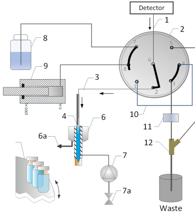
Figure 6: Internal Needle Rinse in needle wash port with fraction collection valve in collect position
