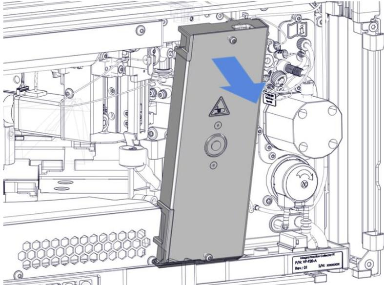
Figure 66: Pulling out the front plate
