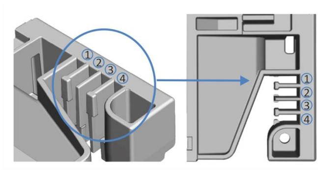
Figure 23: Tubing chase with tubing guides (left: view from inside, right: view from top)
