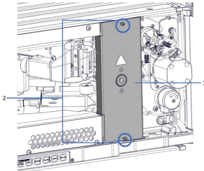
Figure 65: Loosening the two screws in front plate
