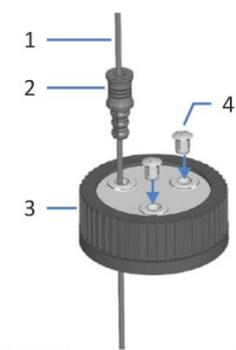
Figure 32: Securing the needle wash line with the reservoir cap
