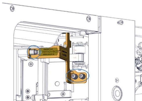
*Figure 17: Remove needle arm shipping lock*
