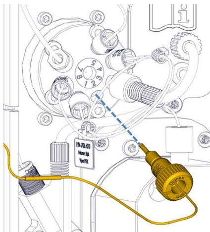
Figure 82: Disconnect Viper Fitting
