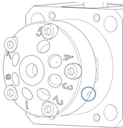
Figure 88: Drain hole on the right side of fraction collection valve
