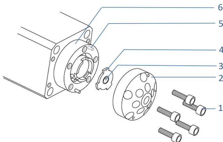
Figure 89: Exploded view of the fraction collection valve
