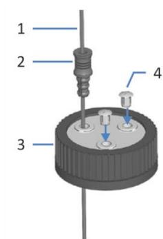
Figure 37: Securing the flush solvent tubing with the reservoir cap
