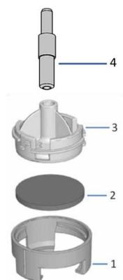
Figure 34: Assembling the filter holder and solvent line adapter
