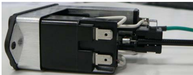
Figure 160. Metal tip of Bowden cable attached to the AC input power module
