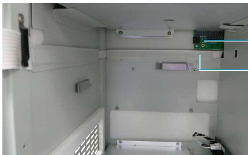
Figure 188. Bracket holding the front panel LED cable onto the autosampler's back wall
