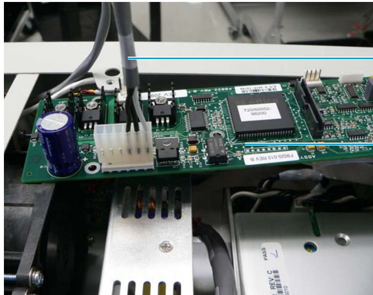
Figure 129. Connecting the oven Peltier cable to the temperature control PCB
