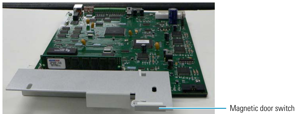
Figure 193. Magnetic door switch
