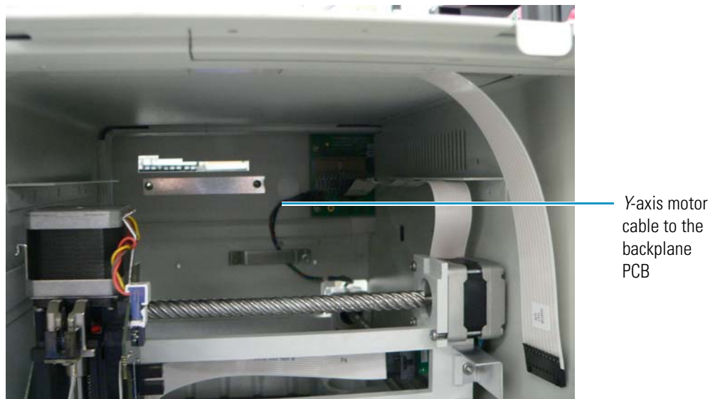
Figure 111. Y-axis motor cable to the backplane PCB
