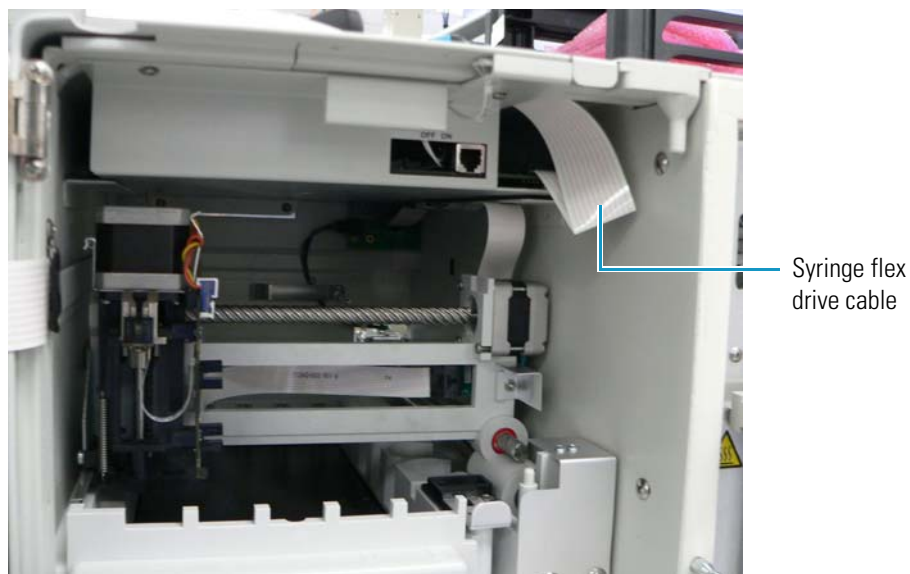
Figure 190. Connection of the syringe flex drive cable to the CPU PCB
