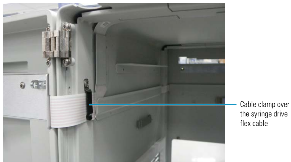
Figure 148. Cable clamp installed over the syringe drive flex cable
