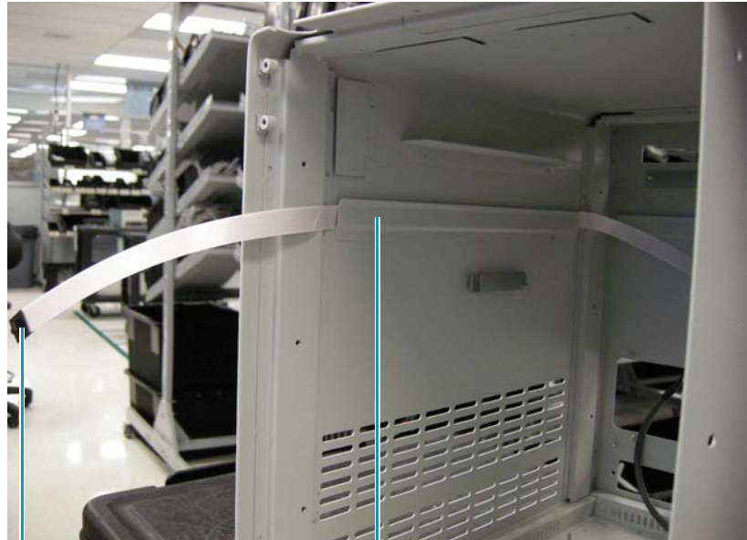
Figure 187. Bracket holding the front panel LED cable onto the autosampler's side wall
