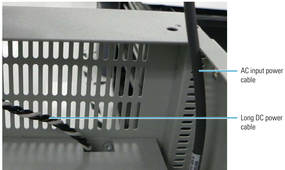
Figure 170. Positioning the AC input power cable
