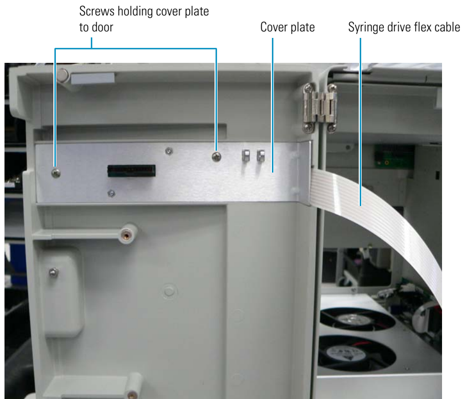
Figure 184. Cover plate on inside of front left door
