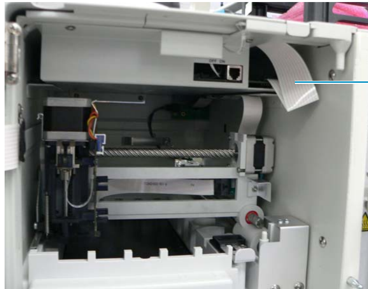
Figure 149. Connection of the syringe flex drive cable to the CPU PCB
