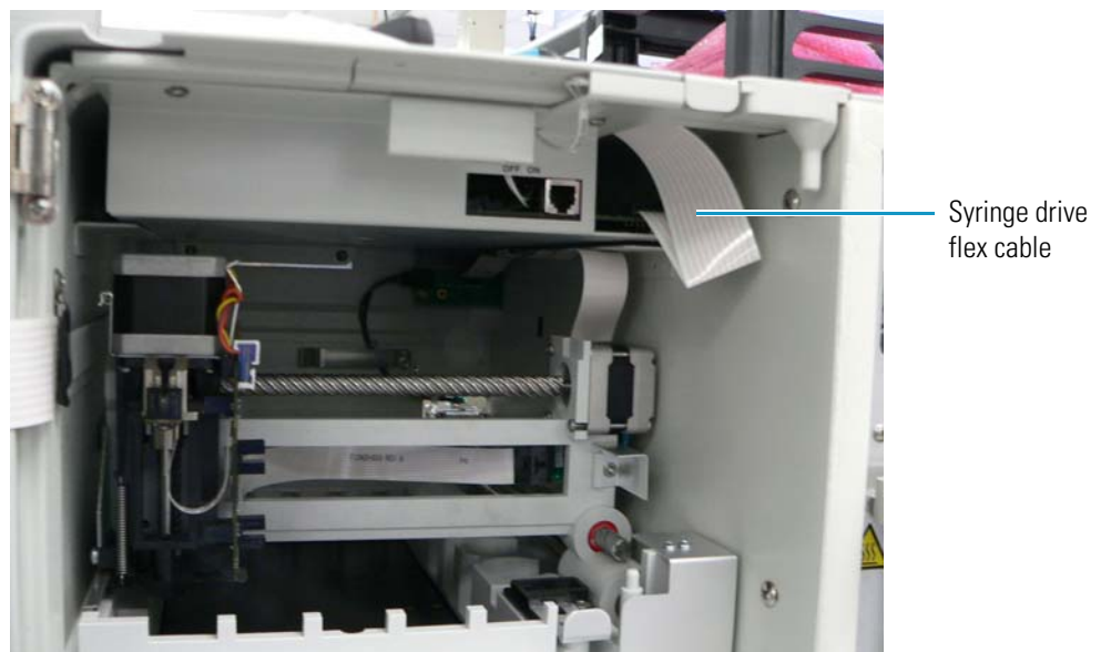
Figure 94. Syringe drive flex cable connected to the CPU PCB
