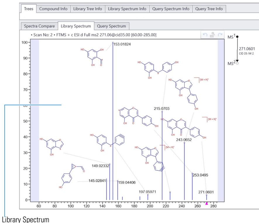
The application annotates the spectral peaks with fragment structures (Figure 15).
