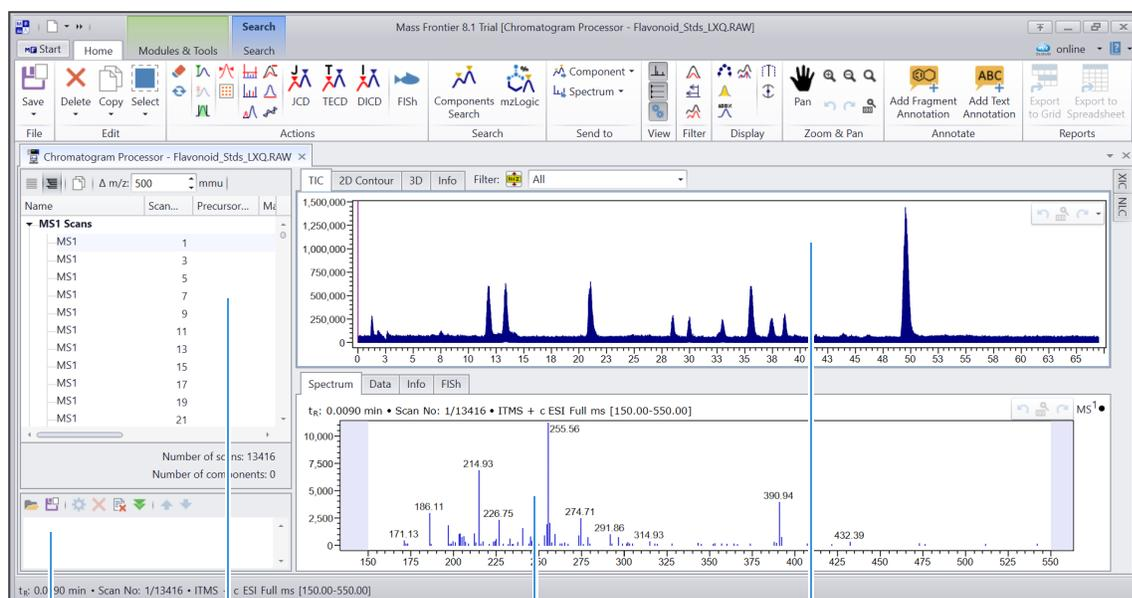
Command processor view      Chromatogram data view      Spectrum page of the MS spectrum view      TIC page of the chromatogram view
