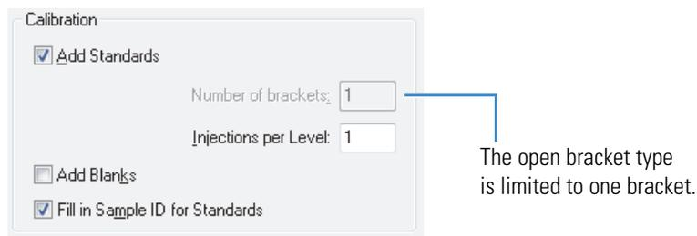
**Figure 45.** Calibration area for the None bracket type
