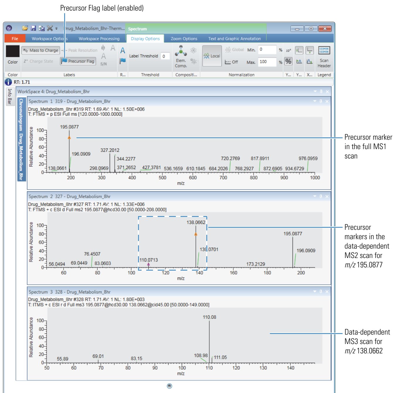
Figure 68. MS1 and MS2 level scans with precursor markers for the data-dependent MS2 level and MS3 level scans
