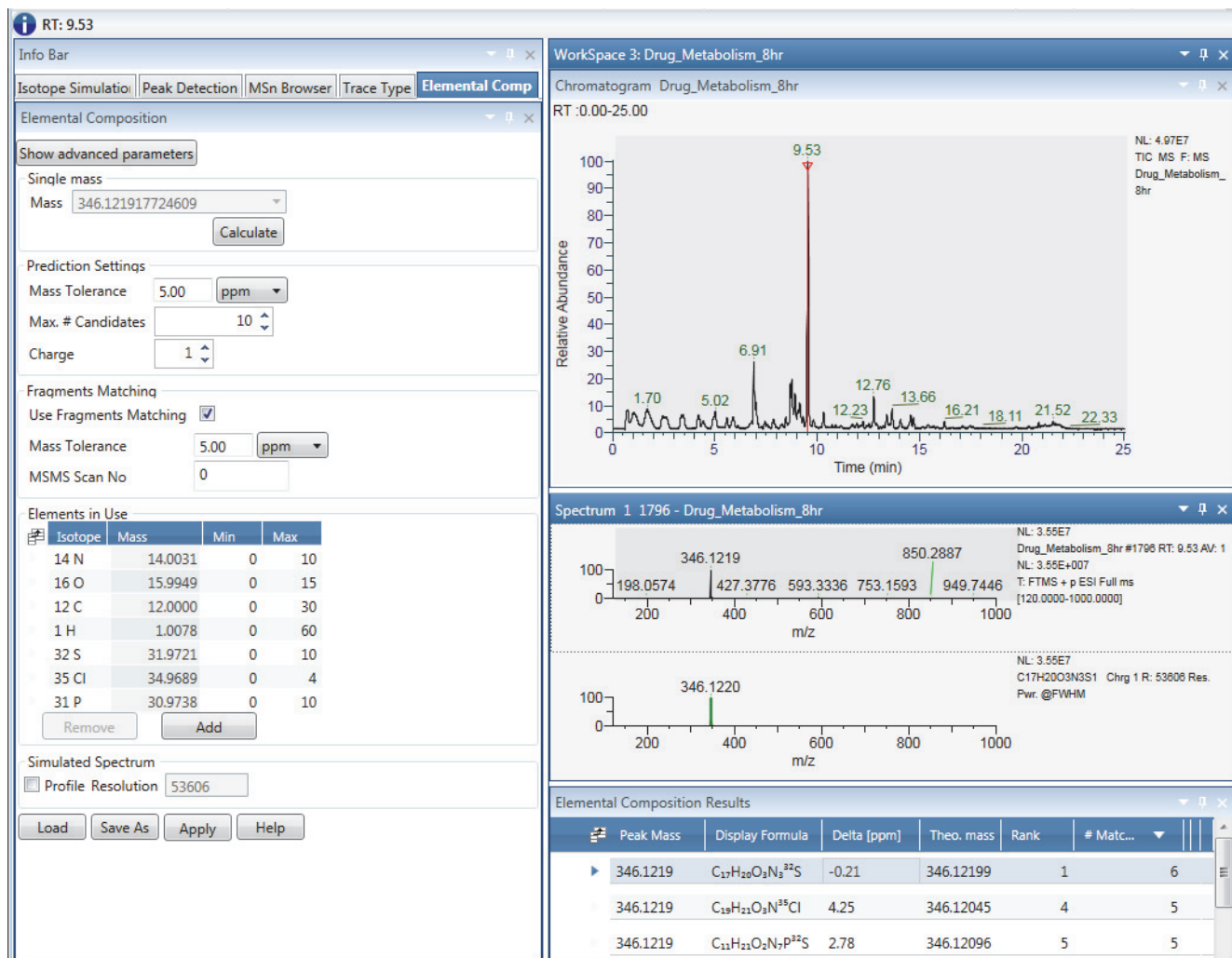
Figure 87. Elemental Composition page and Spectrum view with a theoretical spectrum
