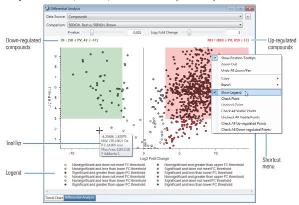
Figure 8. Differential analysis for the compounds extracted from red o-rings or brown o-rings with 50% ethanol/water
