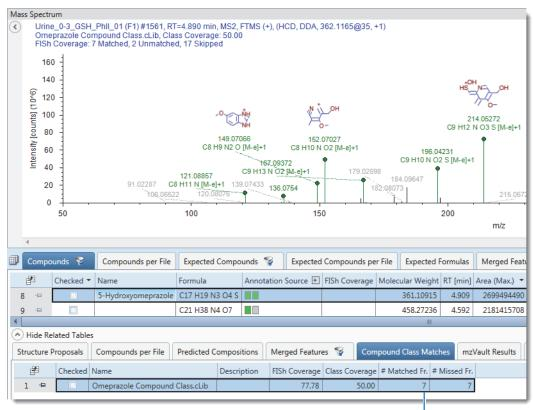
Figure 122. Fragmentation scan and compound class match result for a detected compound
