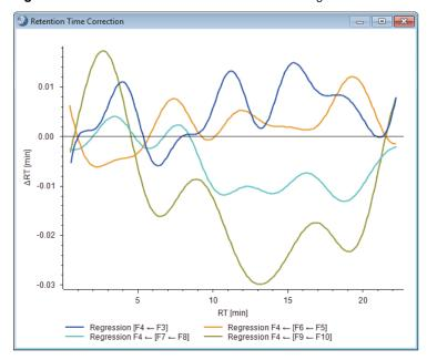
Figure 114. Retention Time Correction view with regression curves for multiple input files
