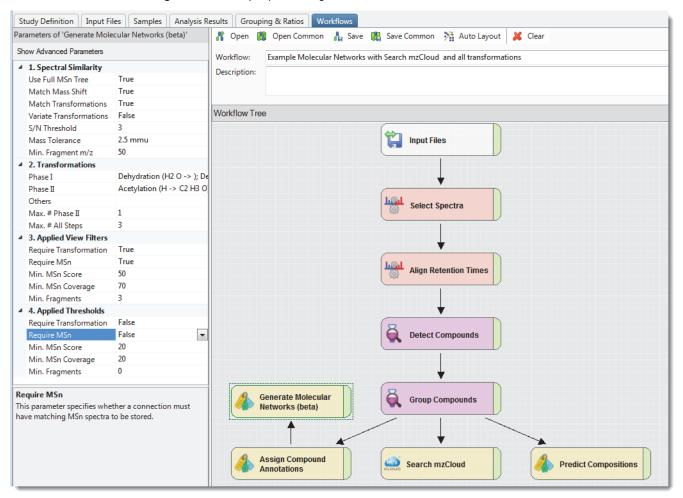
The input to the Generate Molecular Networks node is a list of annotated compounds, and the output from the node is a table of similar compounds for each detected compound.
