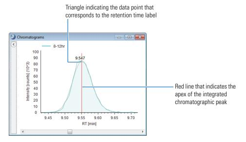
Figure 120. Expected compound trace for a single input file
