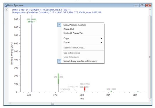
**Figure 88.** MS1 scan with color-coded mass spectrum peaks and the shortcut menu
