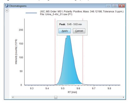
Figure 86. Manually integrated chromatographic peak
