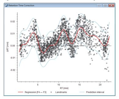
Figure 113. Retention Time Correction view with the regression curve for one input file
