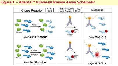
The Adapta<sup>TM</sup> assay is composed of two steps. First, a standard kinase reaction is performed in the presence or absence of inhibitor. In the second step, formation of ADP is detected by adding a europium-labeled anti-ADP antibody, Alexa Fluor® 647 labeled ADP, and EDTA. ADP formed by uninhibited kinase disrupts antibody-tracer interaction, resulting in a low TR-FRET signal. Inhibited kinase forms less ADP, resulting in an intact antibody-tracer interaction and a high TR-FRET signal.
